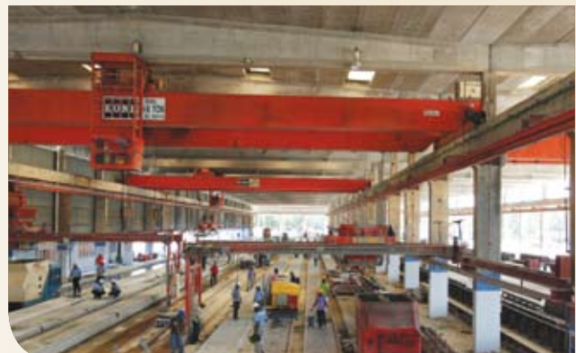
PROPERTY, ENGINEERING & CONSTRUCTION SECTOR: KUB Precast's manufacturing factory for IBS components in Senawang, Negeri Sembilan
