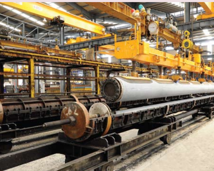
Pile being lifted with a vacuum lift during demoulding process
