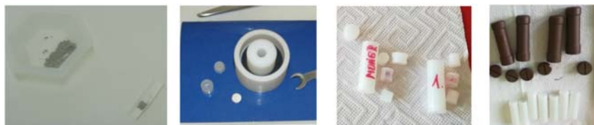
Figure 21.15 Only a few milligrams of samples are packed in plastic capsules and irradiation containers for short irradiation through a pneumatic rabbit system. (Photos by K. Gmélíng).
