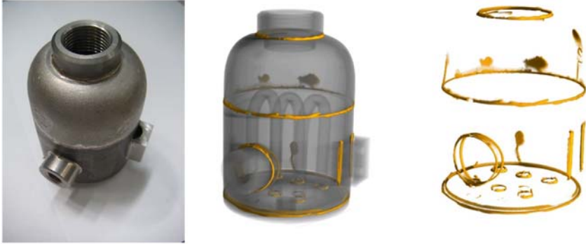
Figure 9.13 Brazing connections inside a stainless steel dummy sample (diameter about 50 mm) demonstrate the high contrast of the boron containing the brazing agent and its distribution after the treatment in the heat [42].
