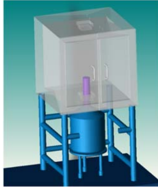
Figure 21.14 A vertical HPGe gamma spectrometer, placed in a low-level counting chamber. The sample-to-detector distance can be adjusted stepwise with a set of plastic spacers (drawing by L. Szentmiklósi).
