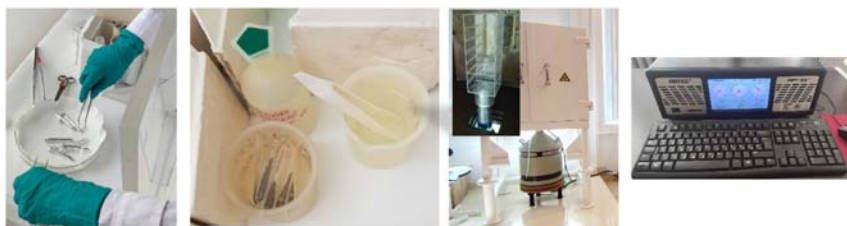
Figure 21.18 After long irradiation, the samples are unwrapped from aluminum foils and etched with mixtures of acids to get rid of potential external surface contamination. Thereafter they are measured at different distances from the HPGe detector at different decay times (Photos by K. Gméling).
