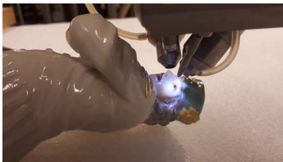
Figure 17.8 Measuring head during analysis of a porcelain figurine by X-ray fluorescence spectroscopy with the use of a micro beam.
