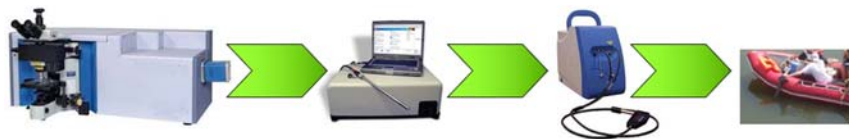
Figure 14.15 Evolution of Raman spectrometers used to identify water quality, from a laboratory instrument to an on-board one.
