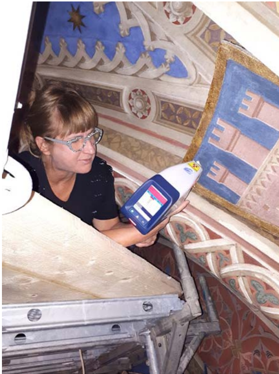
Figure 17.6 Wall paintings analysis by handheld EDXRF instrumentation.
