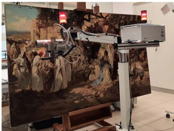
Figure 17.7 Painting's examination with the use of ArtTAX \mu XRF spectrometer.
