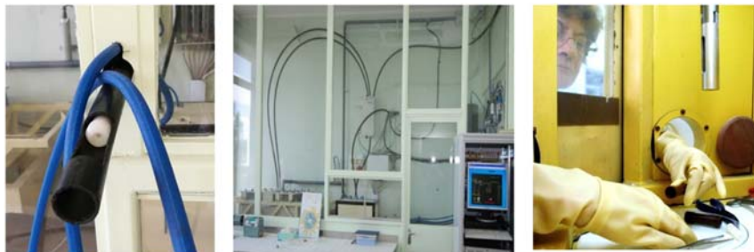
Figure 21.17 For short irradiation, samples are loaded into the irradiation channel through a rabbit system operated with pressured air, and after irradiation, they are repacked into an inactive holder. (Photos by K. Gméling).
