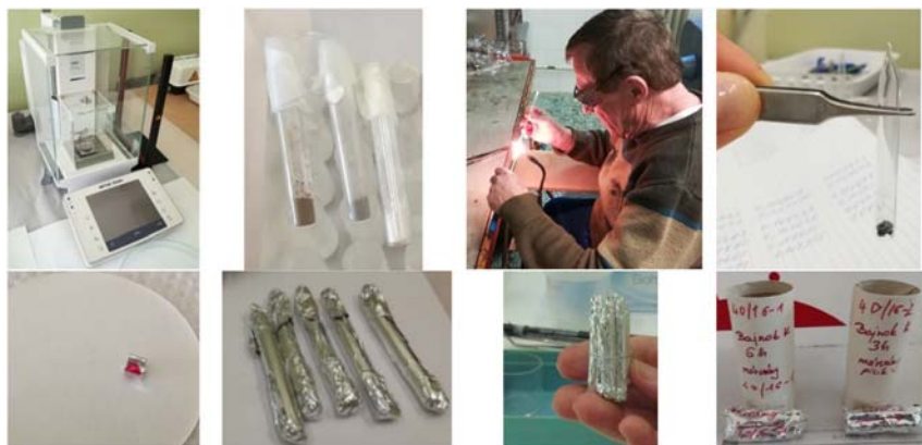
Figure 21.16 Precisely weighed amounts of samples are encapsulated in high-purity quartz ampoules or heat-resistant plastic holders and wrapped in aluminum foil. A set of 6–7 samples can be packed together enabling simultaneous irradiation under identical irradiation conditions in case of long irradiation. (Photos by K. Gmélíng).
