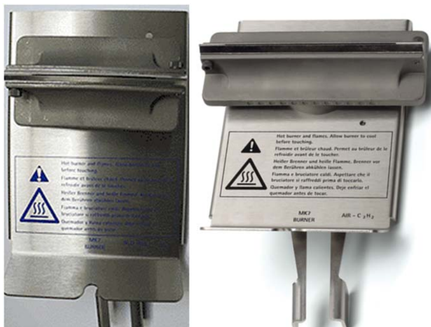
Figure 19.10 AAS burners 50 mm (left) and 100 mm (right). From AAS Burners, < https://www.agilent.com/store/en_US/Prod-210164000/210164000 >, 2021.
