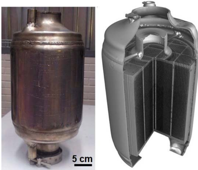
Figure 9.18 Photo ( left ) and neutron tomography results ( right ) of a Diesel particulate filter, where the structure, but also the amount of soot and ash can be determined quantitatively.
