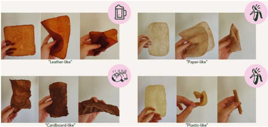
Fig. 12 From upper left to down right: Beer waste with a texture like leather. Banana waste with a texture like vegetable parchment paper. Mix of fruits and vegetables with a texture like rough cardboard or paper. Sample made from banana waste with a texture like plastic material
