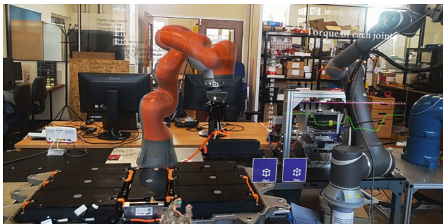
Fig. 8 Demonstrative case: cable removal task
