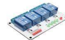
Pump Run Stop Relays
