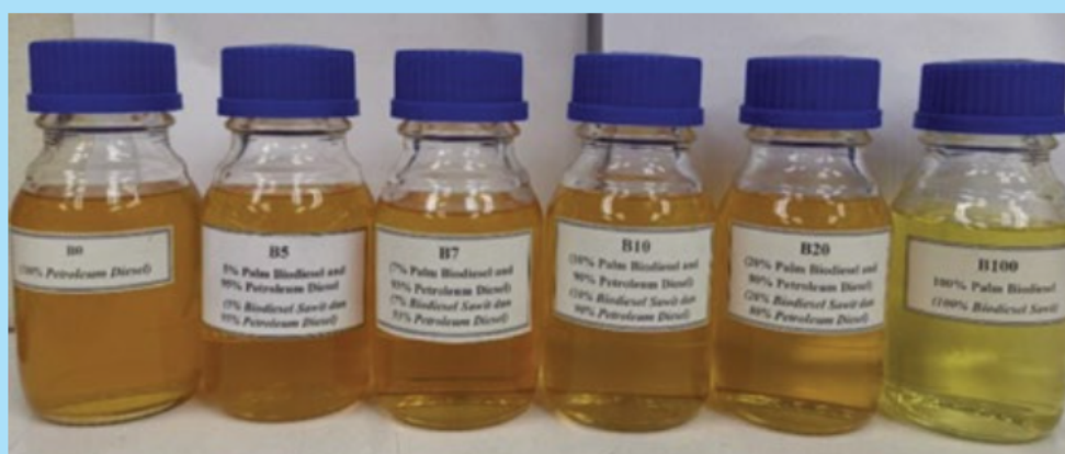
Rajah 2. Diesel petroleum B0, B5, B7, B10, B20 dan biodiesel sawit (B100).
