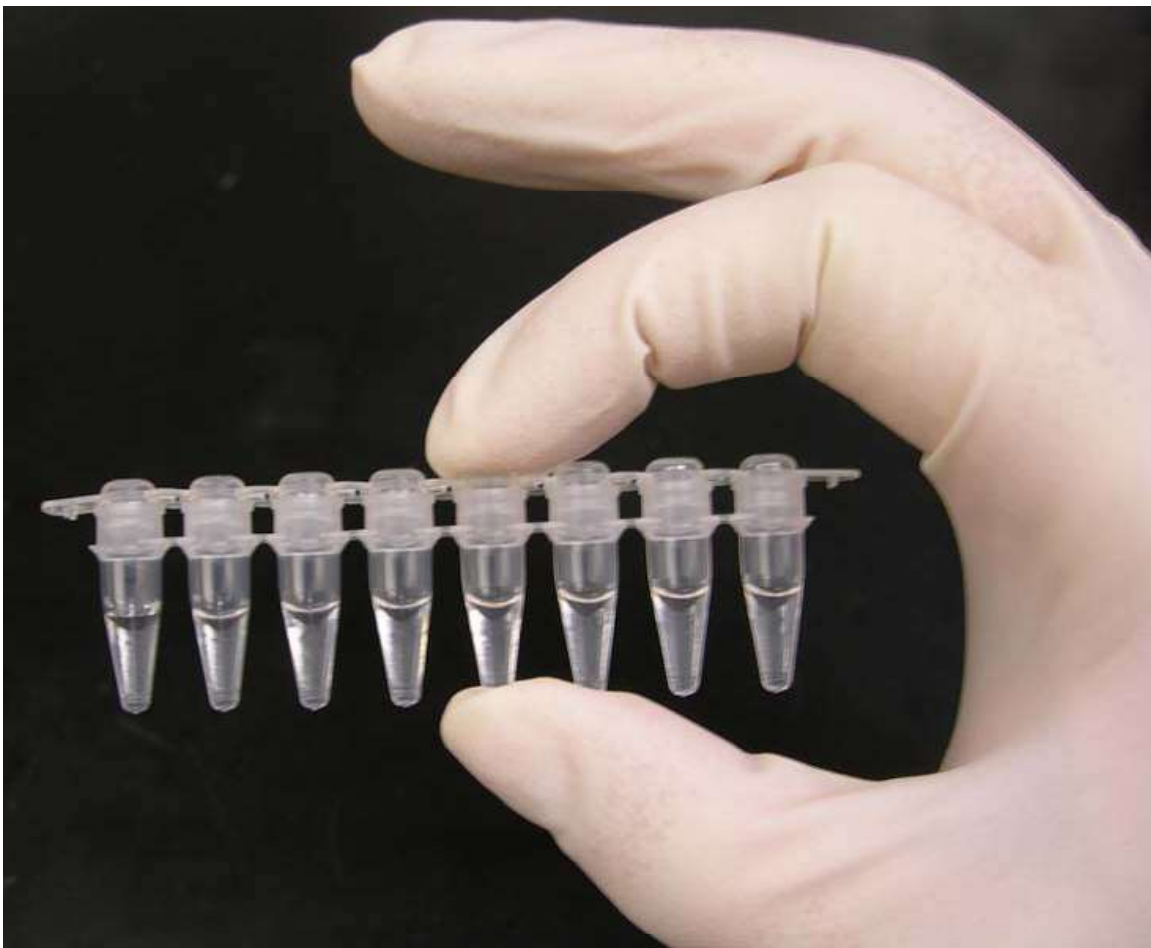
A strip of eight PCR tubes, each containing a 100 \mu l reaction mixture
