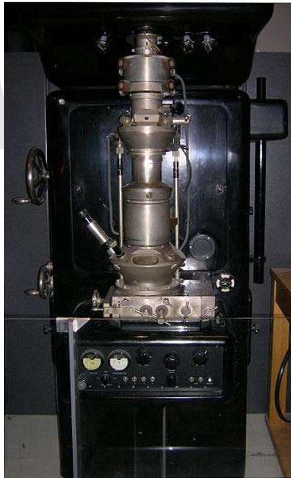
Electron microscope constructed by Ernst Ruska in 1933
