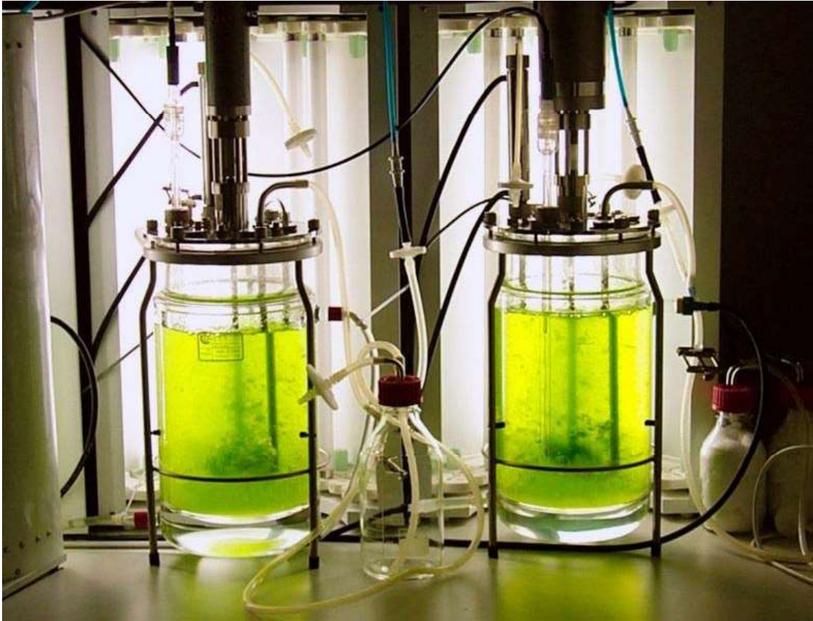
Moss photobioreactor with Physcomitrella patens
