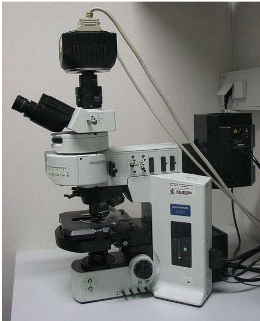
An upright fluorescence microscope (Olympus BX61) with the fluorescent filter cube turret above the objective lenses, coupled with a digital camera.
