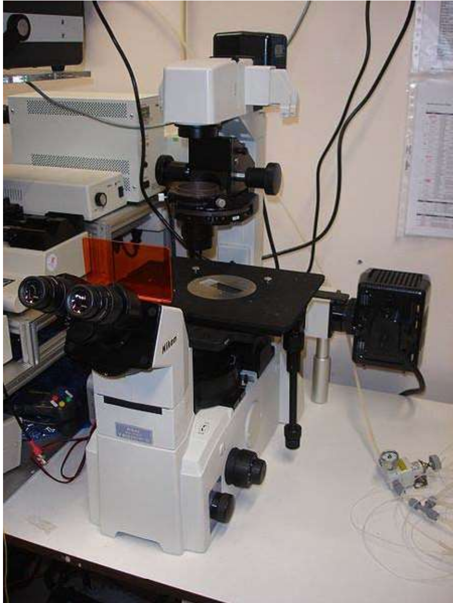
An inverted fluorescence microscope (Nikon TE2000) with the fluorescent filter cube turret below the stage. Note the orange plate that allows the user to look at a sample while protecting their eyes from the UV light.
