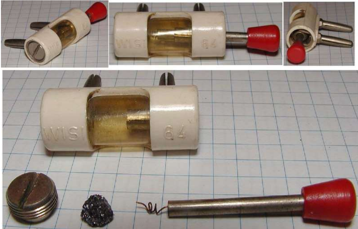
A crystal detector in commercial form from the 1960's
