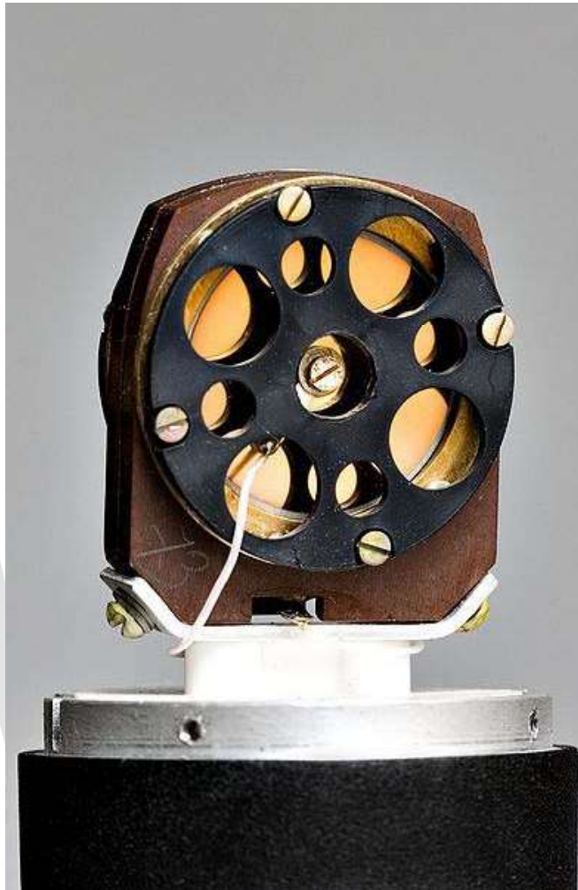
Inside the Oktava 319 condenser microphone
