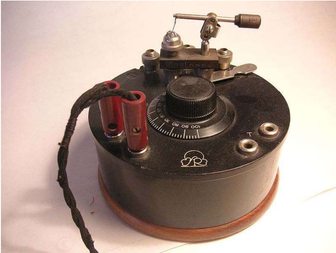
A small portable crystal radio, with a cat's whisker detector visible at top
