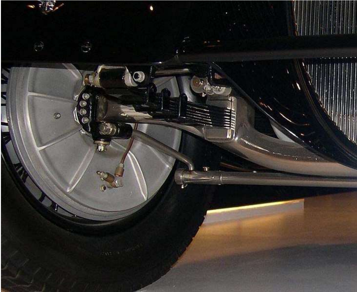
Quarter-elliptical spring in a 1937 Bugatti Type 57SC
