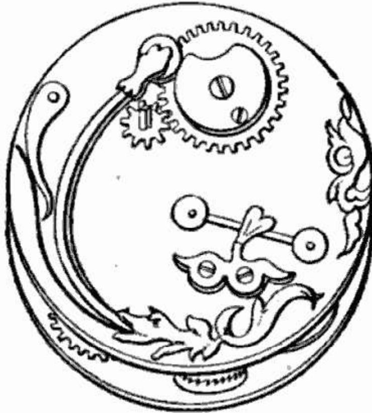
16th century pocketwatch movement with stackfreed (near top).
