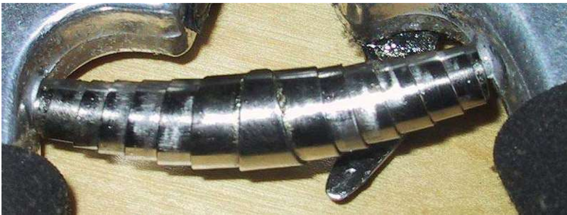
A volute spring. Under compression the coils slide over each other, so affording longer travel.
