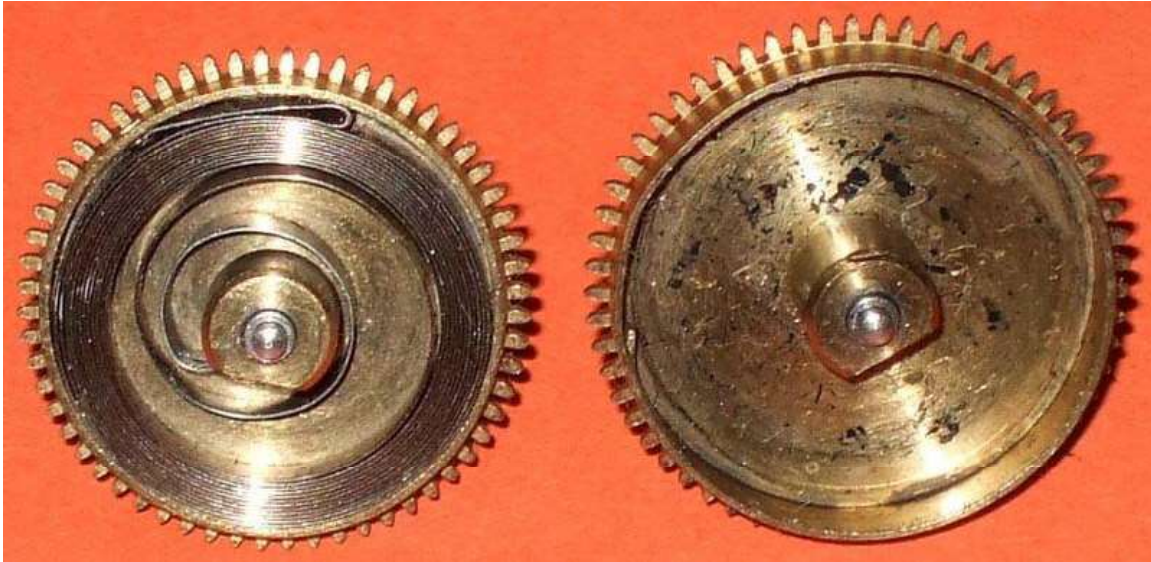
Going barrel of a watch
