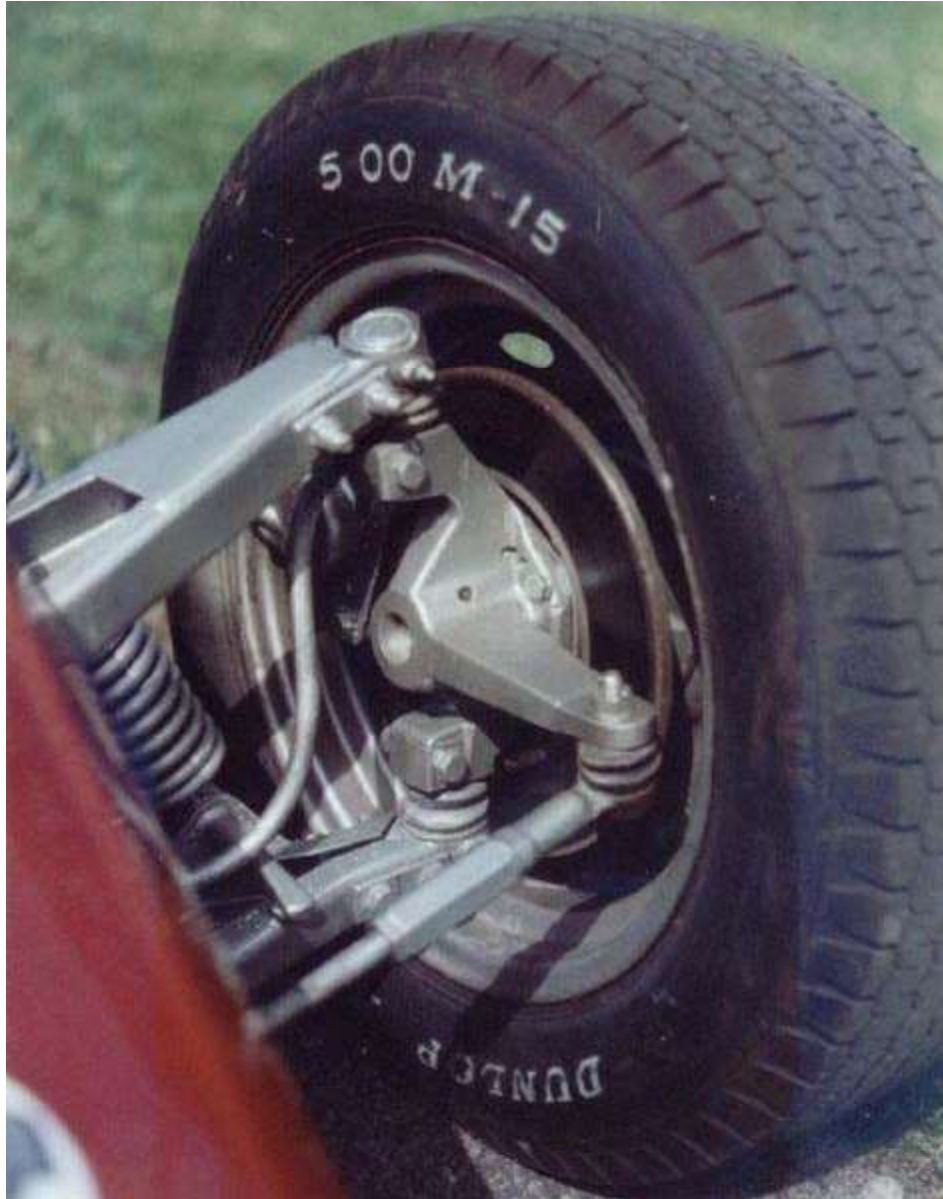
Part of car front suspension and steering mechanism: tie rod, steering arm, king pin axis (using ball joints).
