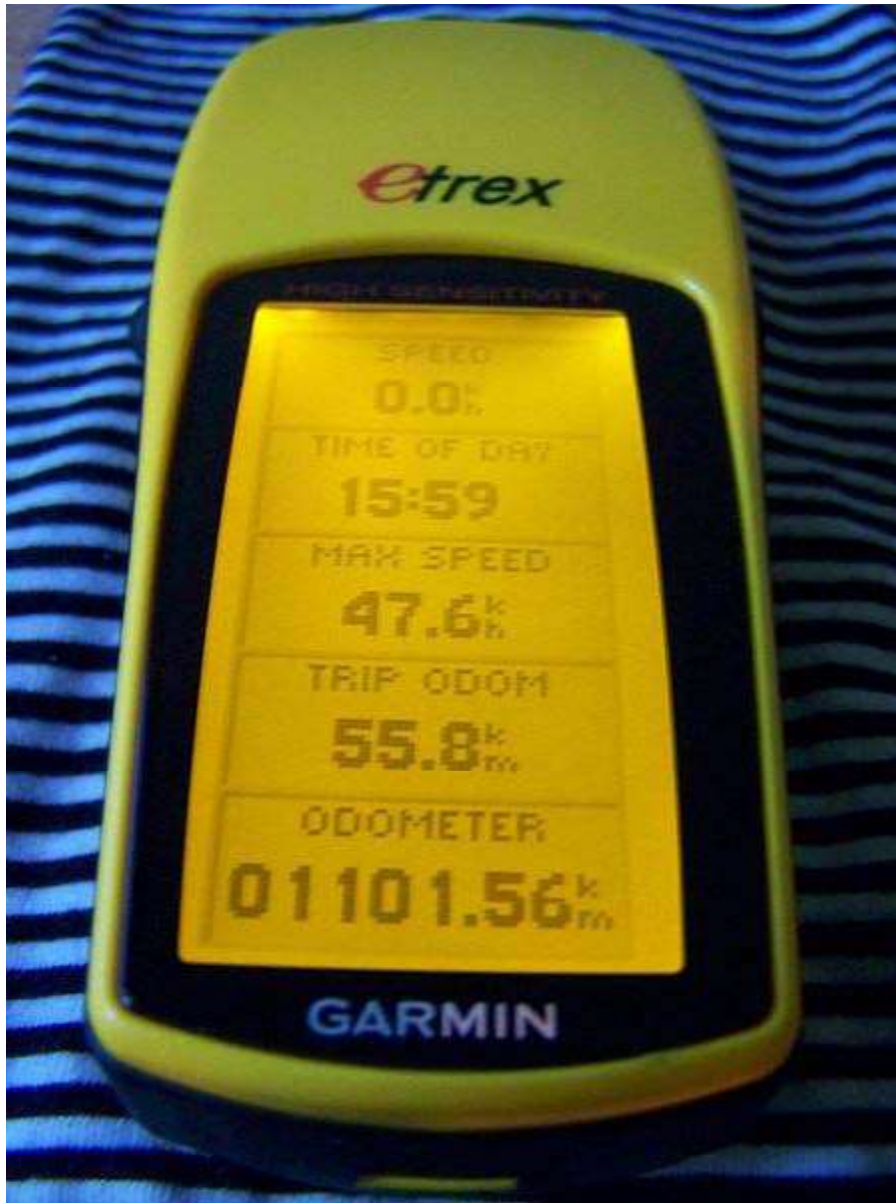
A Garmin etrex H GPS receiver, showing an odometer, trip odometer as well as speed related information
