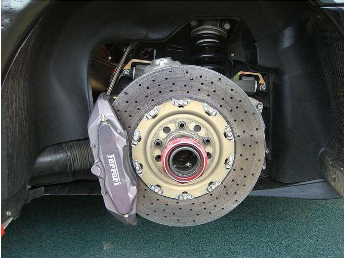
A reinforced carbon brake disc installed on a Ferrari F430 Challenge race car
