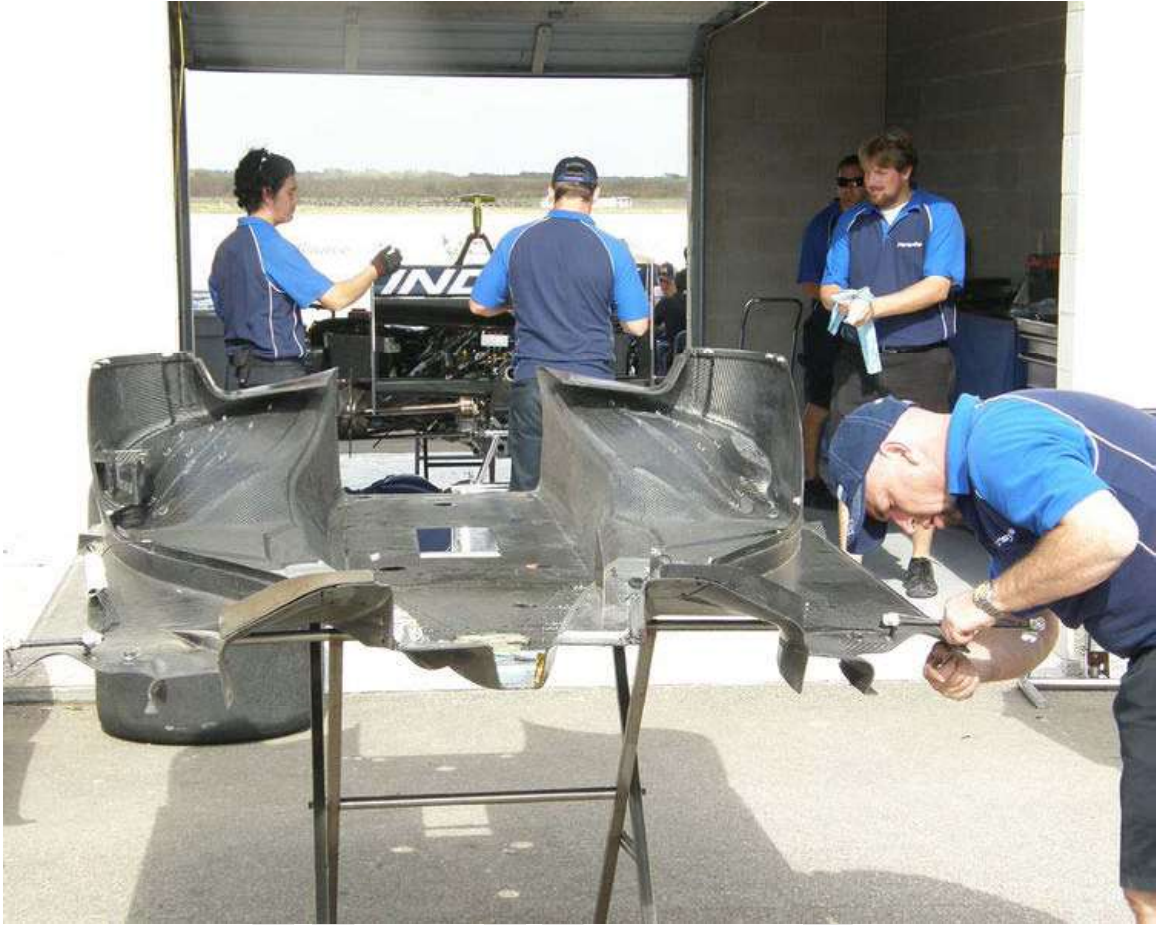
The bottom panel of the Panoz DP01 ChampCar exhibiting complex aerodynamic design.
