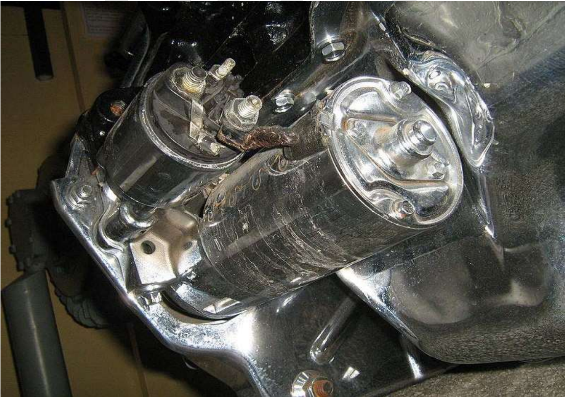
Typical starter installed underneath and toward the rear of an automobile engine
