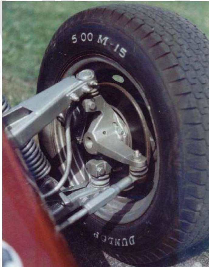
Part of car steering mechanism: tie rod, steering arm, king pin axis (using ball joints).
