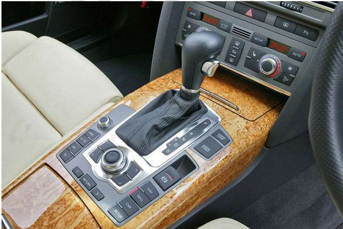
a right-hand drive 2005 Audi A6 (C6), showing the Multi Media Interface (MMI) controls
