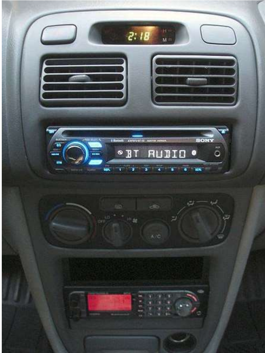
Uniden BCT-15 radio scanner installed with aftermarket head unit
