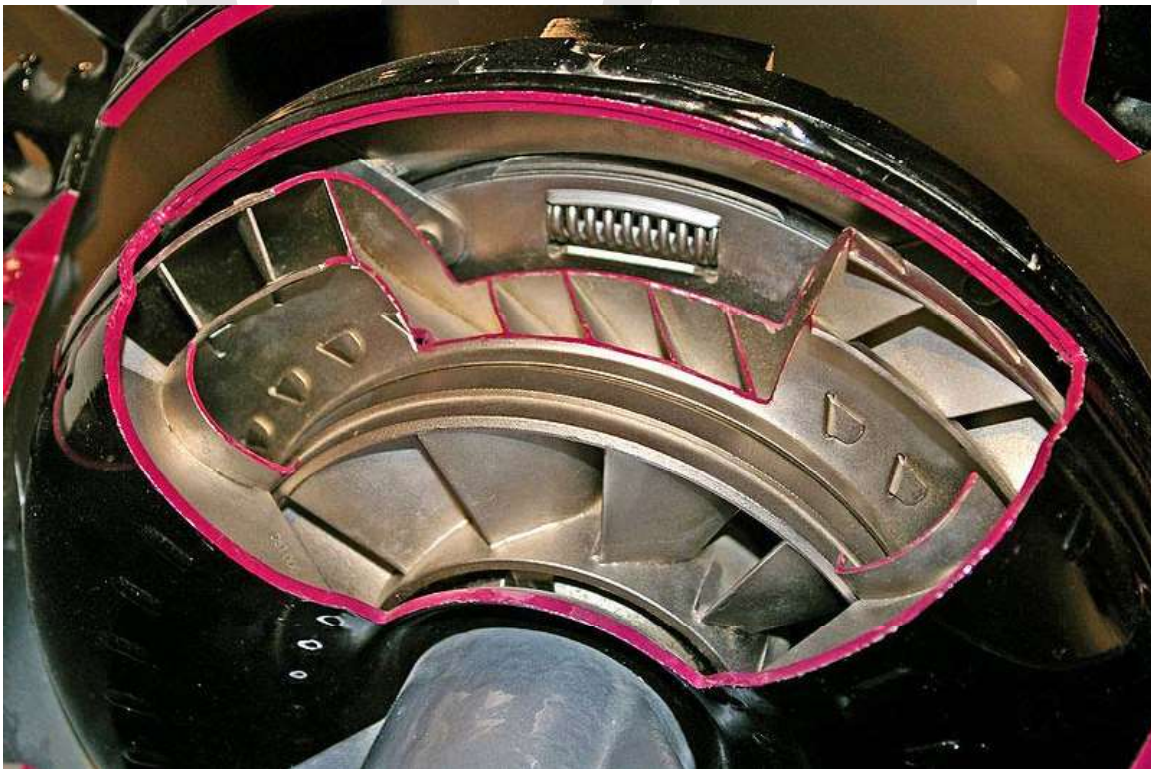
A cut-away model of a torque converter
