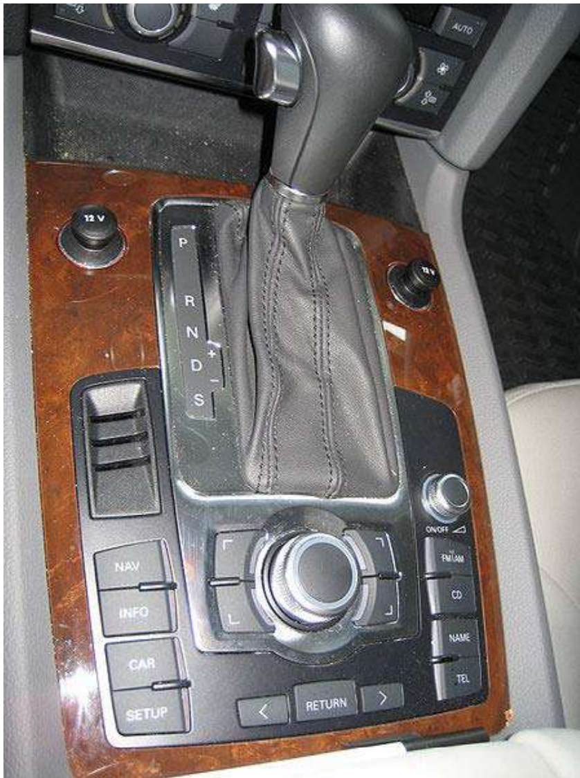
the MMI controls (to the rear of the gear lever) on a left-hand drive Audi Q7
