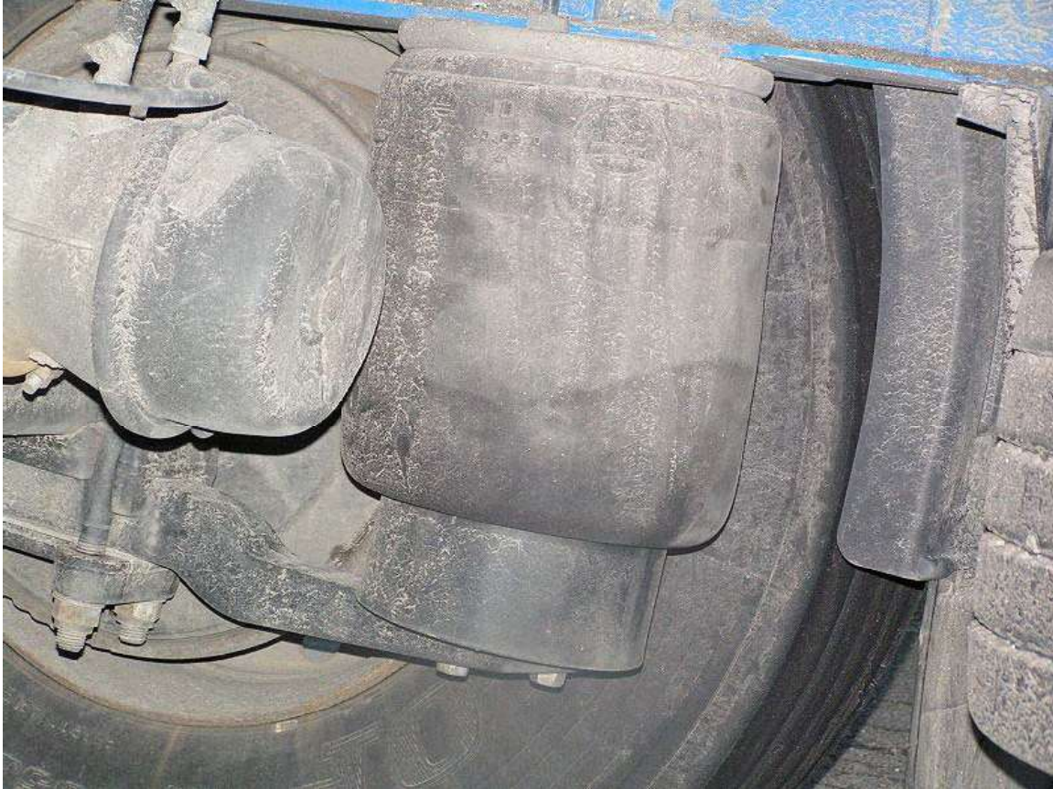
Pneumatic spring on a semitrailer
