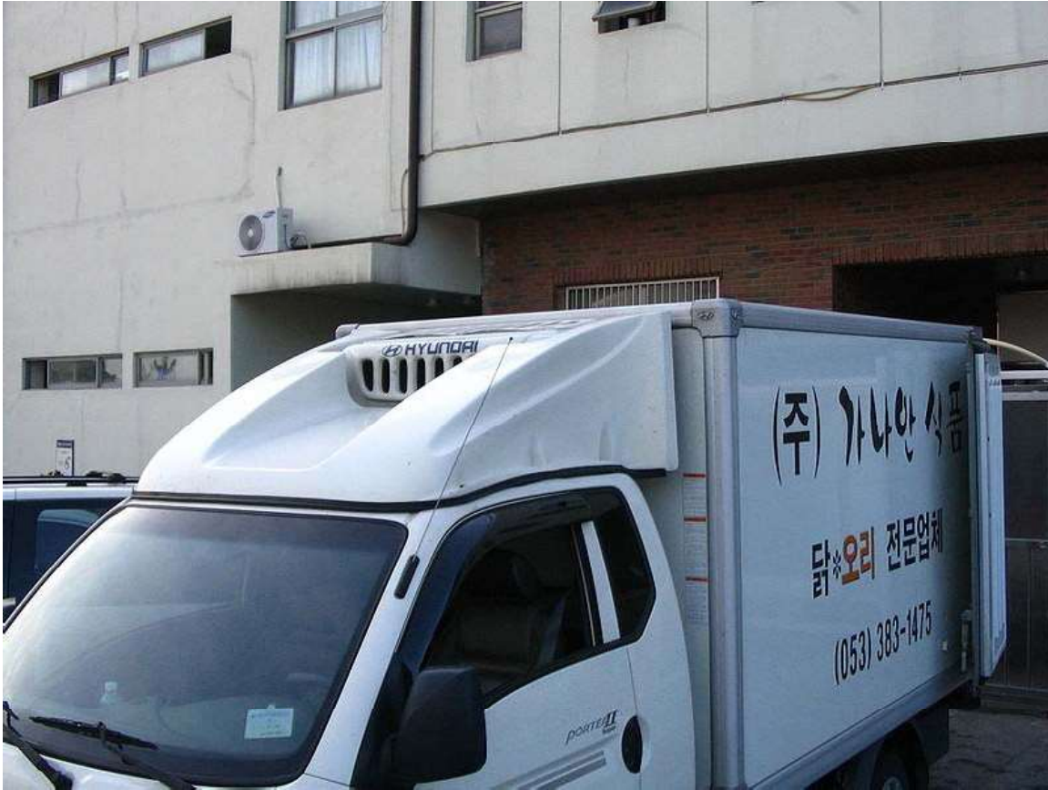
A truck with added bodywork on top of the cab to reduce drag.
