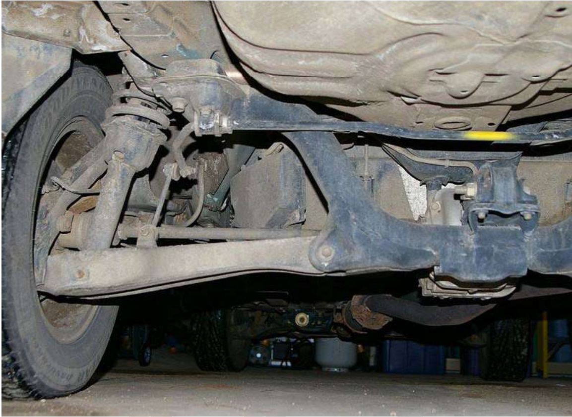
A rear independent suspension on an AWD car.
