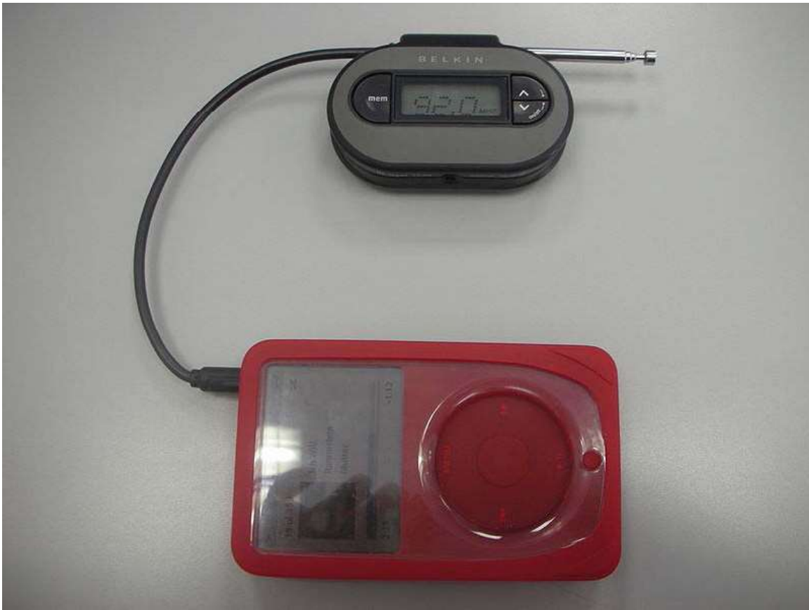
Belkin TuneCastII FM Transmitter with a modified antenna connected to a fifth generation iPod video.
