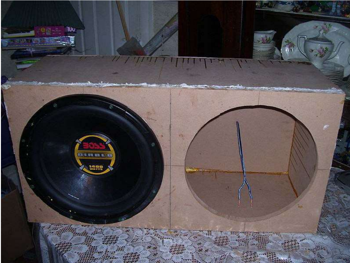
A homemade car audio subwoofer speaker box with a 15 inch Boss Audio subwoofer and an empty space for a second driver
