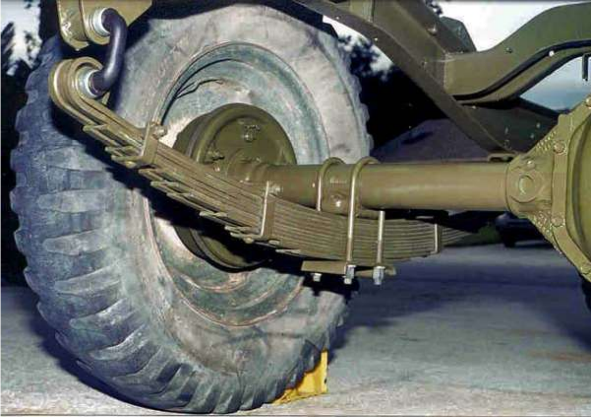
The rear suspension on a truck: a leaf spring.
