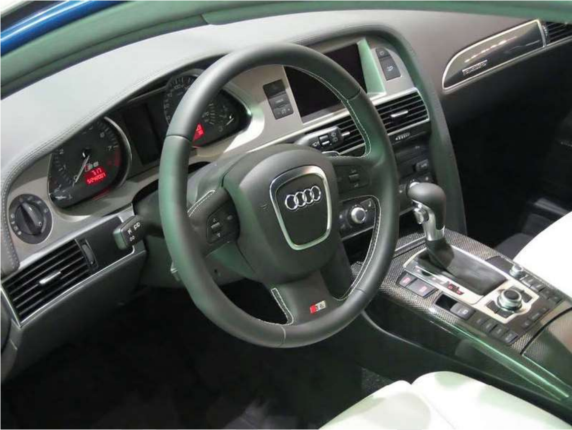
a left-hand drive 2007 Audi S6 (C6), showing the MMI controls, and the display screen in the dashboard
