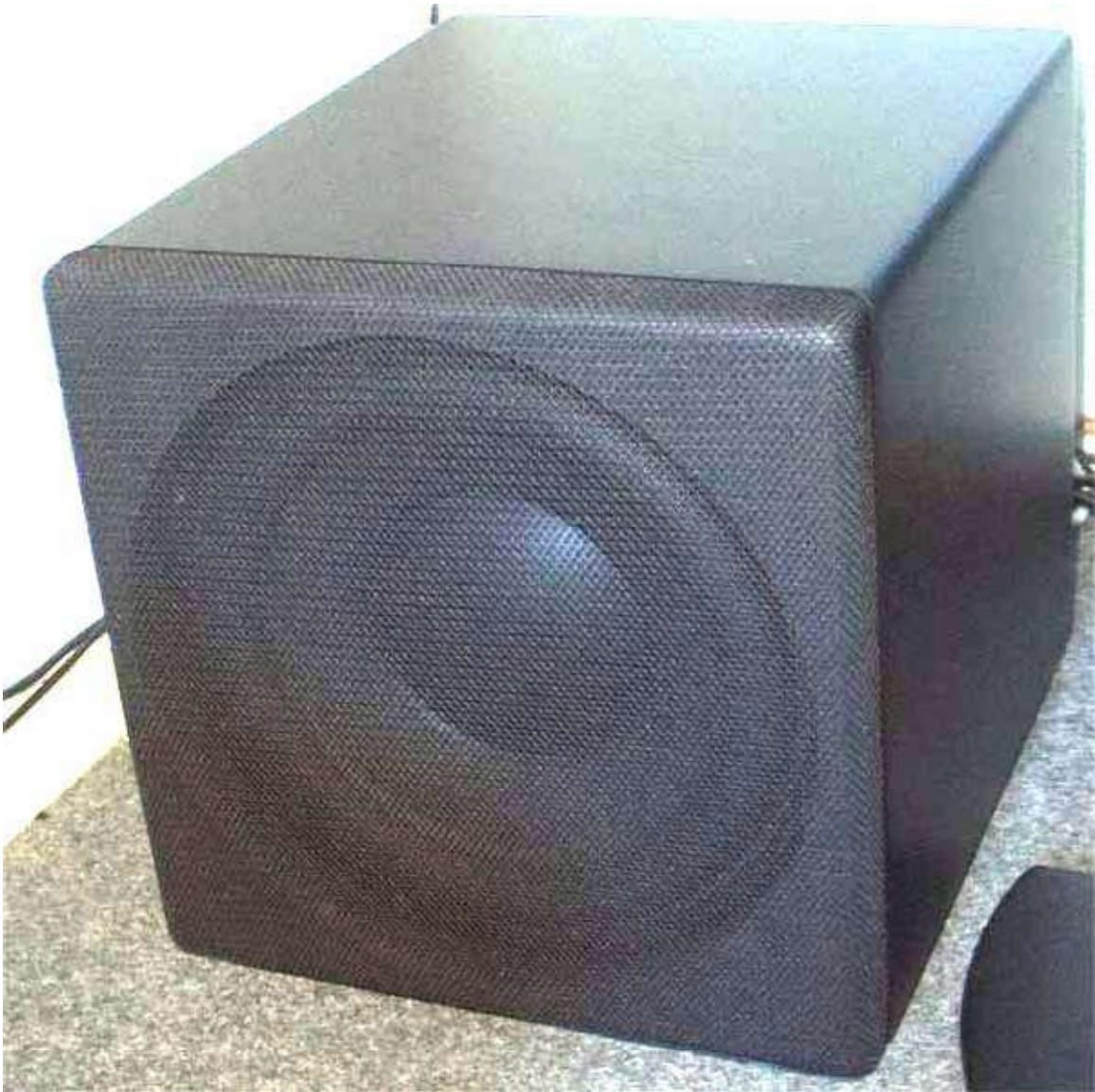
Subwoofer mounted in a sealed enclosure
