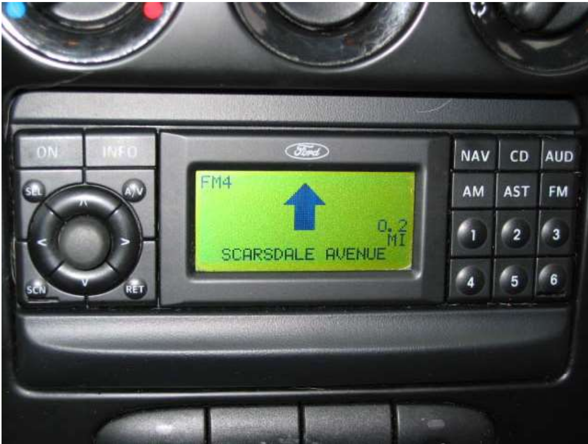
Early Factory Navigation System (as fitted to 1997 UK Specification Ford Mondeo)
