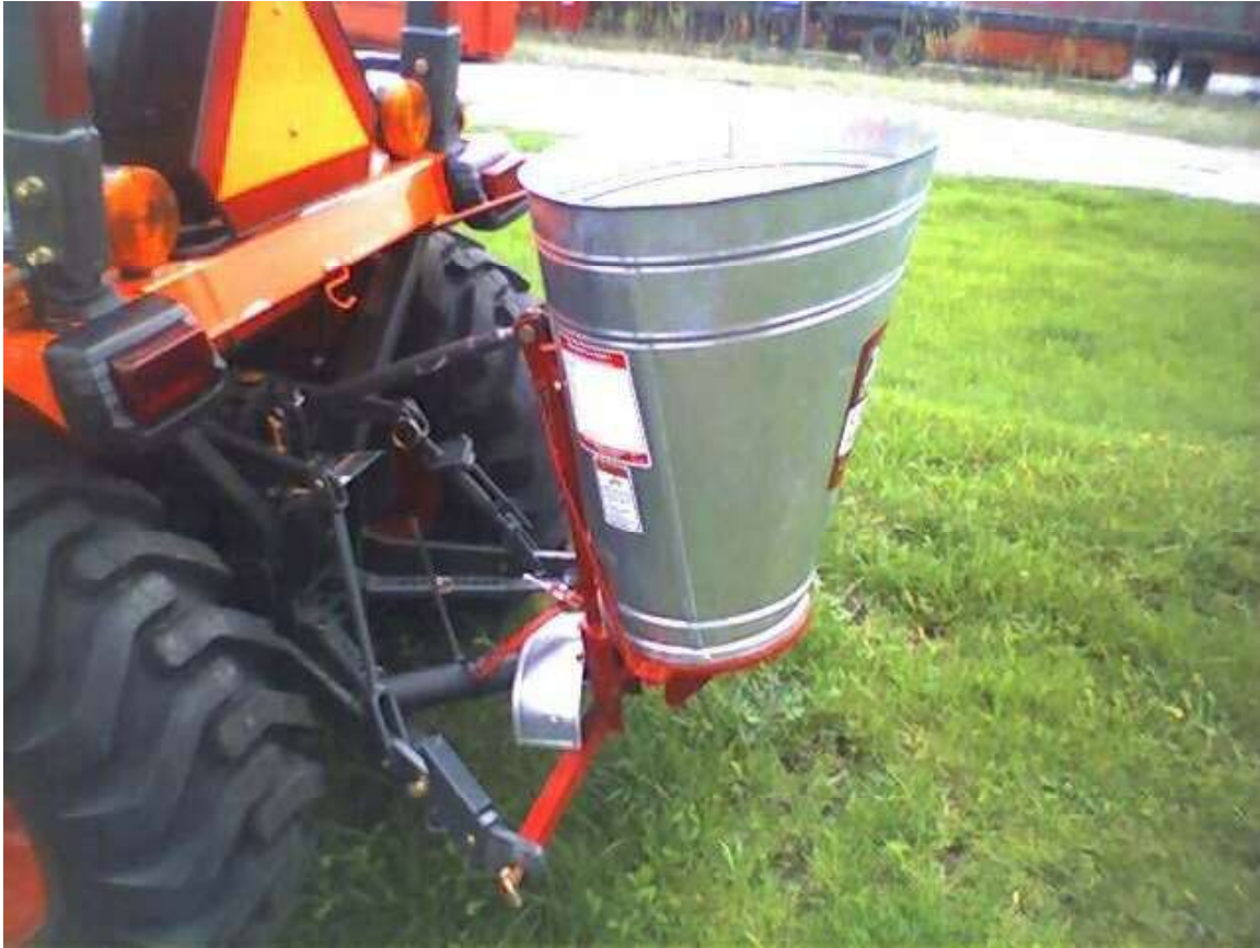
Side view of a small broadcast seeder showing three-point hitch and PTO shaft
