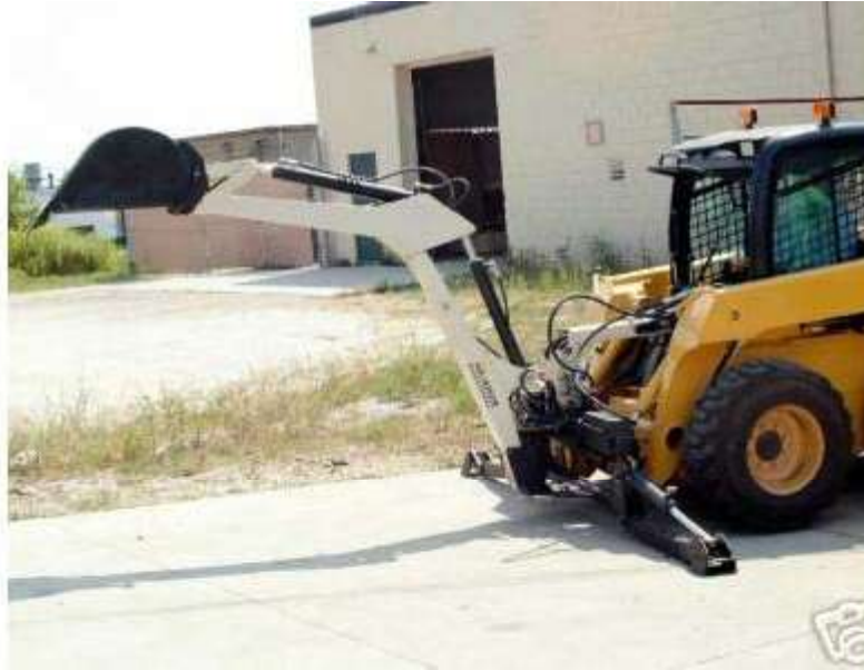
A skid loader with its bucket replaced by backhoe attachment
