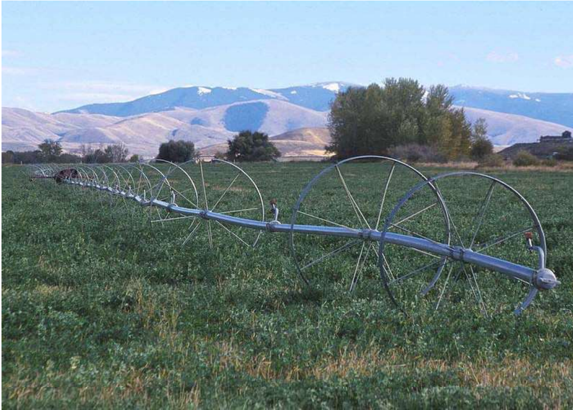
Wheel line irrigation system in Idaho. 2001. Photo by Joel McNee, USDA Natural Resources Conservation Service.
