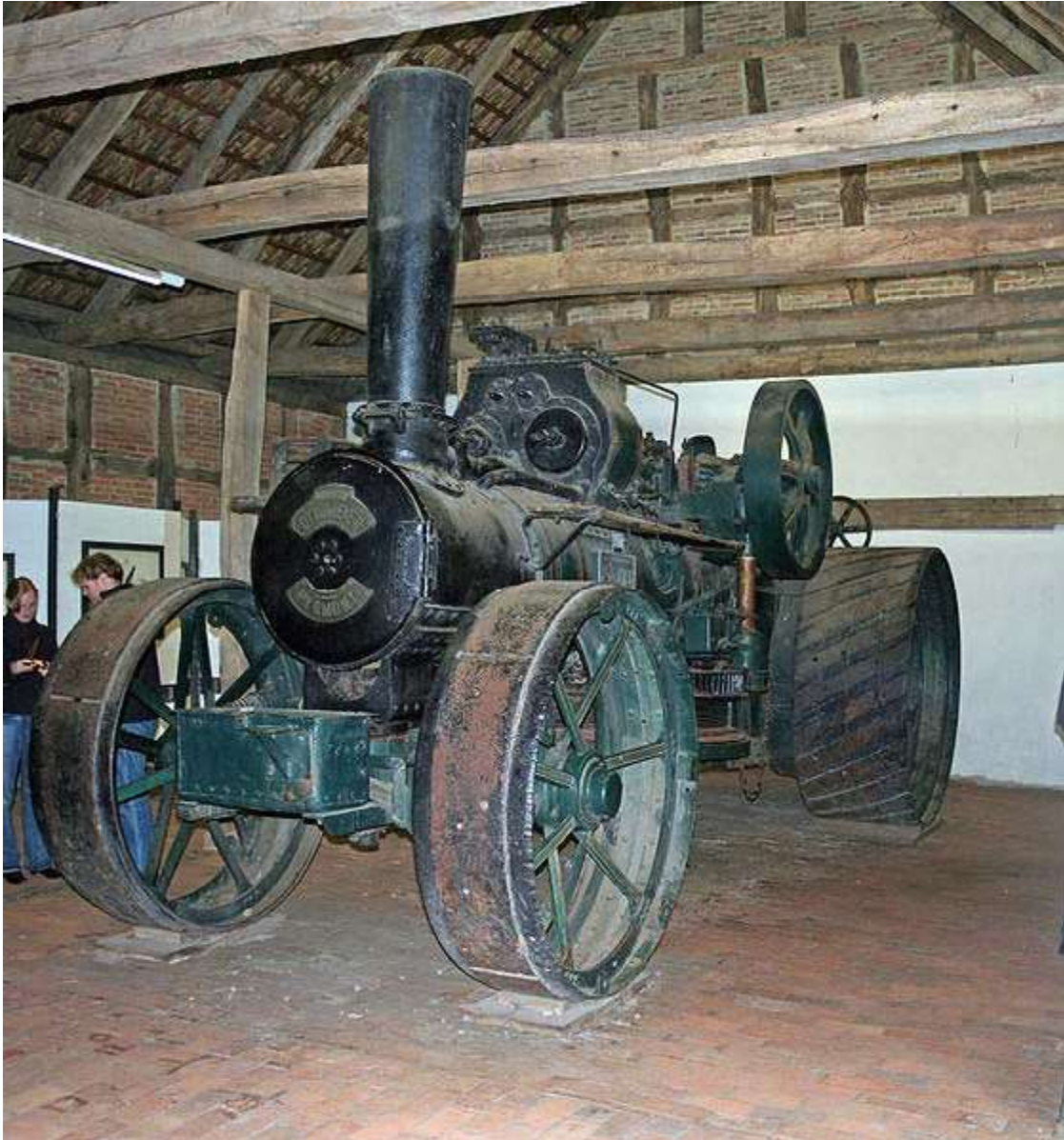
Ploughing engine Heumar , made by the Ottomayer company (Germany), used in pairs with a balance plough. Built 1929, 220 PS, 21 tons.
