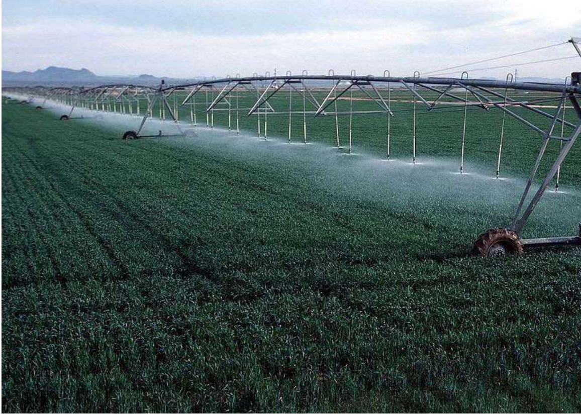
Center pivot with drop sprinklers. Photo by Gene Alexander, USDA Natural Resources Conservation Service.
