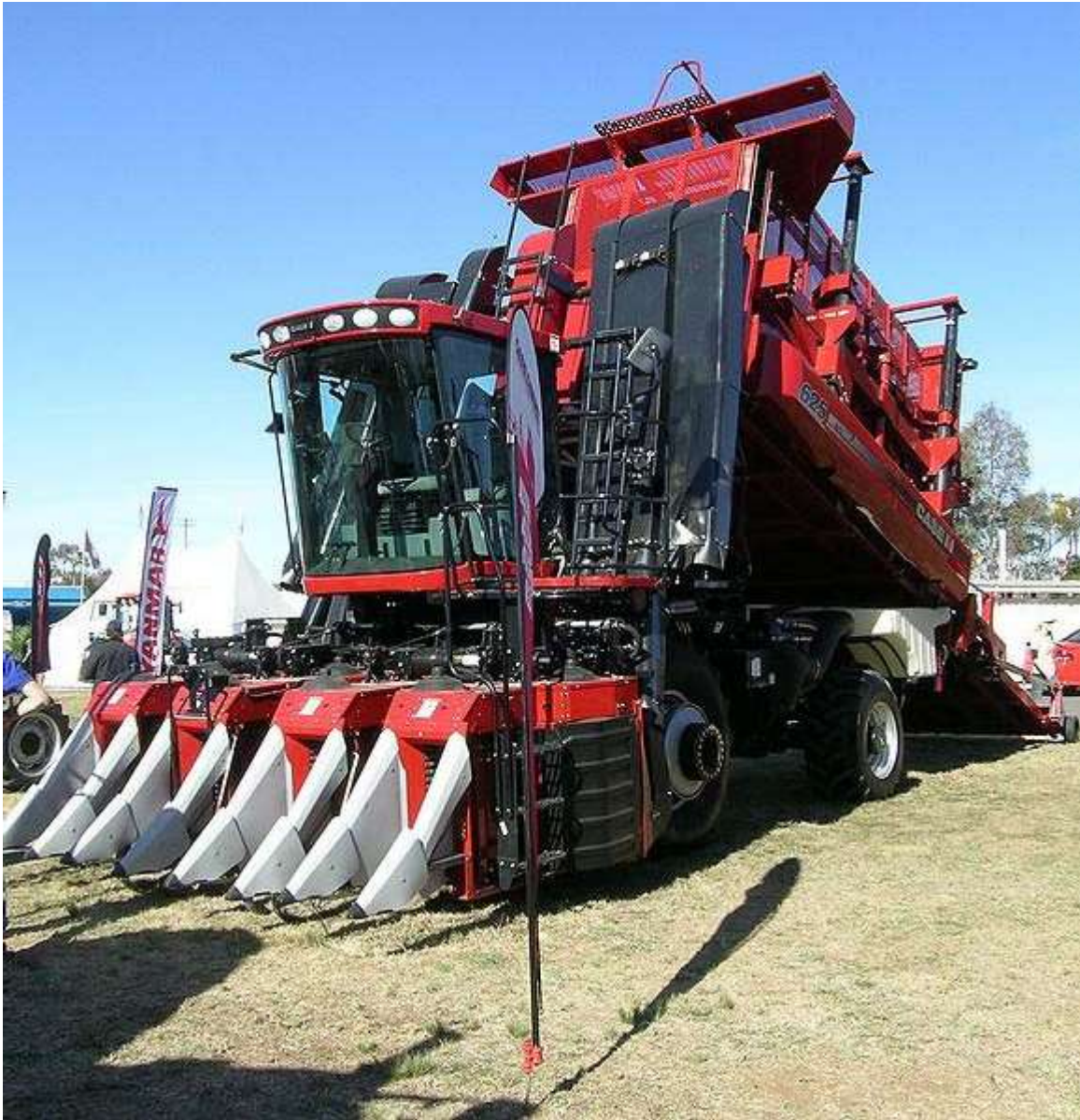
Case IH Module Express 625 picks cotton and simultaneously builds cotton modules.
