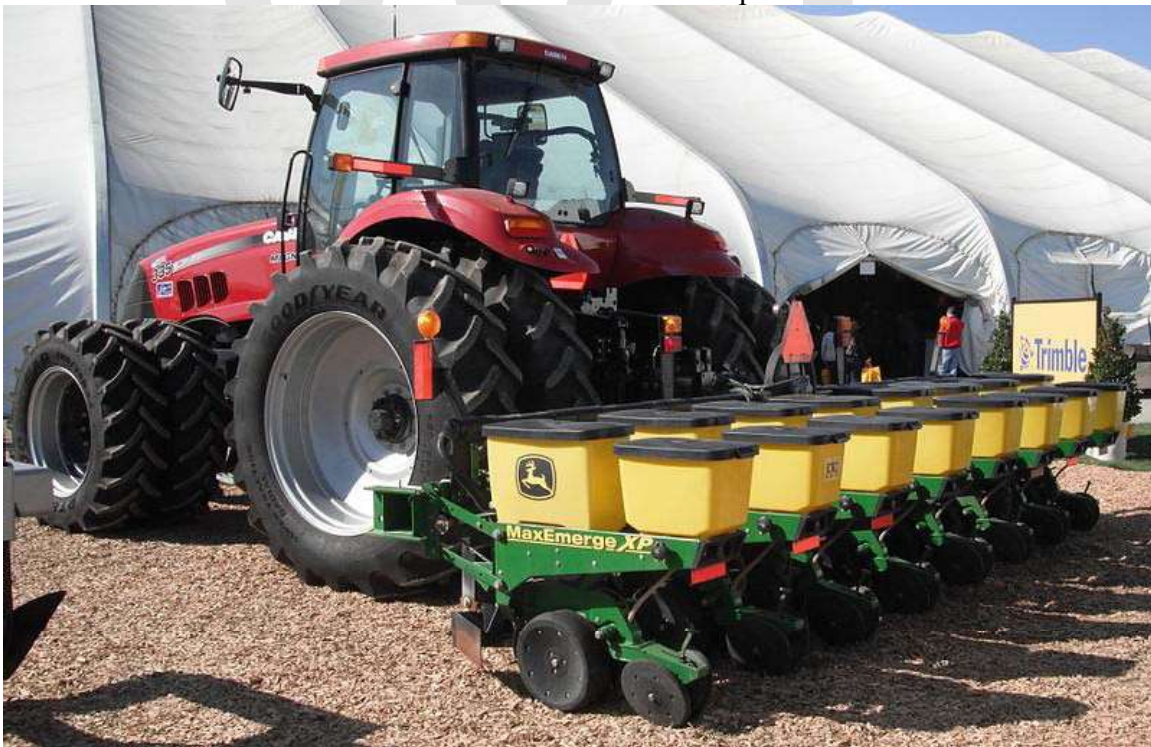
John Deere MaxEmerge XP Planter with Case IH AFS precision farming system which auto-steers using GPS
