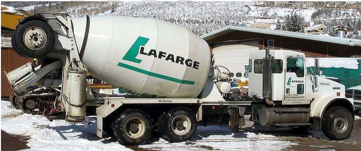
A rear-discharge concrete transport truck
