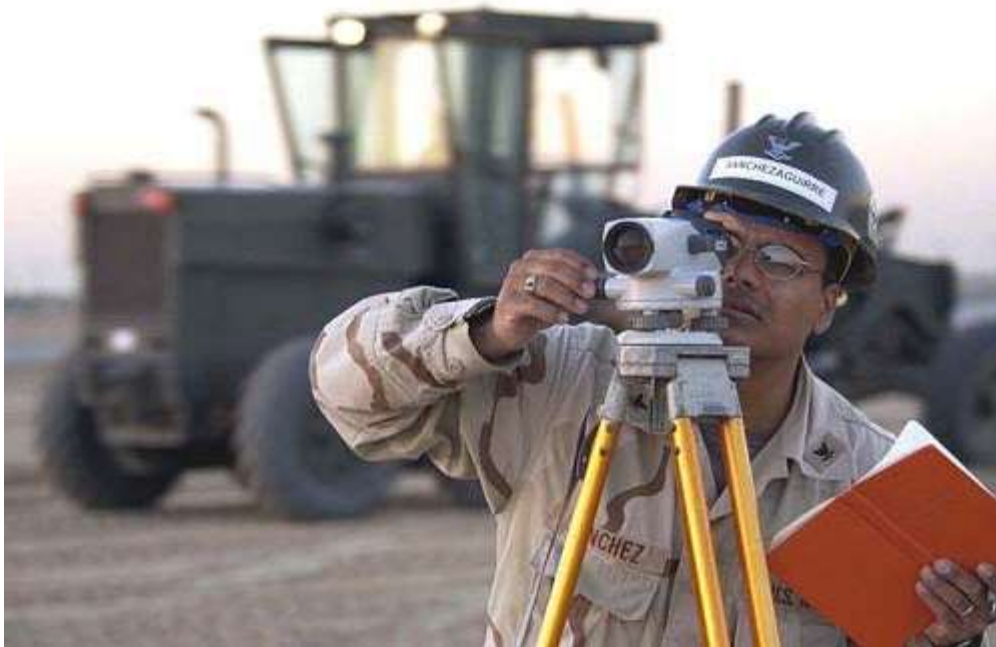
US Navy Surveyor at work with a leveling instrument.
