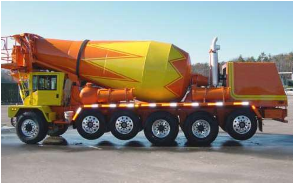
Terex Advance front discharge truck with three lift axles including one tag axle
