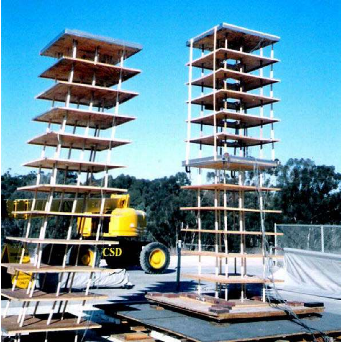
Testing base-isolated (right) and regular (left) building model
