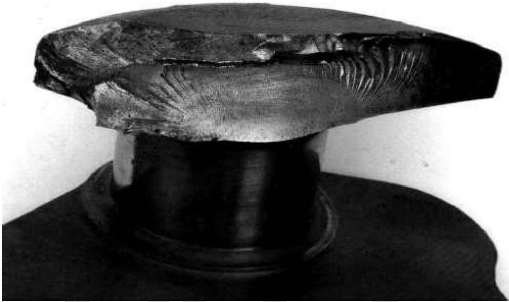
Crankshaft fatigue fracture
