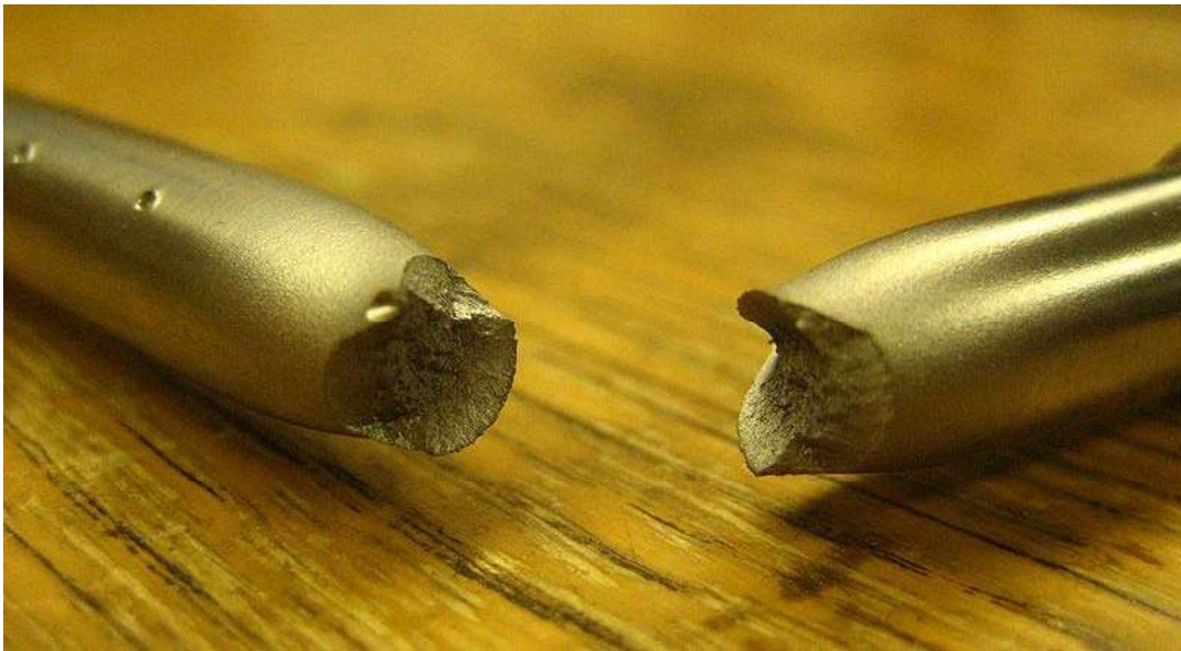
Ductile failure of a specimen strained axially.
