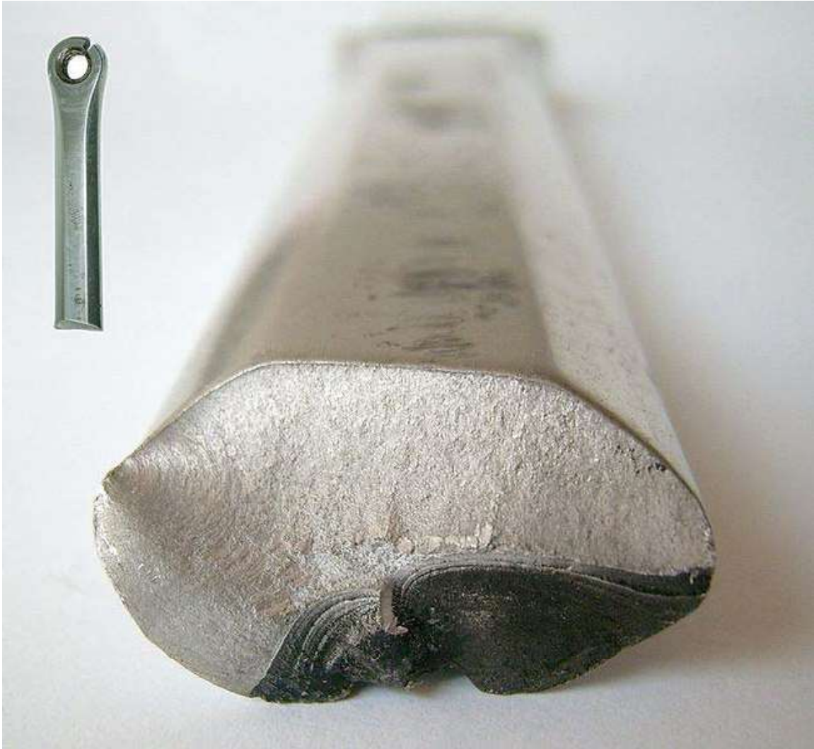
Fracture of an Aluminum Crank Arm. Bright: Brittle fracture. Dark: Fatigue fracture.
