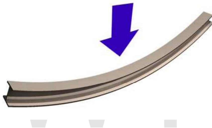
Bending of an I-beam
