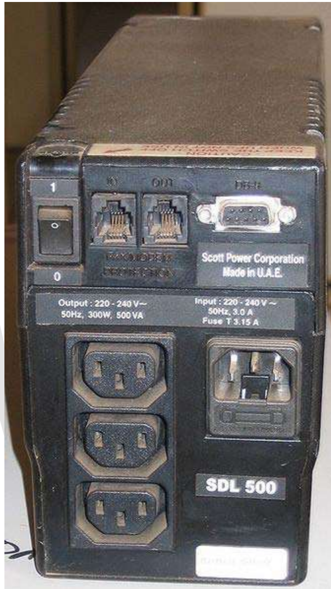
The unit in the photo has IEC connector inputs and outputs
