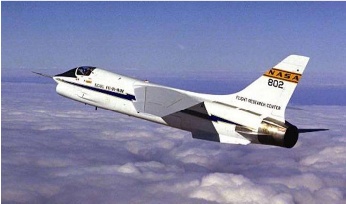
F-8C Crusader digital fly-by-wire testbed
