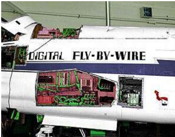
Green colored flight control wiring of a test aircraft
