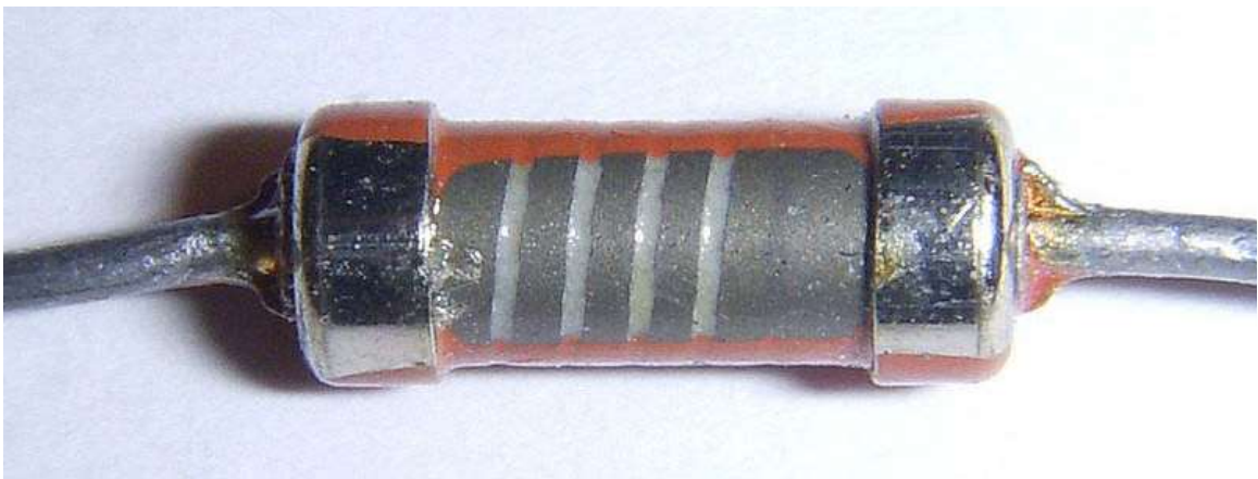
Partially exposed Tesla TR-212 1 k \Omega carbon film resistor
