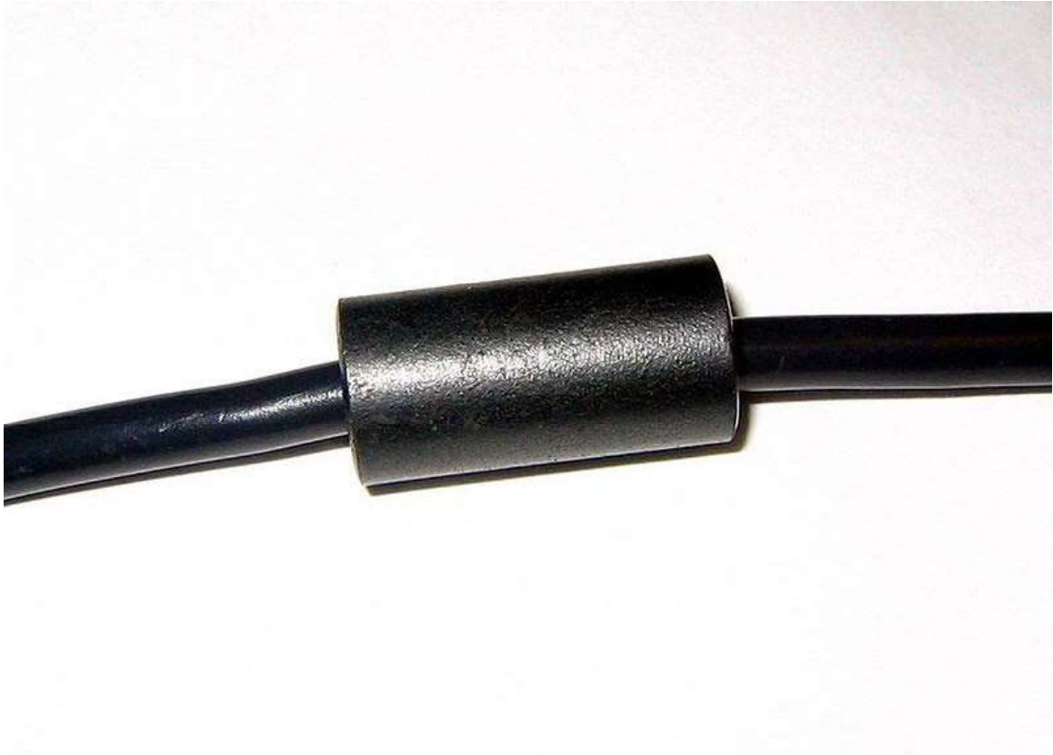
A ferrite ring on a computer data cable.
