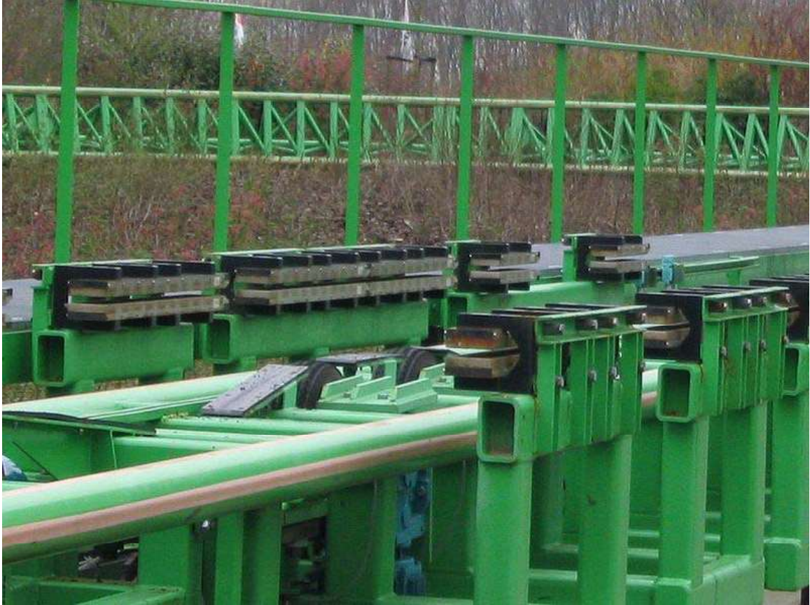
Eddy current brakes at the Intamin roller coaster Goliath in Walibi World (Netherlands)
