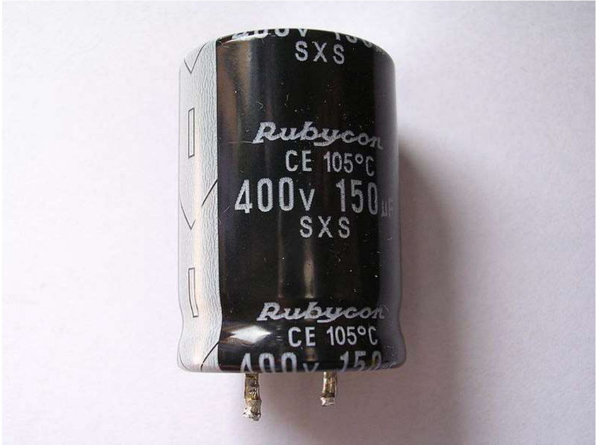
A typical electrolytic capacitor
