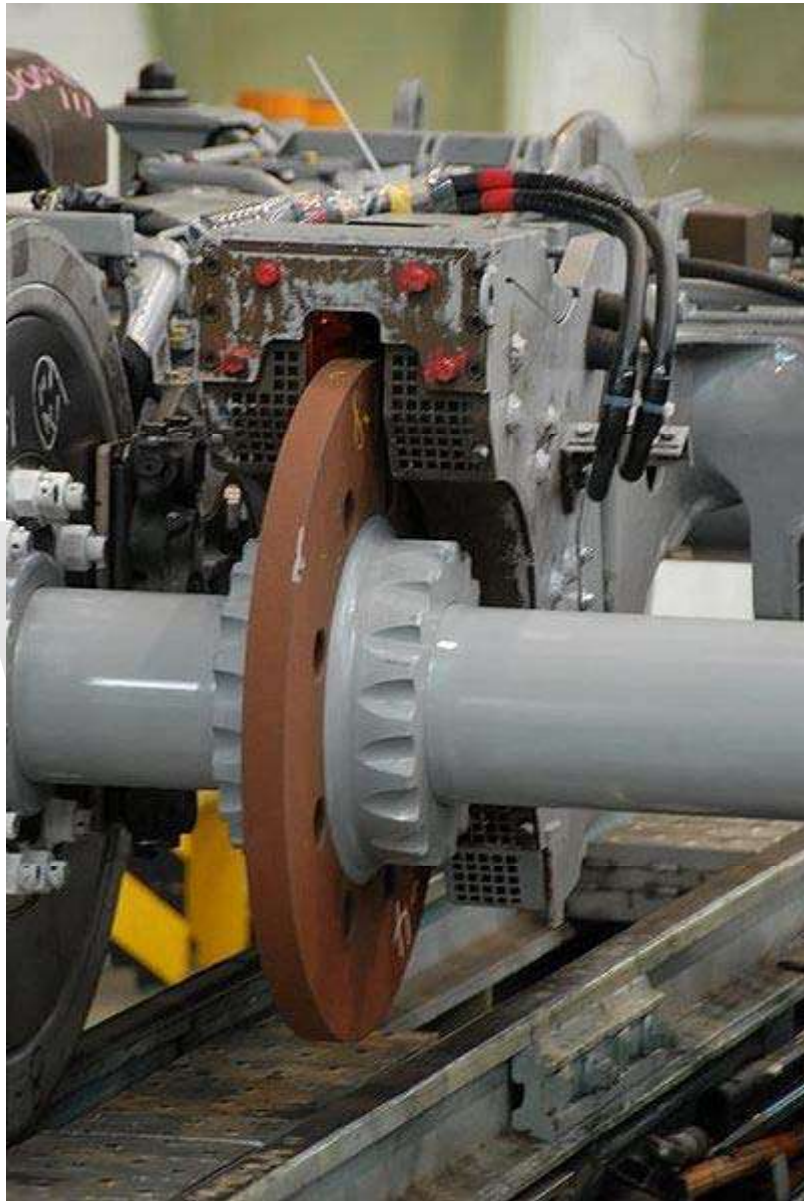
Circular eddy current brake on 700 Series Shinkansen
