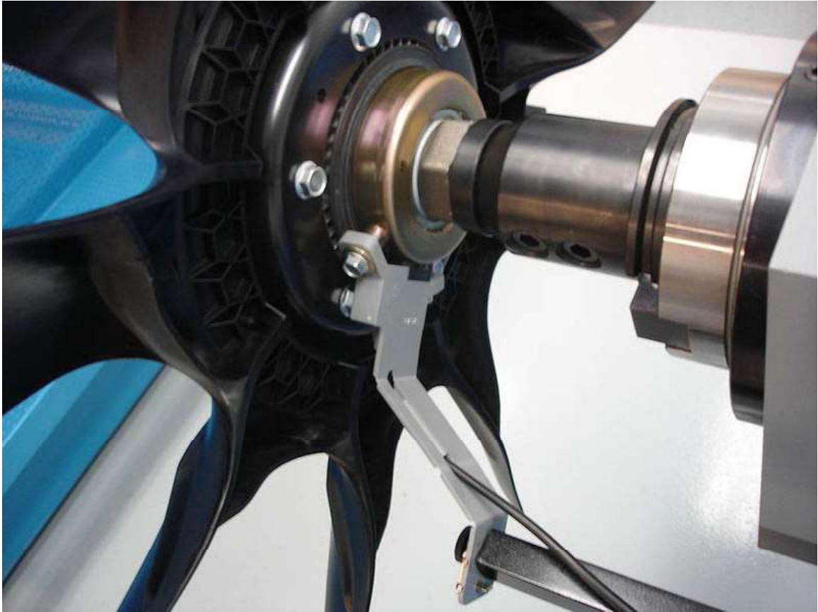
Clutch with Hall Effect sensor.
