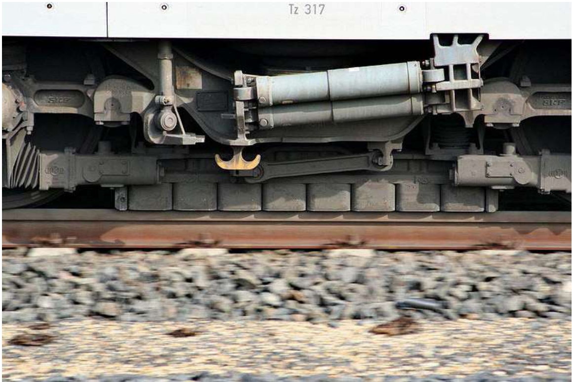
An eddy current brake of a German ICE 3 in action.
