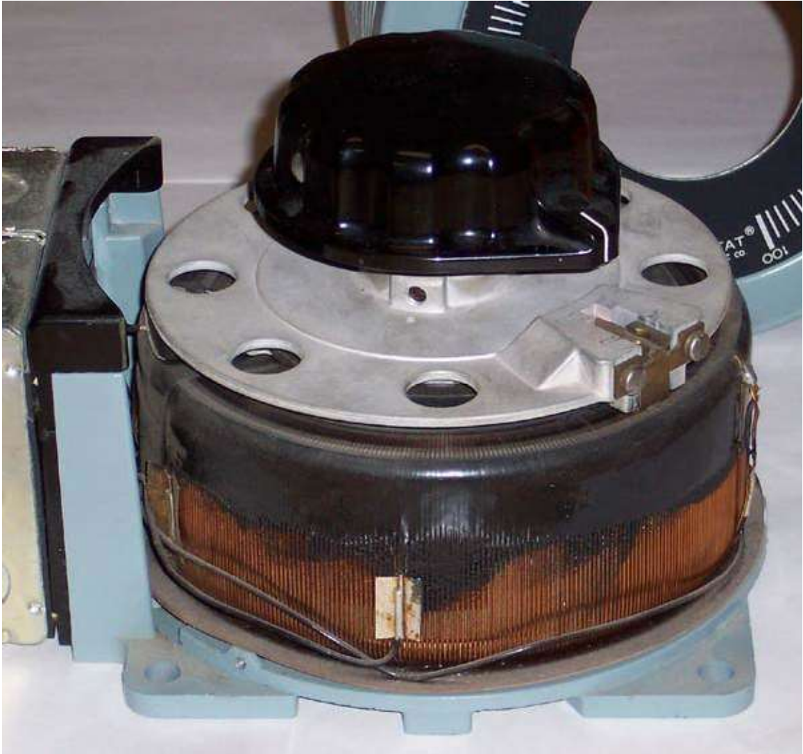
A variable autotransformer
