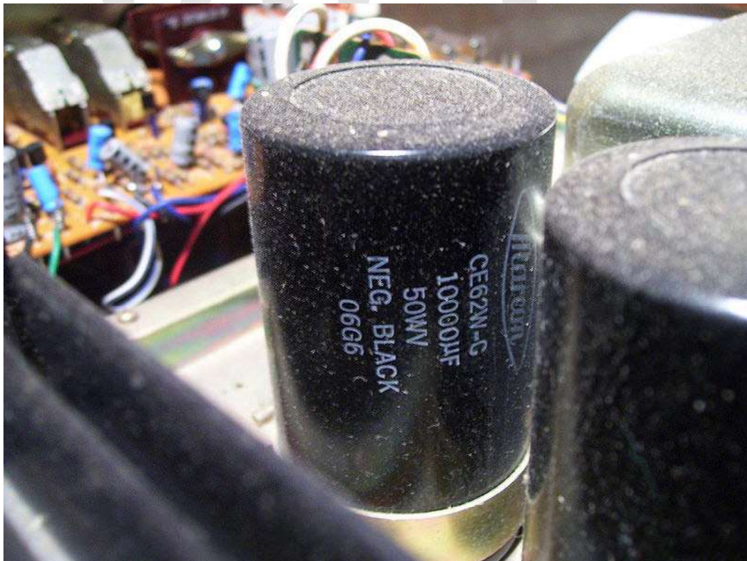
A 10,000 microfarad capacitor in a TRM-800 amplifier
