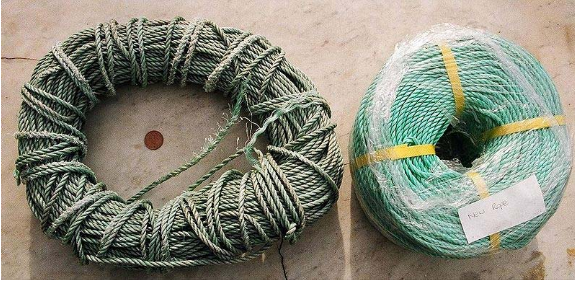
UV damaged polypropylene rope (left) and new rope (right)
