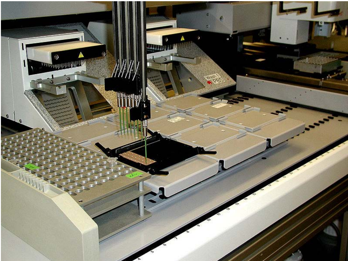
Robotic preparation of MALDI mass spectrometry samples on a sample carrier.
