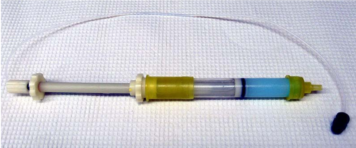
Nickel-affinity column. The resin is blue since it has bound nickel.
