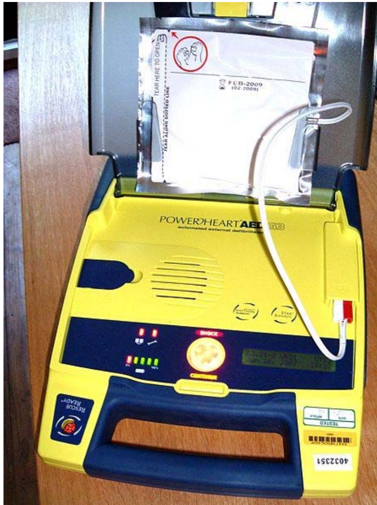
An automated external defibrillator, open and ready for pads to be attached
