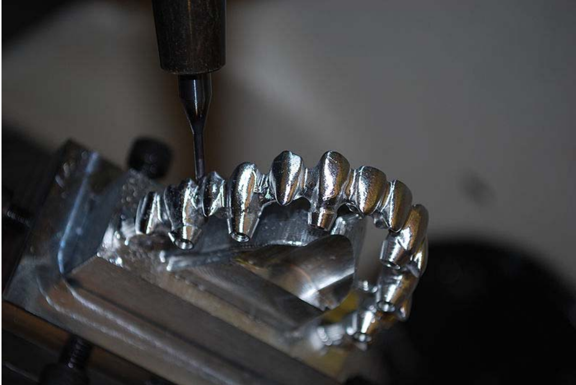
Full dental bridge being machined using WorkNC Dental CAD/CAM software
