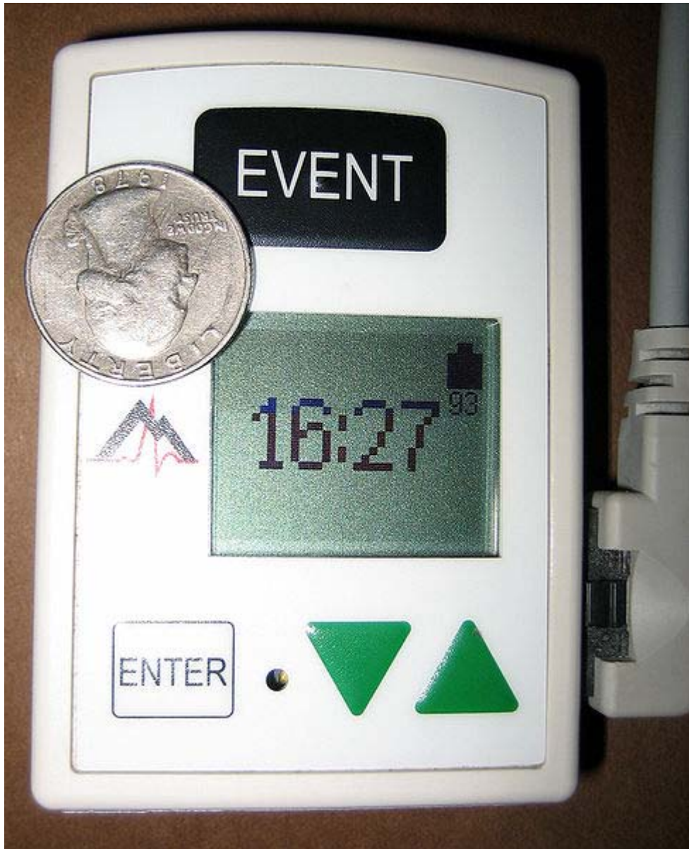
A Holter monitor with a US quarter dollar coin to show scale
