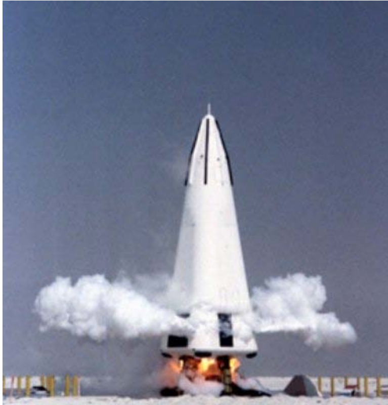
McDonnell Douglas DC-X used vertical takeoff and vertical landing
