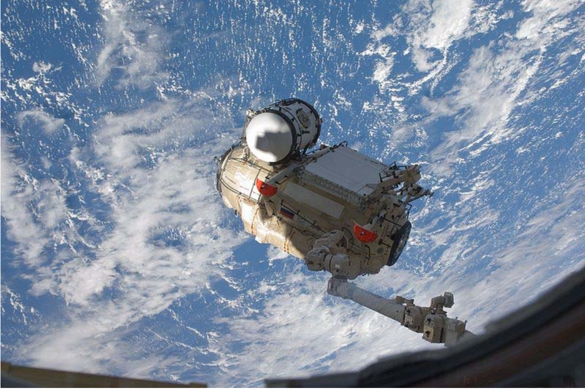
Canadarm2 transfers MRM-1 to the Earth-facing port of the Zarya module
