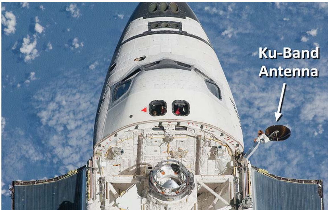
The failed Ku band dish antenna
