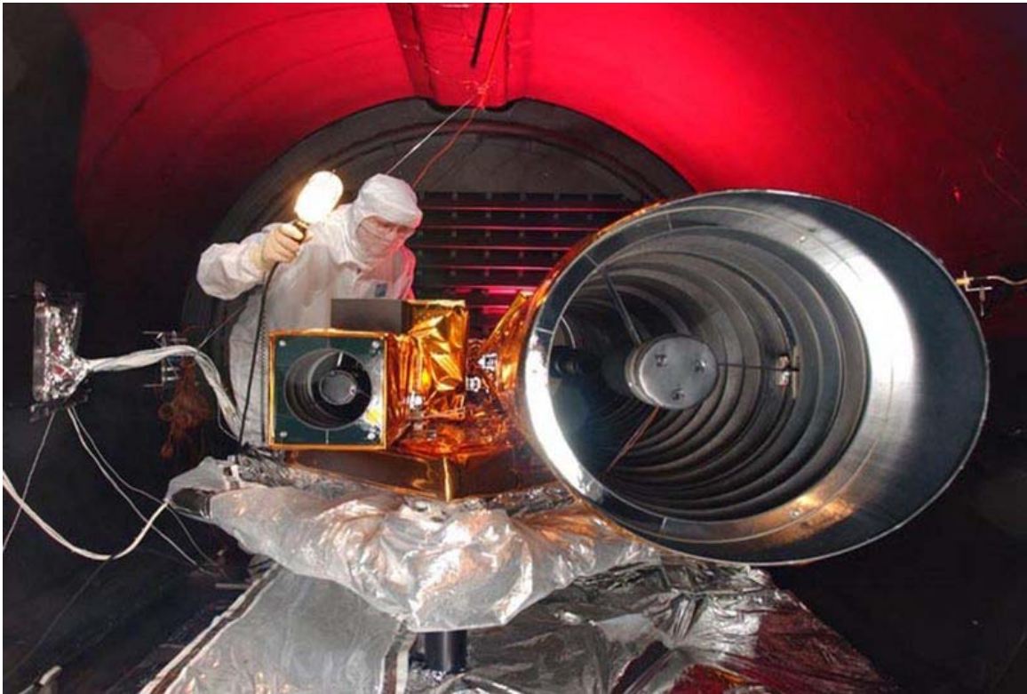
Cameras of the flyby spacecraft, HRI at right, MRI at left
