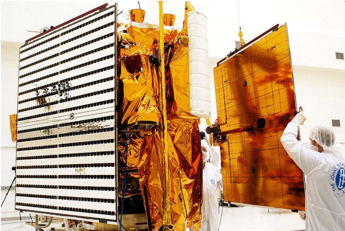
MESSENGER assembly installation of solar panels Astrotech
