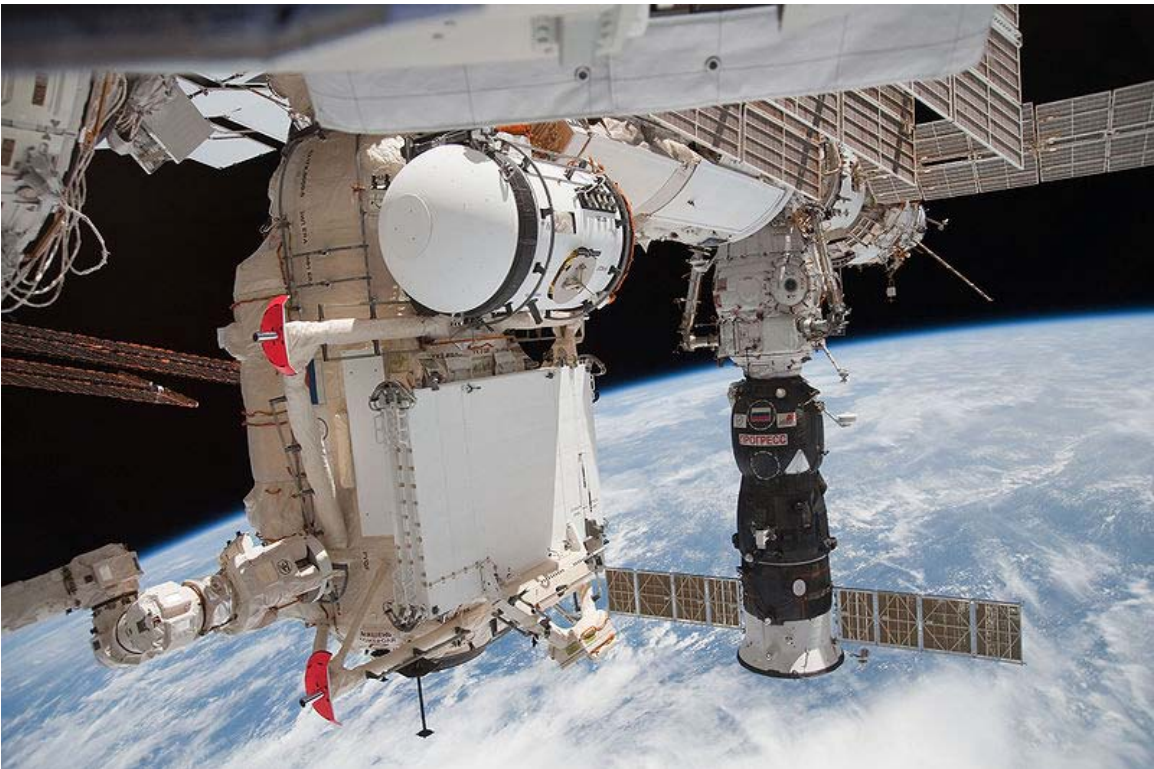
Canadarm2 attaches MRM-1 to the Zarya module
