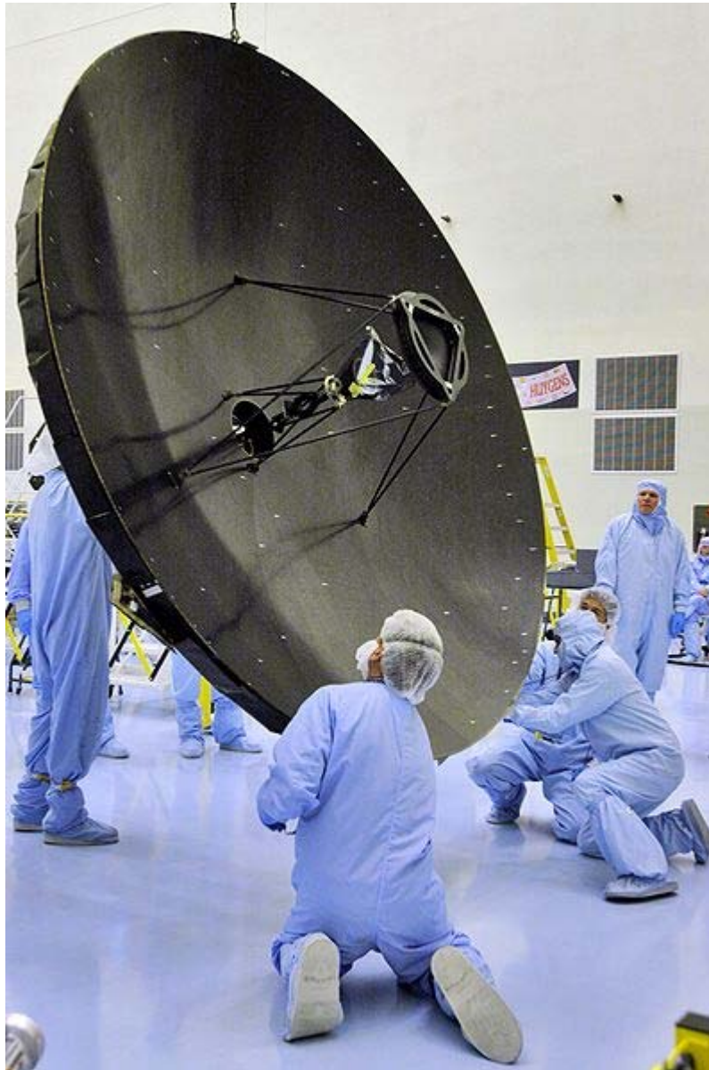
MRO High Gain Antenna installation
