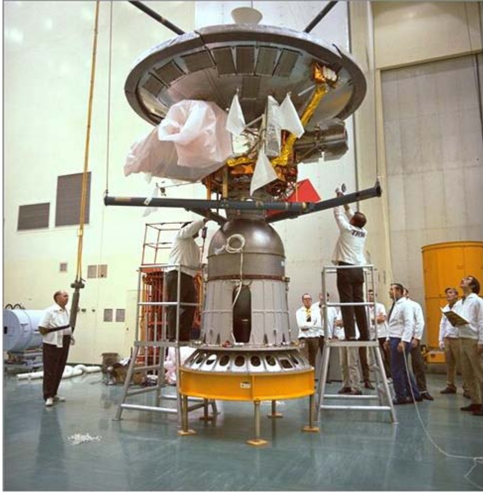
Pioneer 10 on a kick motor just prior to be encapsulated for launch
