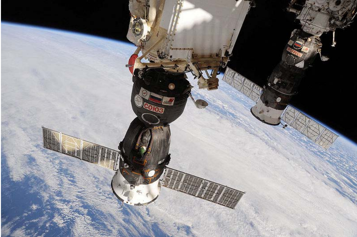
Soyuz TMA-19 spacecraft docked to Rassvet Mini-Research Module 1 (MRM1).
