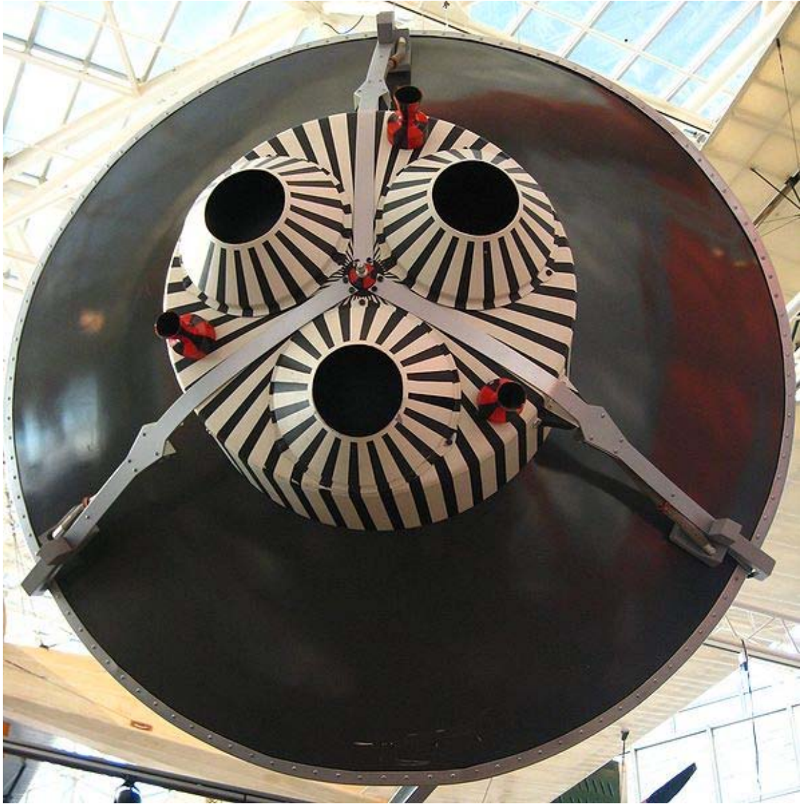
Mercury heat shield and retrorocket pack
