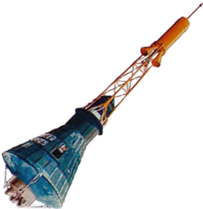
The Mercury spacecraft with escape tower
