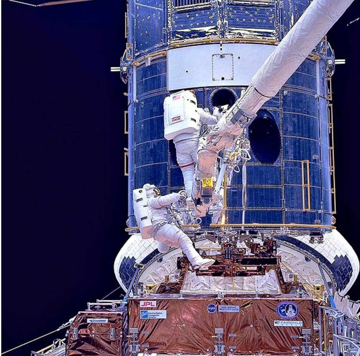
Astronauts installing corrective optics during SM1
