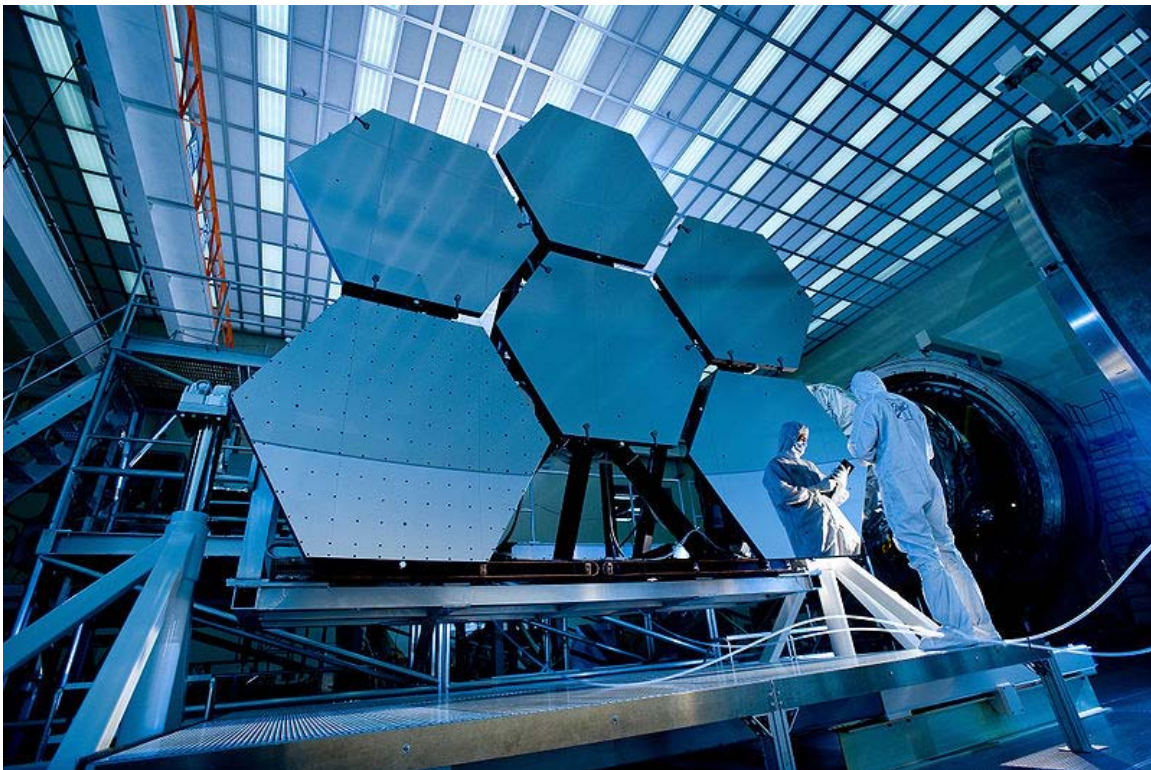
Six of the James Webb Space Telescope beryllium mirror segments undergoing a series of cryogenic tests at the X-ray & Cryogenic Facility at NASA's Marshall Space Flight Center in Huntsville, Alabama
