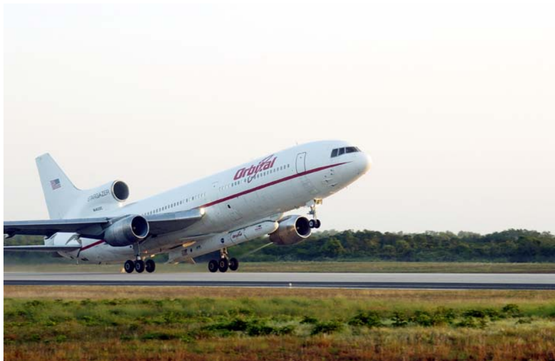
The Lockheed L-1011 Stargazer take-off with GALEX attached under-belly
