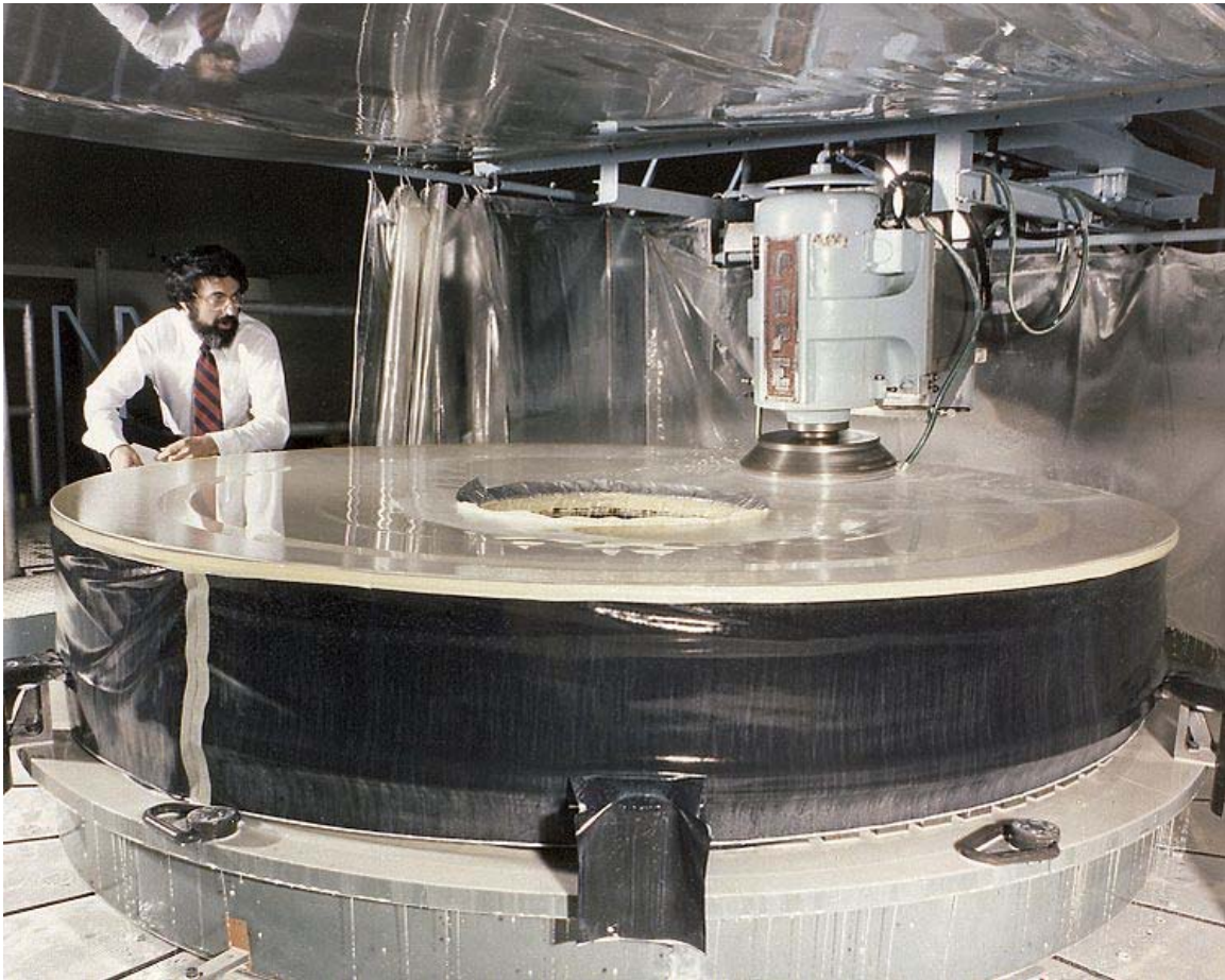
Polishing of Hubble's primary mirror begins at Perkin-Elmer corporation, Danbury, Connecticut, March 1979. The engineer pictured is Dr. Martin Yellin, an optical engineer working for Perkin-Elmer on the project.
