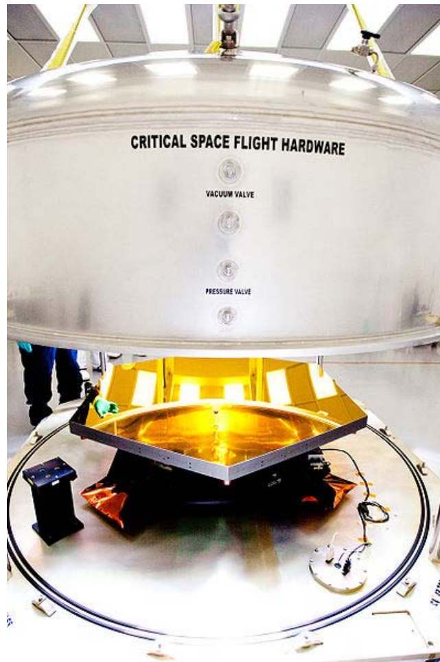
The James Webb Space Telescope's Engineering Design Unit (EDU) primary mirror segment, coated with gold
