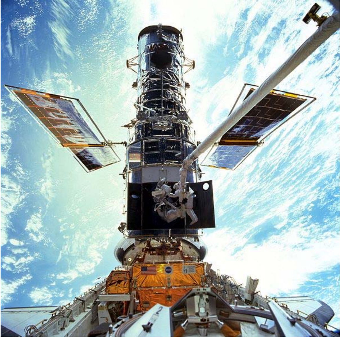
Astronauts replacing gyroscopes during SM3A
