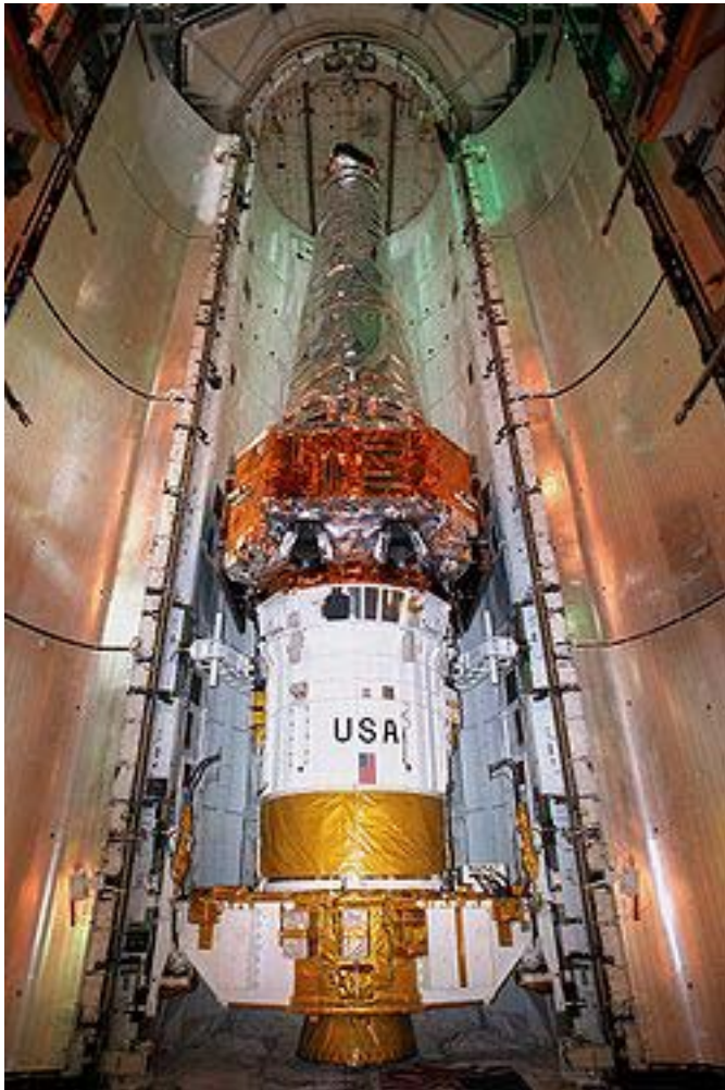
Chandra X-ray Observatory and Inertial Upper Stage sit inside the payload bay on Space Shuttle Columbia mission STS-93
