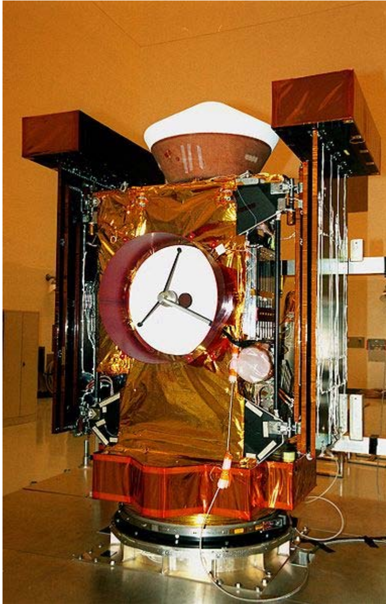
Stardust awaiting testing of the solar arrays.
