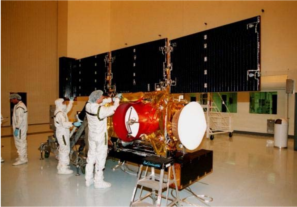
The solar arrays being checked in the Payload Hazardous Servicing Facility.
