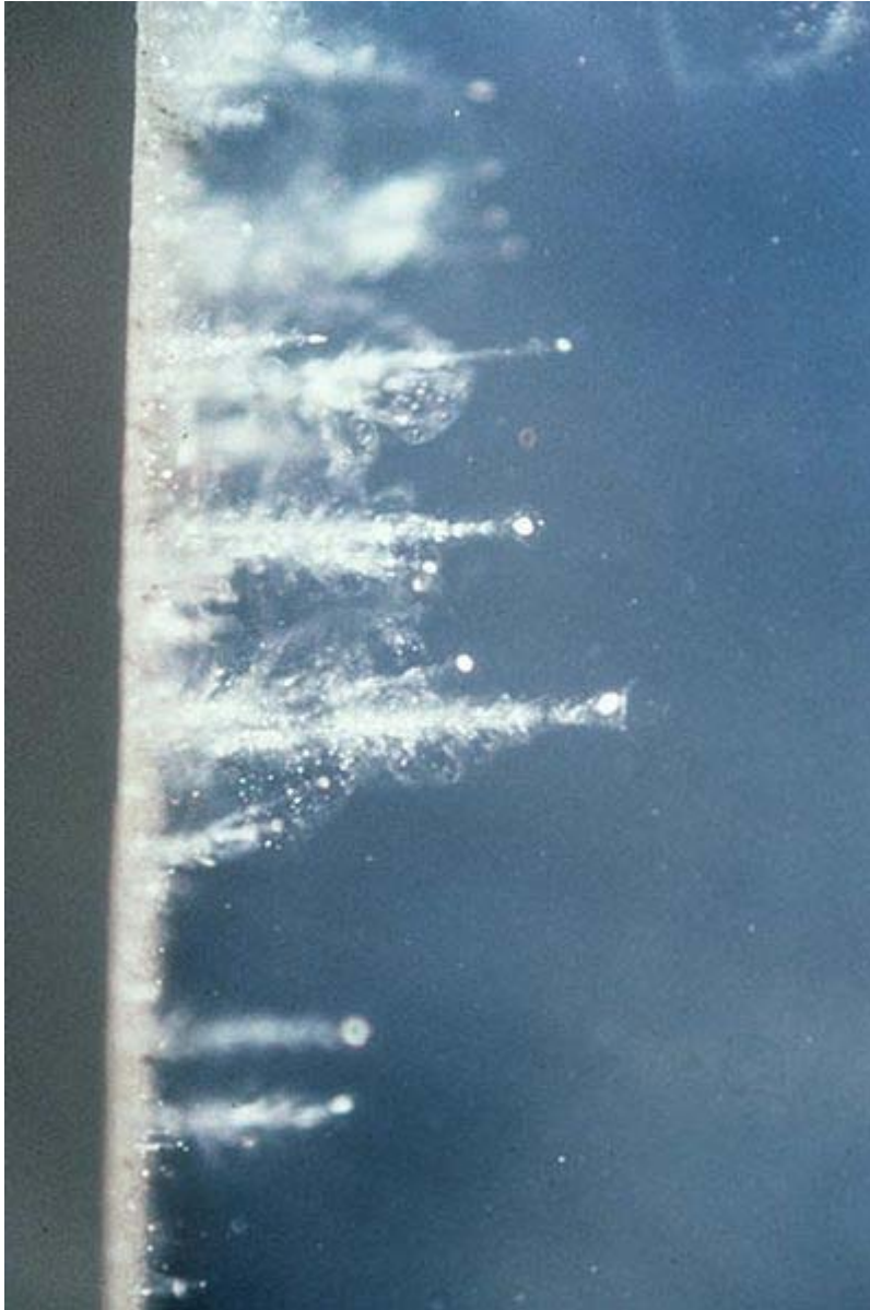
Visible dust grains in the aerogel collector.
