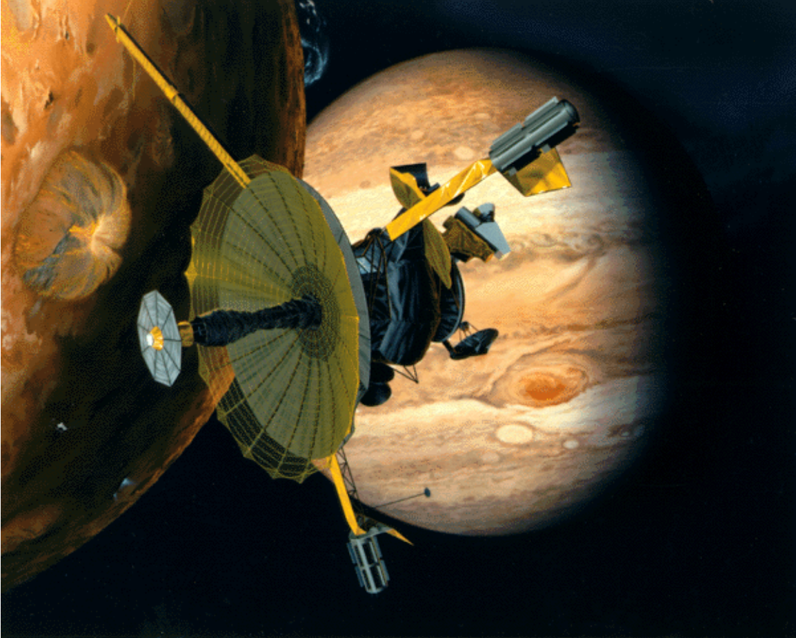
Artist's concept of Galileo at Io. Note the fully deployed high-gain antenna. Compare with below image.
