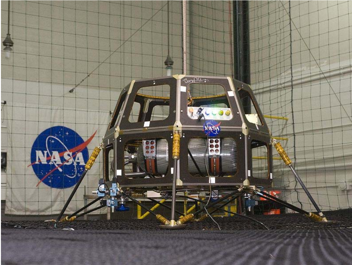
The Modular Common Spacecraft Bus that will become LADEE, being tested at NASA Ames Research Center in 2008.
