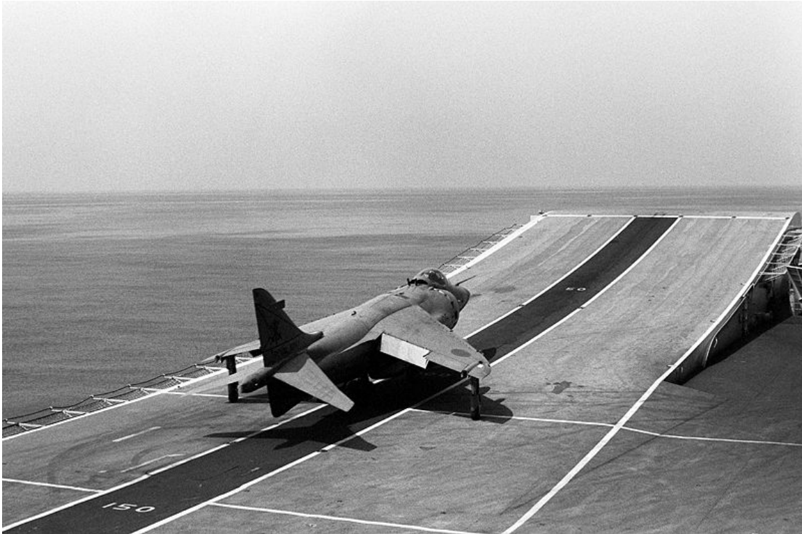
The ski-jump on Royal Navy carrier HMS Invincible
