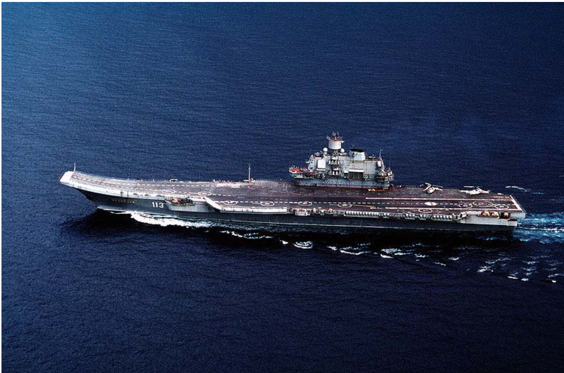
A view of the Russian Admiral Kuznetsov showing prominent ski-jump ramp
