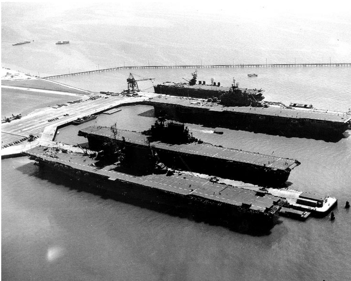
Four US Navy carriers right after the war, showing size and length differences: Saratoga (bottom), an early battlecruiser conversion; Enterprise (2nd from bottom), an early fleet carrier; Hornet (3rd from bottom), a war-time built Essex -class carrier; and San Jacinto (top), a light carrier based on a cruiser hull.
