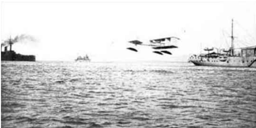
The first seaplane carrier, the French La Foudre (right, with hangar and crane), with one of her Canard Voisin seaplanes taking off, during tactical exercises in June 1912
