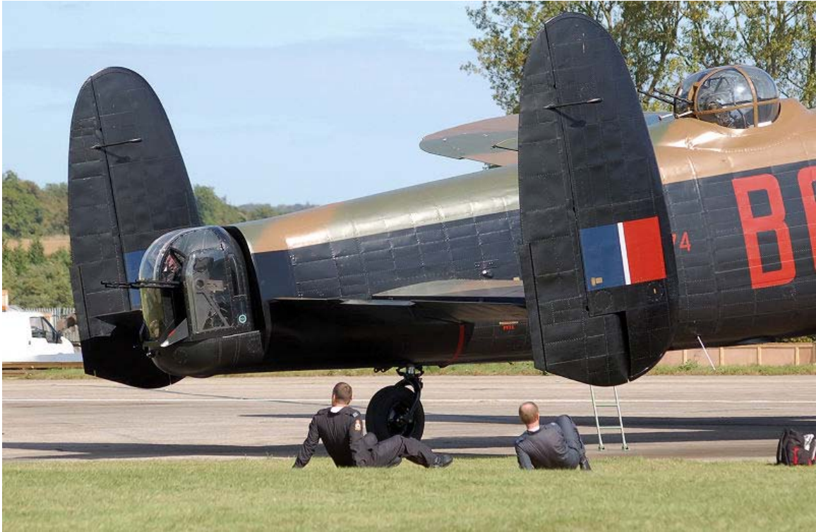
Tail and dorsal gun turrets of the Battle of Britain Memorial Flight Lancaster (PA474)
