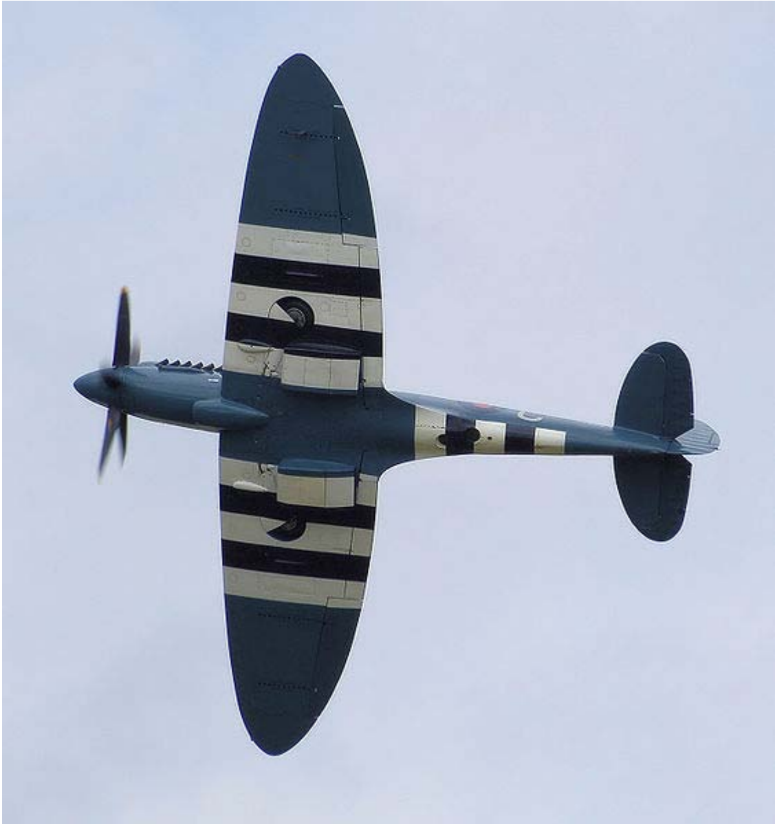
The elliptical planform of a Spitfire Mk XIX, seen at a British air show in 2008
