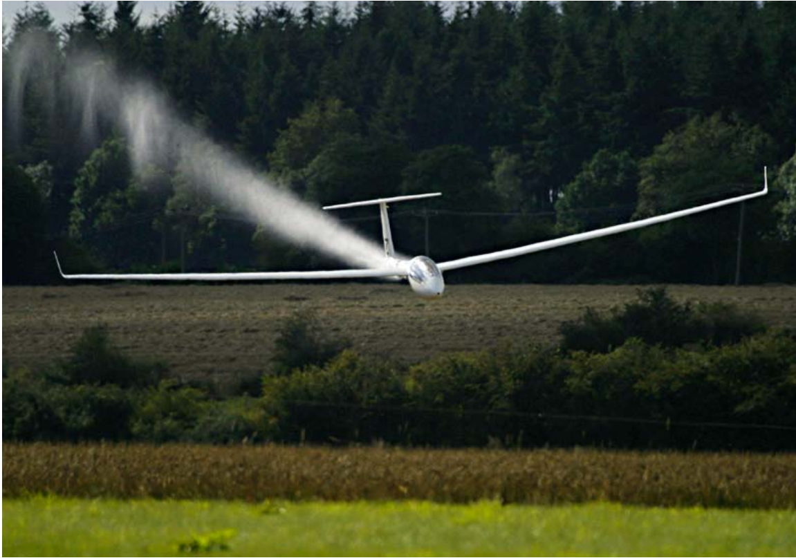
A glider releasing its water ballast
