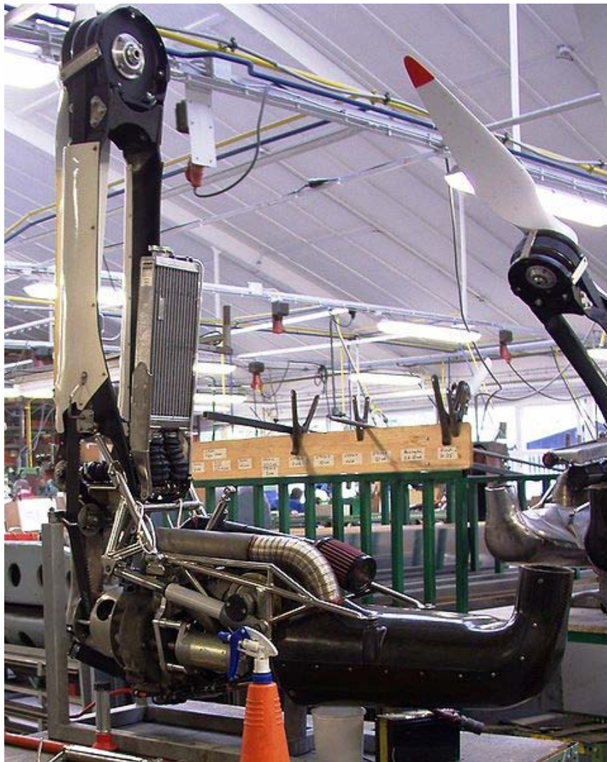
Powerplant from a Schleicher ASH 26e self-launching motor glider, mounted on a test stand for maintenance at the Alexander Schleicher GmbH & Co in Poppenhausen, Germany. Counter-clockwise from top left: propeller hub, mast with belt guide, radiator, Wankel engine, muffler shroud.
