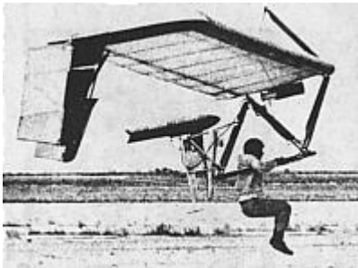
Icarus V hang glider powered with a G8-2 rocket engine, 1979.
