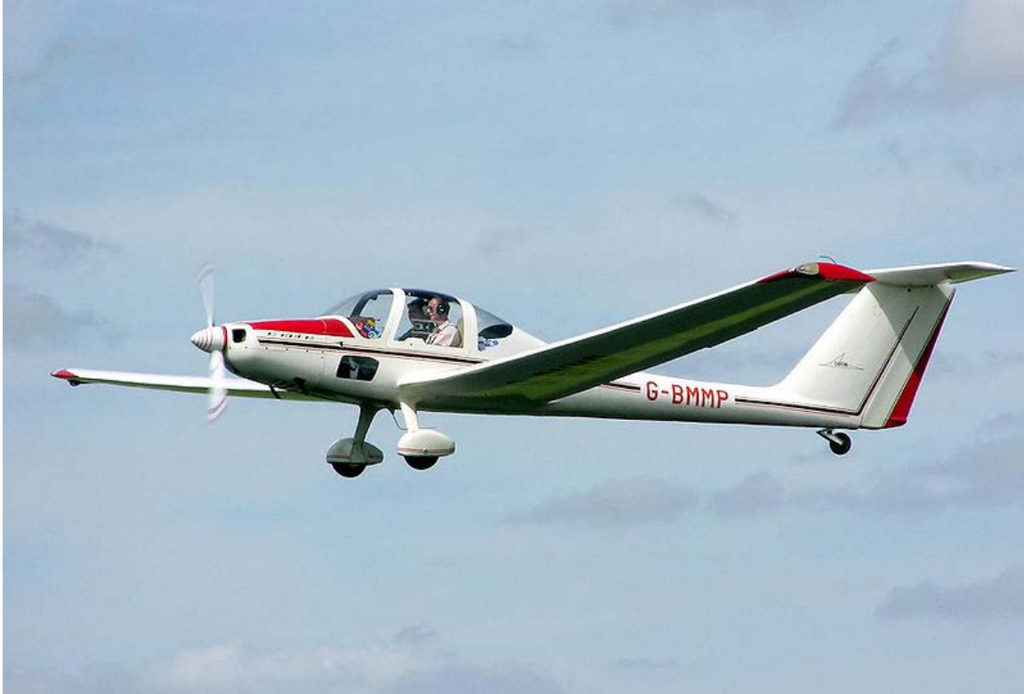
Grob G109B touring motor glider, with fibre-reinforced plastic construction.
