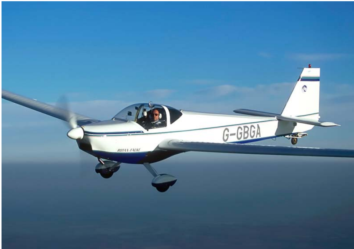
Scheibe SF25C - an older touring motorglider with tube and fabric fuselage construction.
