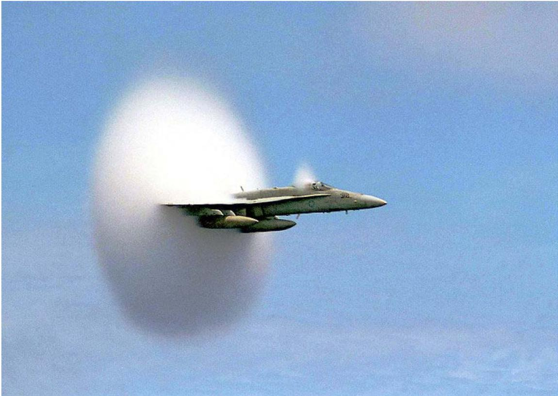
An F/A-18 Hornet at transonic speed and displaying the Prandtl–Glauert singularity just before reaching the speed of sound
