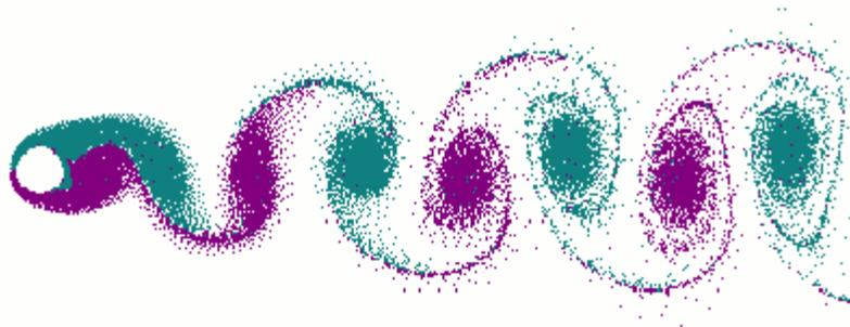
A vortex street around a cylinder. This occurs around cylinders, independently of the fluid, the cylinder size and the fluid speed, provided that there is a Reynolds number of between 250 and 200,000.
