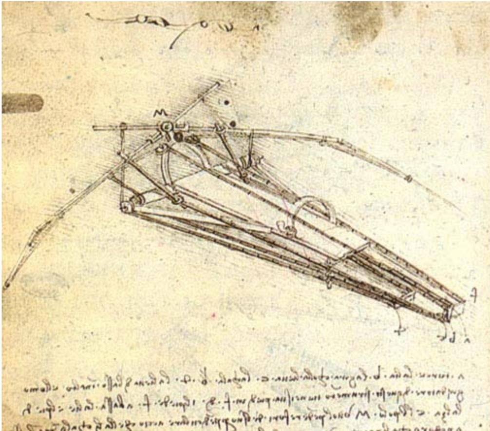
A drawing of a design for a flying machine by Leonardo da Vinci (c. 1488). This machine was an ornithopter, with flapping wings similar to a bird, first presented in his *Codex on the Flight of Birds* in 1505.
