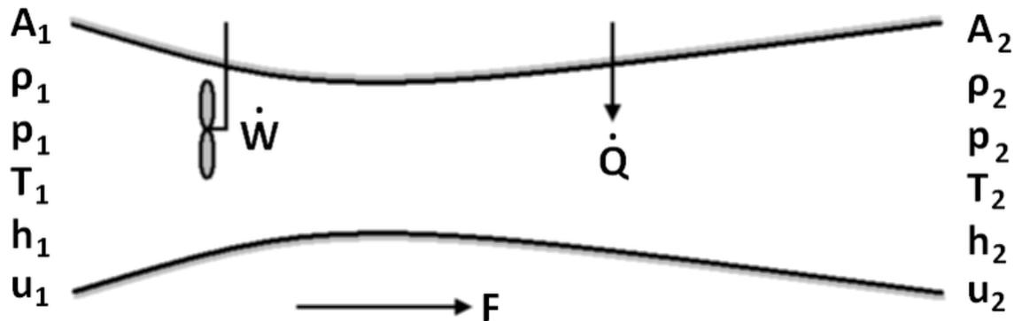
Control volume schematic of internal flow with one inlet and exit including an axial force, work, and heat transfer. State 1 is the inlet and state 2 is the exit.
