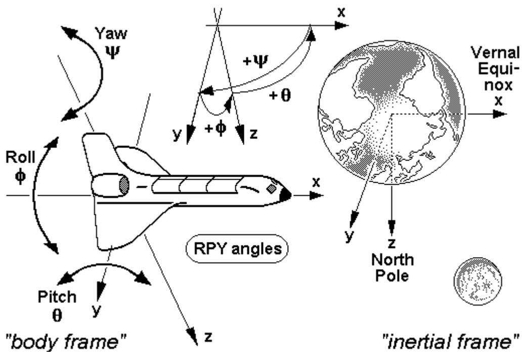
RPY angles of space shuttles and other space vehicles, first using a local frame as reference and second using an inertial frame as reference.
