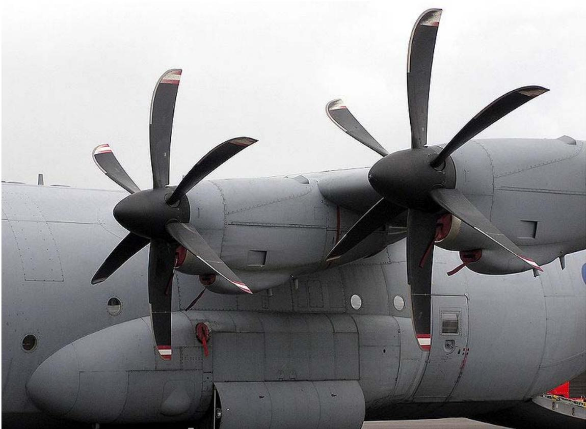
The feathered propellers of an RAF Hercules C.4
