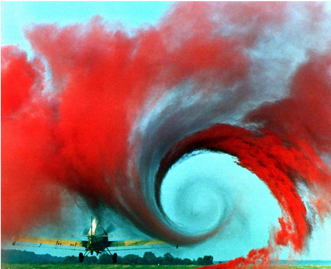
A vortex is created by the passage of an aircraft wing, revealed by smoke. Vortices are one of the many phenomena associated to the study of aerodynamics. The equations of aerodynamics show that the vortex is created by the difference in pressure between the upper and lower surface of the wing. At the end of the wing, the lower surface effectively tries to 'reach over' to the low pressure side, creating rotation and the vortex.
