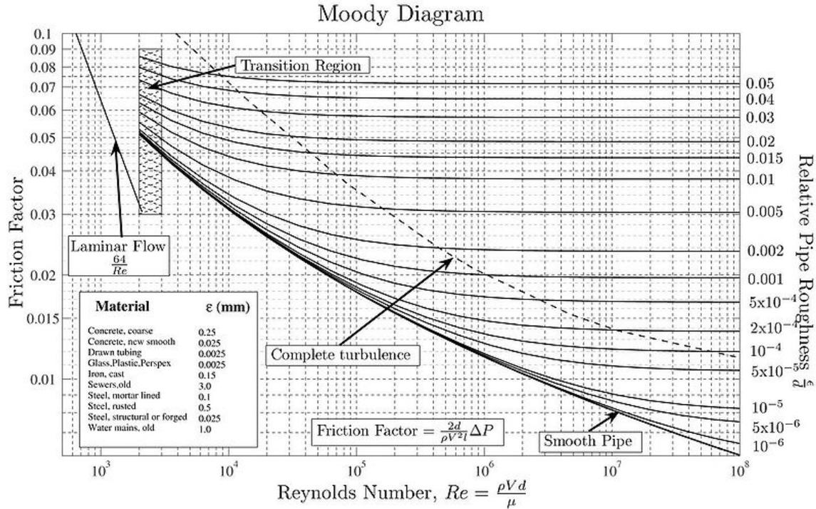
Pressure drops seen for fully-developed flow of fluids through pipes can be predicted using the Moody diagram which plots the Darcy–Weisbach friction factor  $f$  against Reynolds number  $Re$  and relative roughness  $\epsilon / D$ . The diagram clearly shows the laminar, transition, and turbulent flow regimes as Reynolds number increases. The nature of pipe flow is strongly dependent on whether the flow is laminar or turbulent
