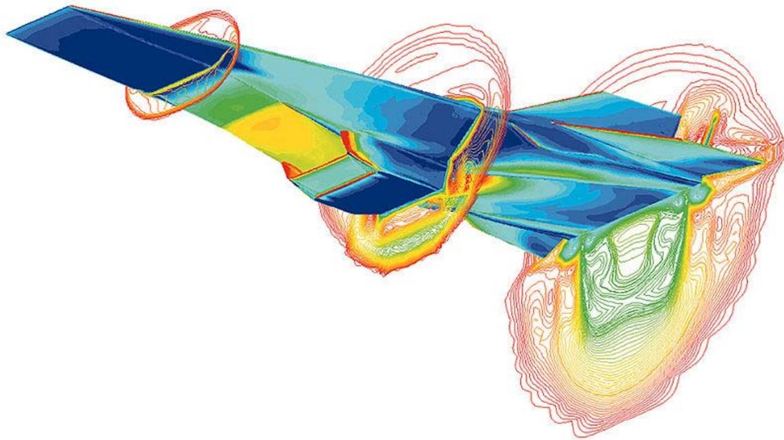
A computer generated model of NASA's X-43A hypersonic research vehicle flying at Mach 7 using a computational fluid dynamics code.
