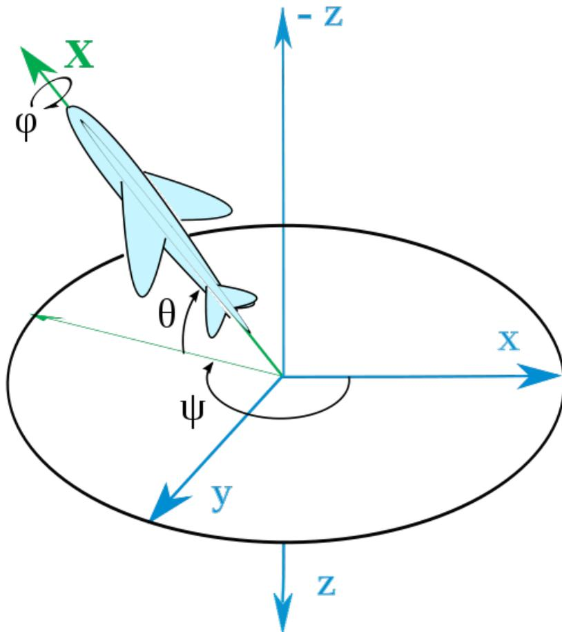
Heading, elevation and bank angles ( $Z$ - $Y'$ - $X''$ ) for an aircraft. The aircraft's pitch and yaw axes  $Y$  and  $Z$  are not shown, and its fixed reference frame  $xyz$  has been shifted backwards from its center of gravity (preserving angles) for clarity. Axes named according to the air norm DIN 9300
