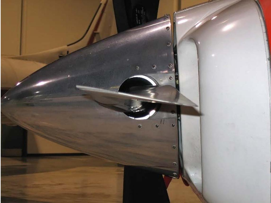
A propeller blade in feathered position
