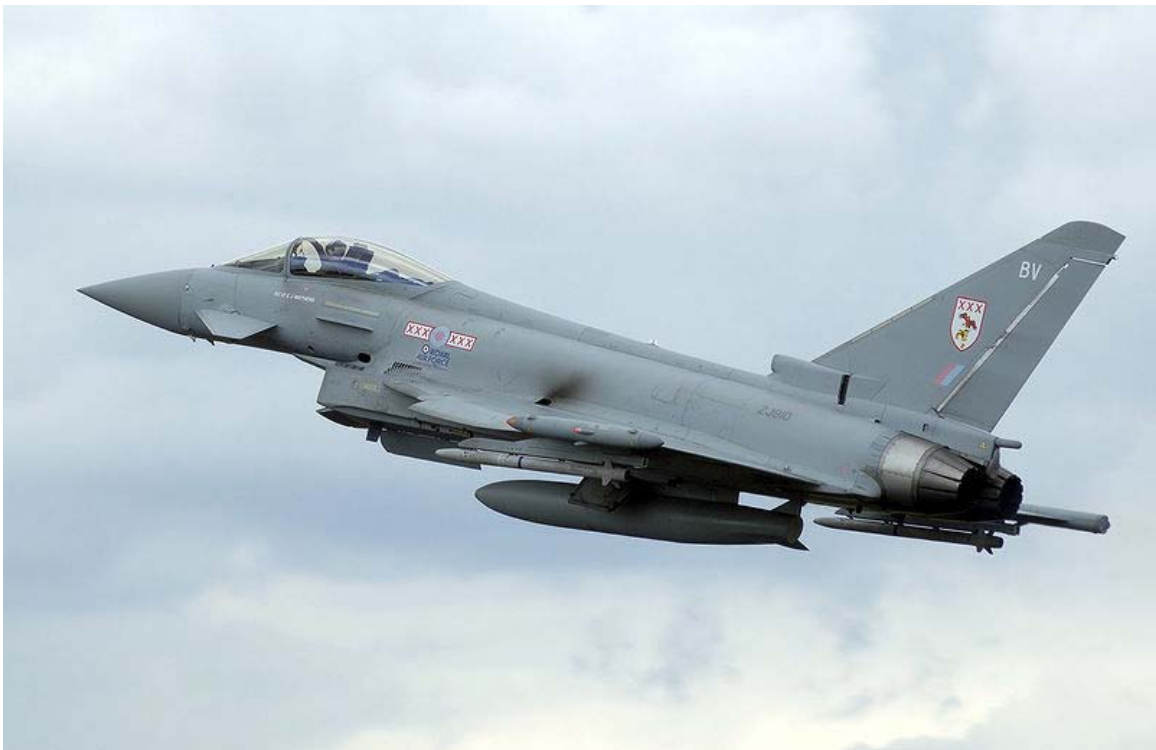
The Eurofighter Typhoon is capable of supercruise at Mach 1.5
