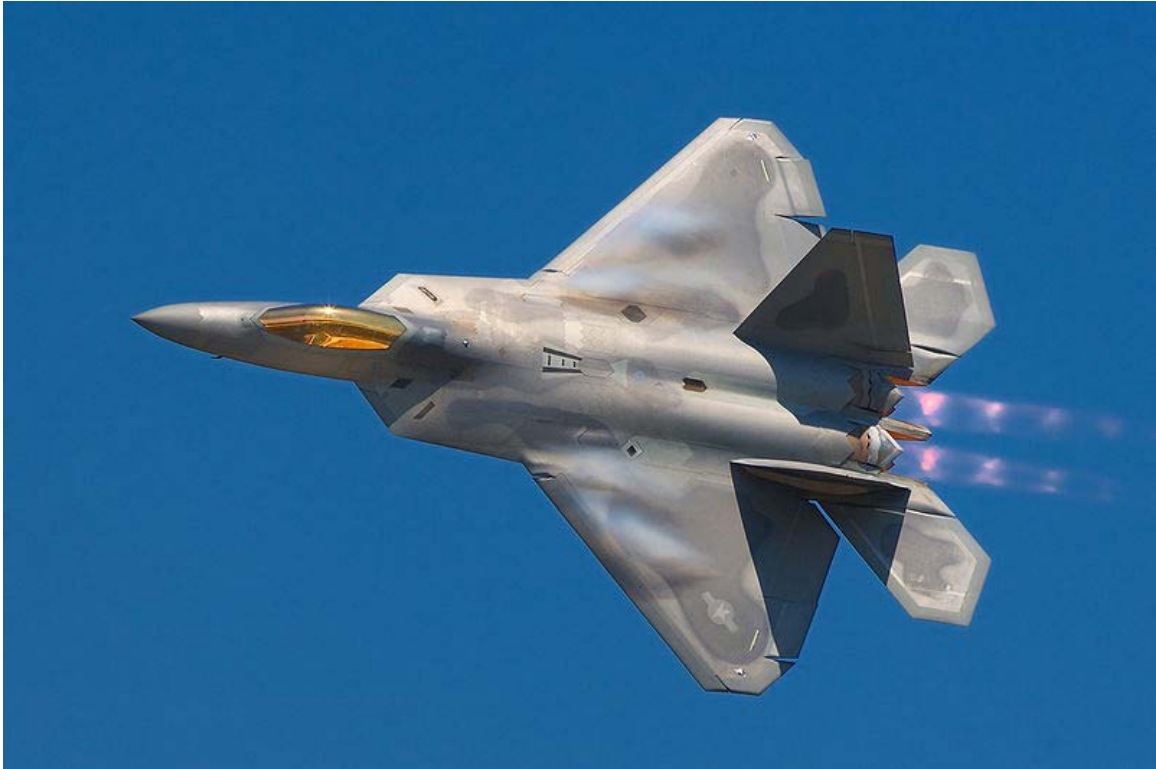
The F-22 Raptor is capable of supercruise (but is seen here running afterburner)
