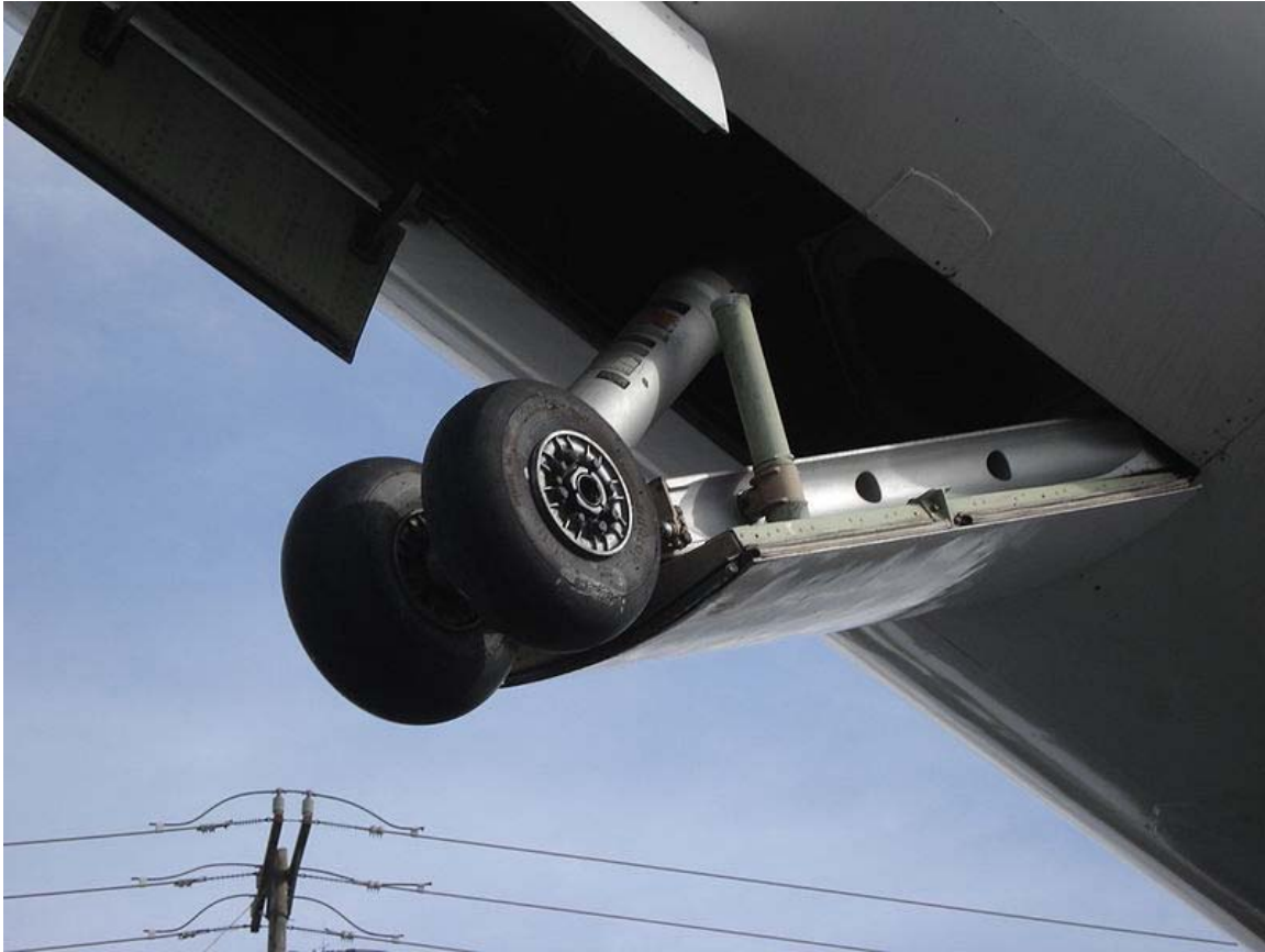
Tail bumper of Concorde G-BOAG at the Museum of Flight in Seattle
