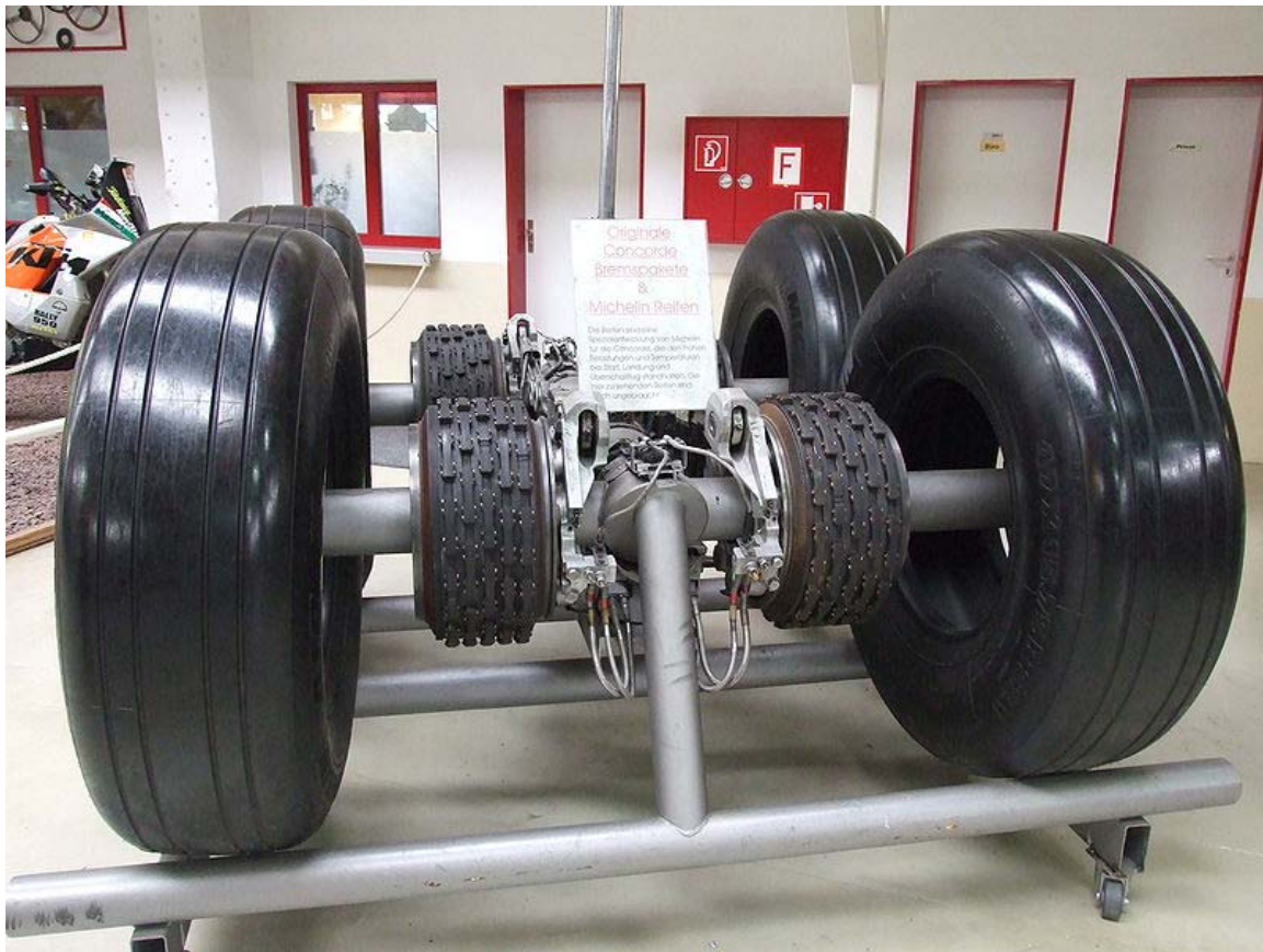
Concorde tyres and brakes
