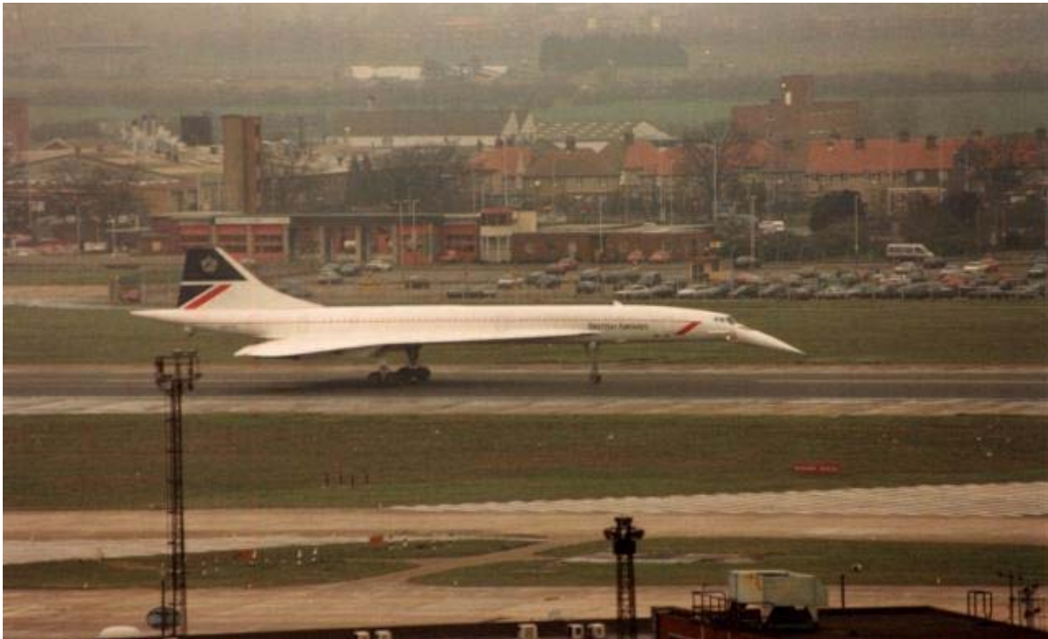
Concorde with droop nose in fully down position during rollout after landing
