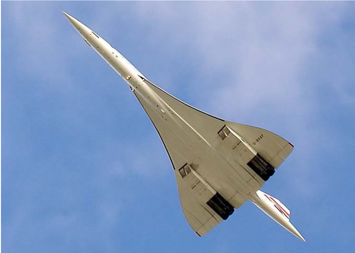
Concorde's final flight, G-BOAF from Heathrow to Bristol, on 26 November 2003. The extremely high fineness ratio of the fuselage is evident.
