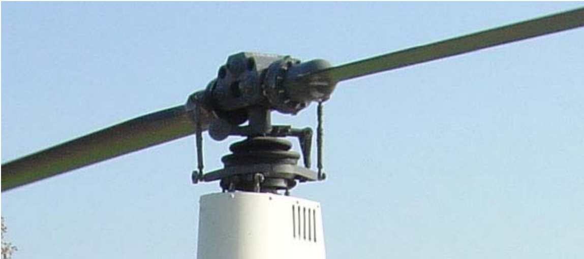
The simple rotor of a Robinson R22
