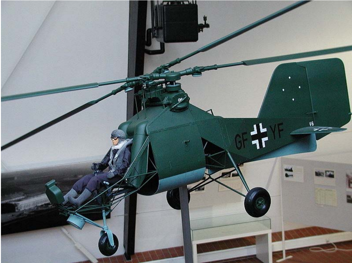
Flettner Fl 282 "Kolibri" was an early ancestor of helicopters with intermeshing rotors.
