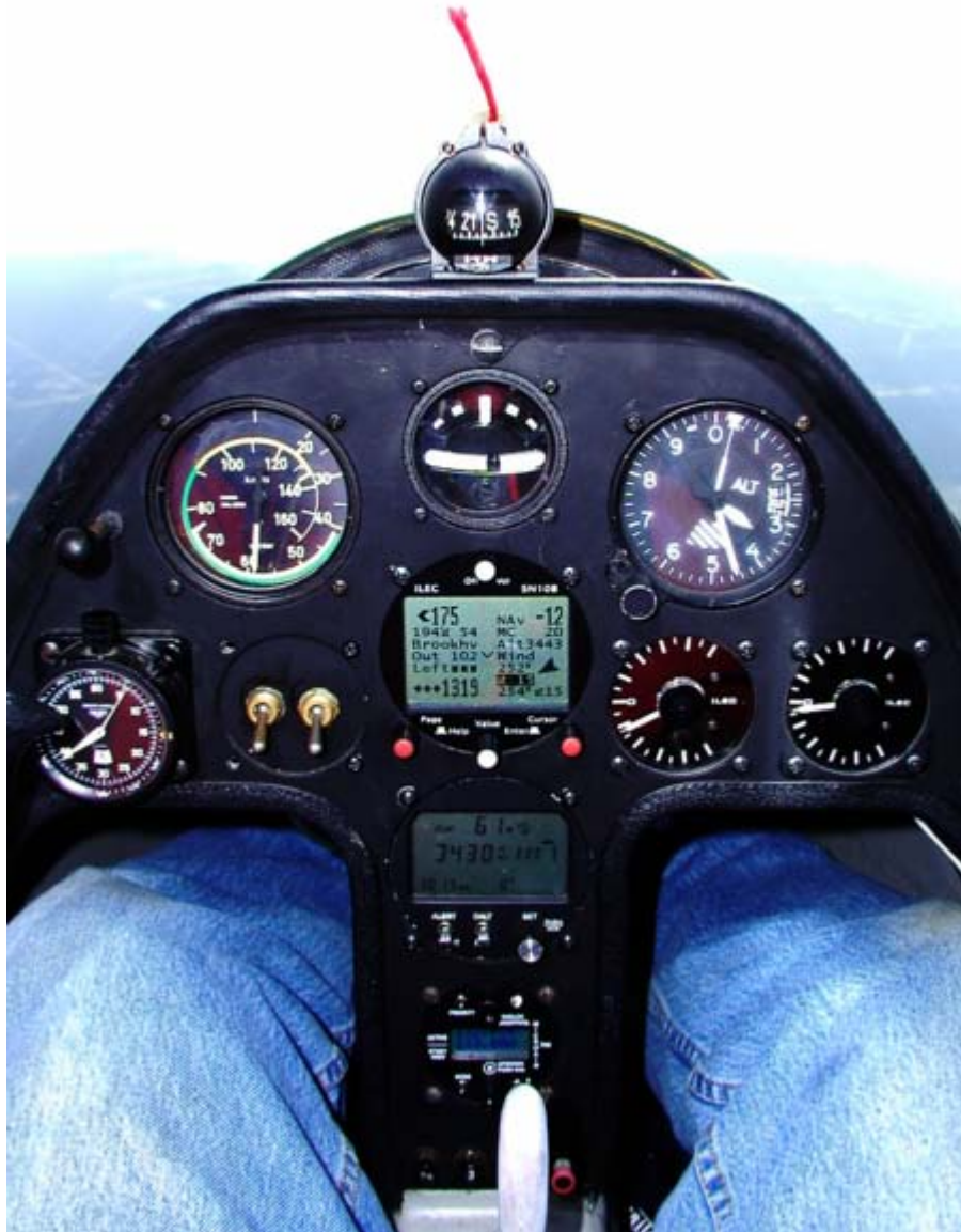
Schempp-Hirth Janus-C glider Instrument panel equipped for "cloud flying". The turn and bank indicator is top center. The heading indicator is replaced by a GPS-driven computer with wind and glide data, driving two electronic variometer displays to the right.
