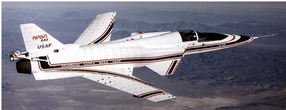
Grumman X-29, an experimental aircraft for forward swept wing research
