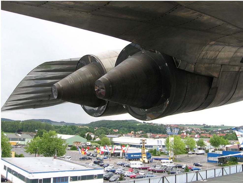
Engines RD-36-51A of a Tu-144D
