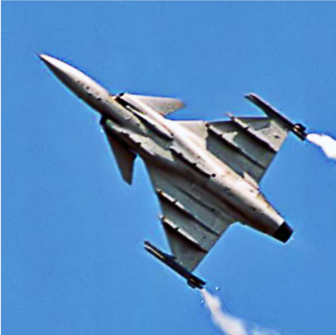
Canards visible on a JAS 39 Gripen at the Farnborough Airshow
