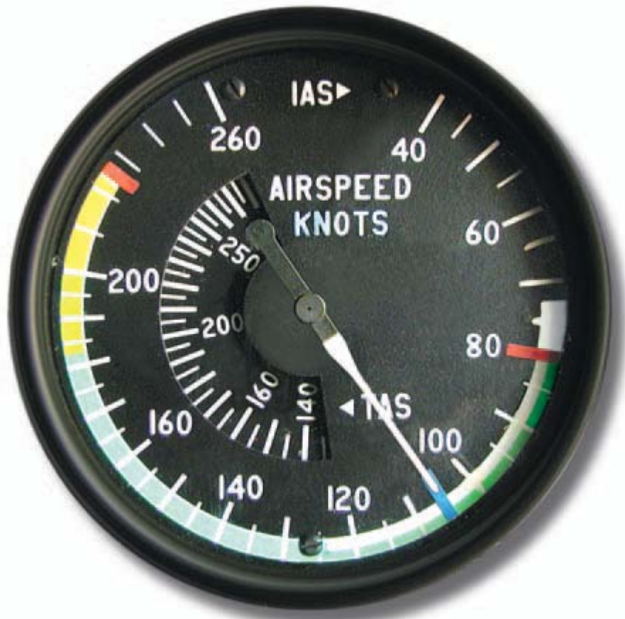
Airspeed indicator markings for a light multiengine airplane.
