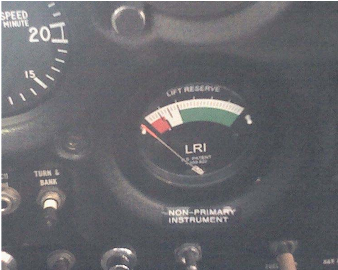
Lift Reserve Indicator as installed
