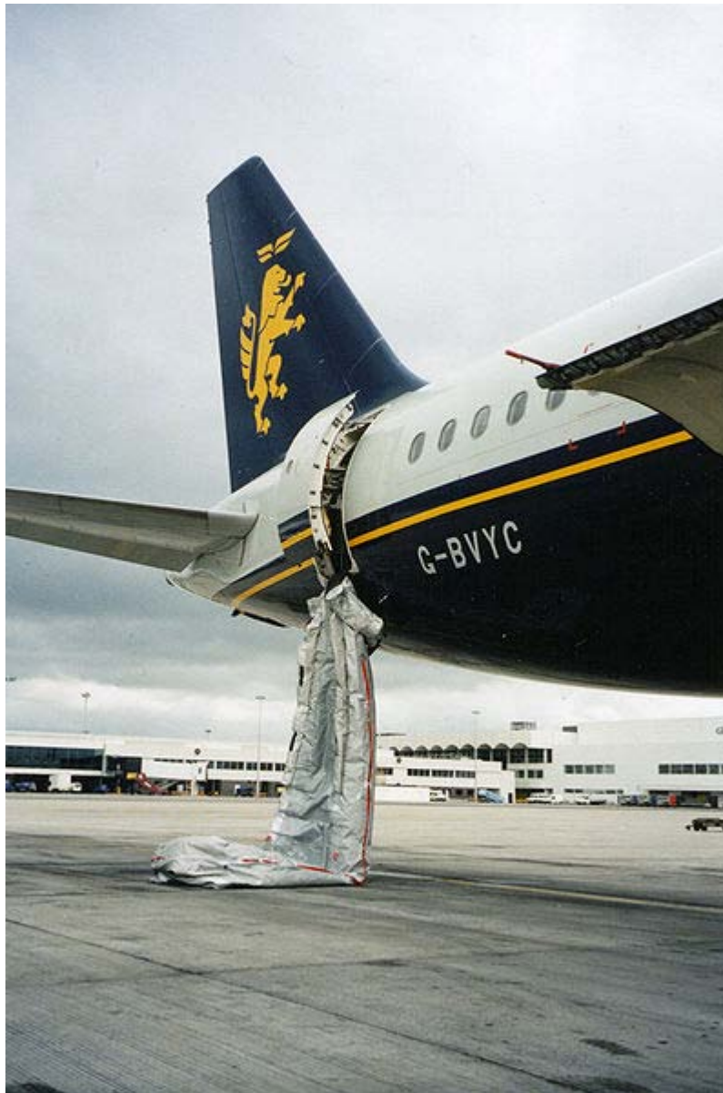
Deflated evacuation slide on an Airbus A320.
