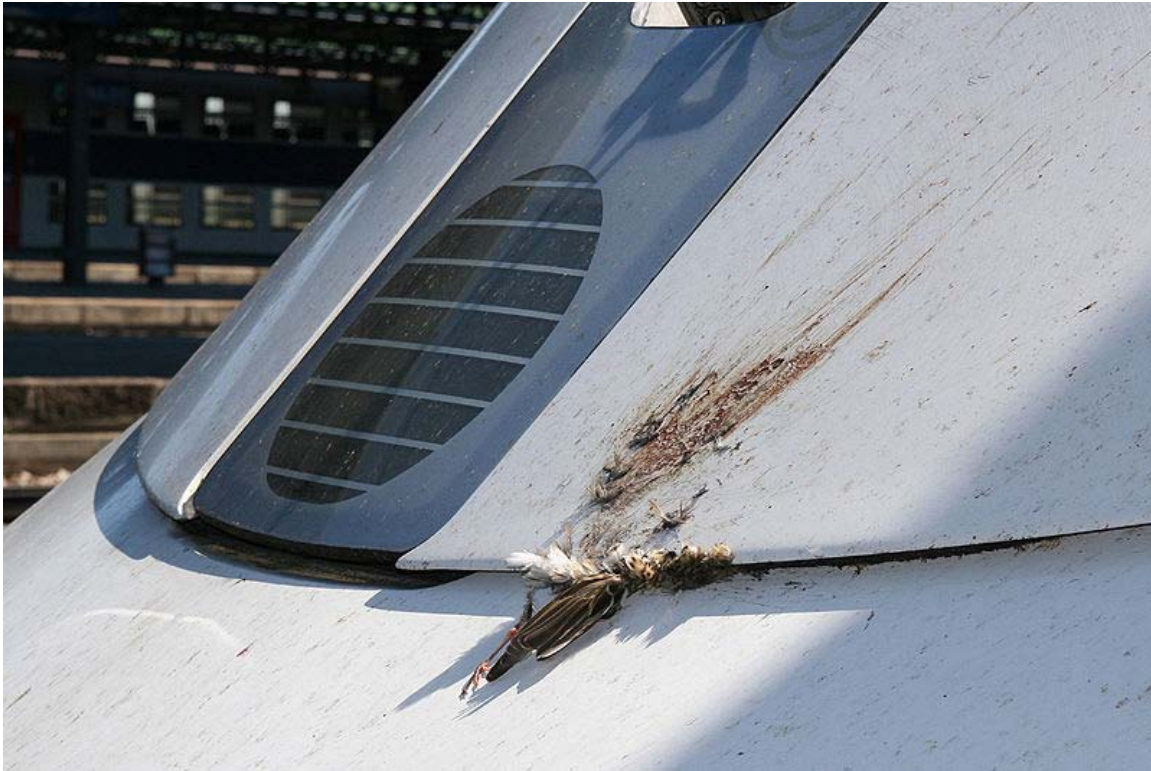
A ICE 3 high speed train after hitting a bird
