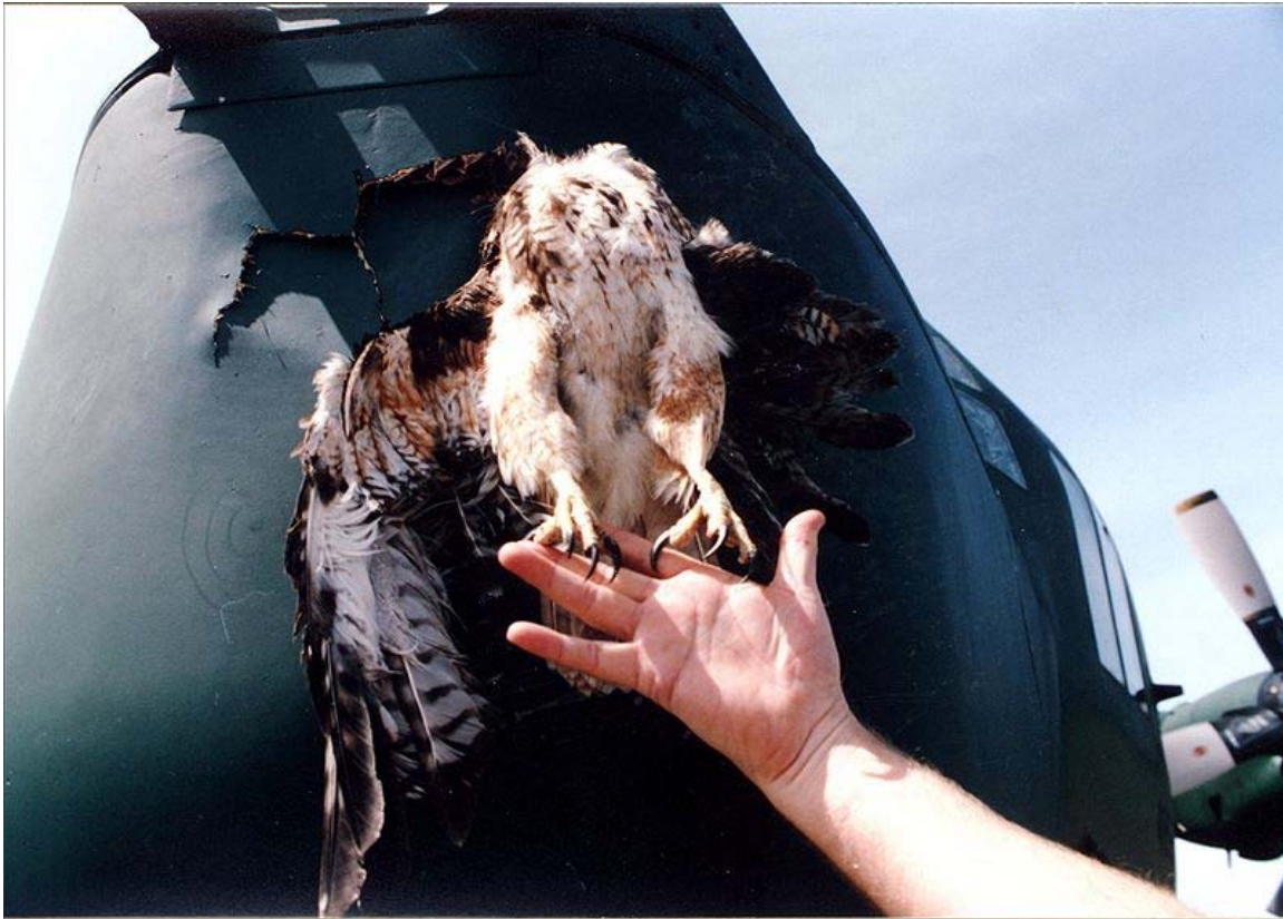
A hawk stuck in the nosecone of a C-130
