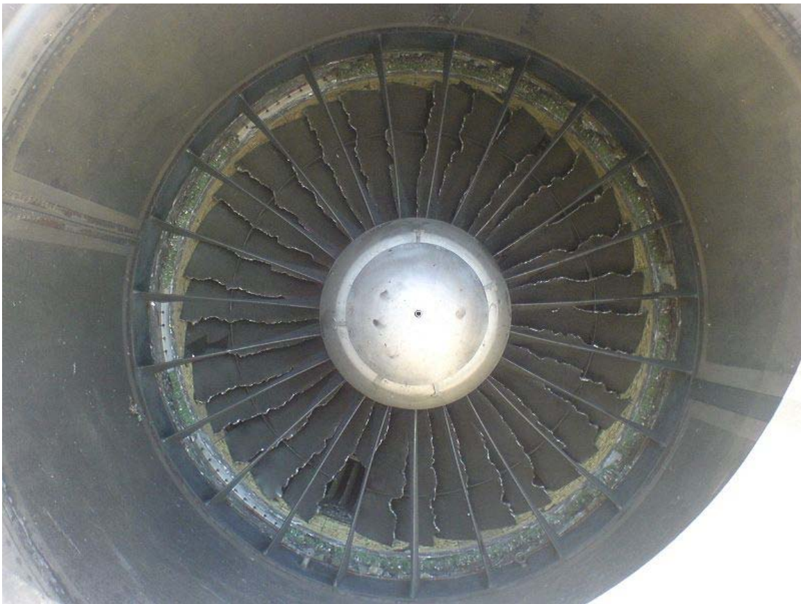
View of fan blades of JT8D Jet engine after a bird strike.
