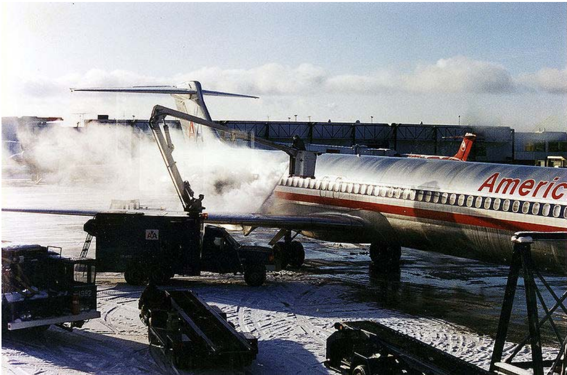
An American Airlines MD-80 aircraft being de-iced at Syracuse Hancock International Airport.
