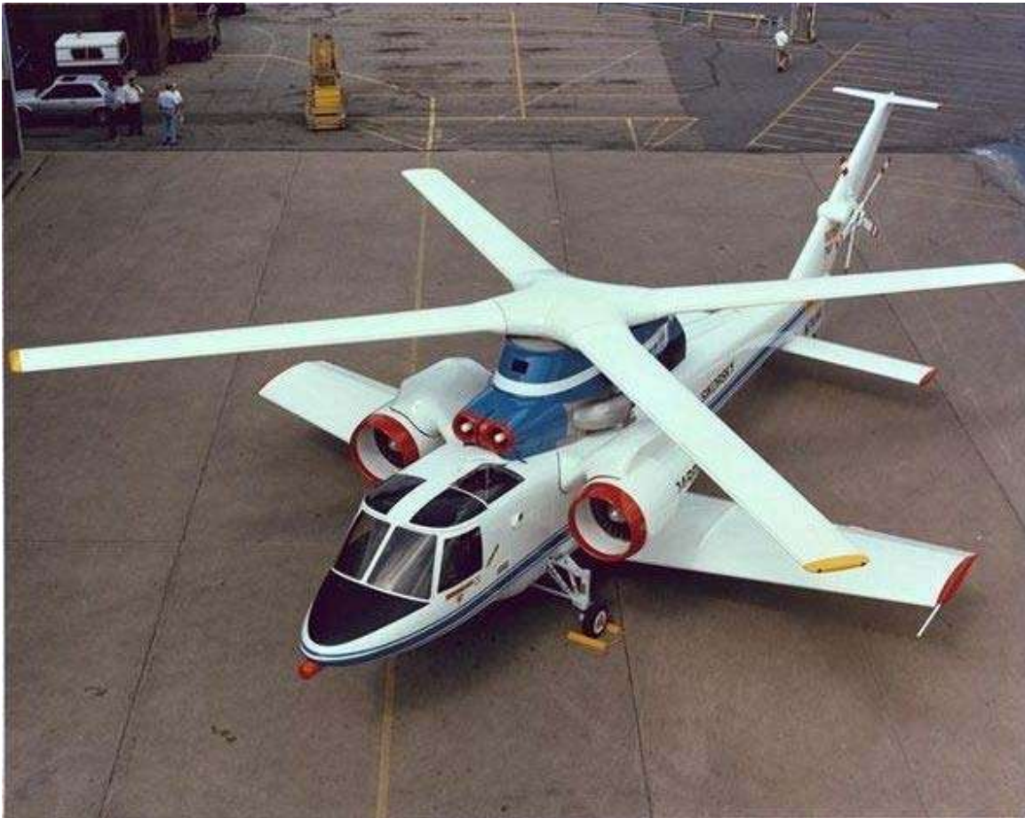
Sikorsky S-72 modified as the X-Wing testbed
