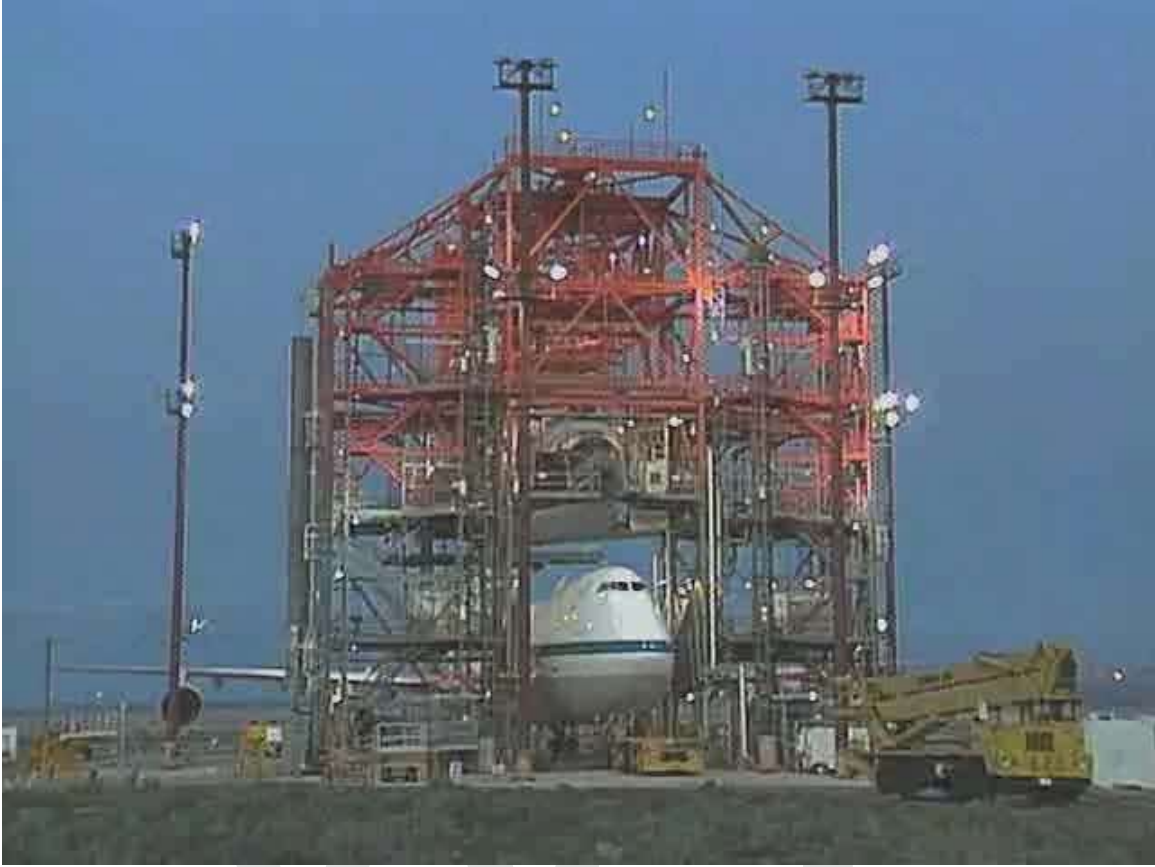
SCA mating with Endeavour in the Mate-Demate Device (MDD), April, 1994
