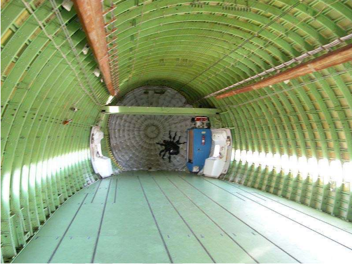
Aft end of the interior. Note the large stuffed spider mounted on the aft pressure bulkhead.
