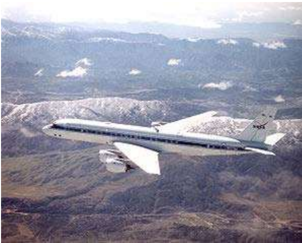
NASA Dryden DC-8 airborne laboratory refitted with CFM56 turbofan engines
