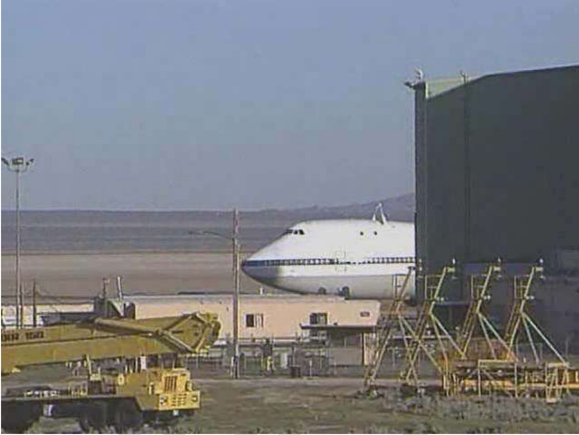
SCA approaching Endeavour suspended in the Mate-Demate Device (MDD), April, 1994
