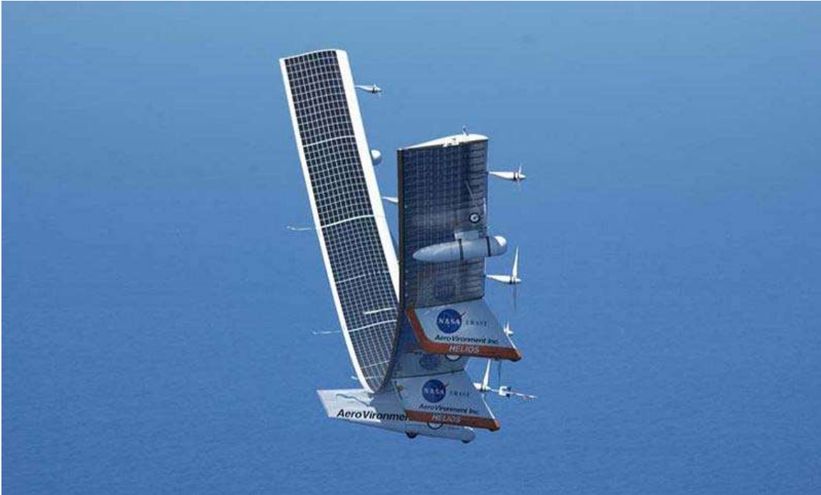
Helios with very high wing dihedral just before breaking up
