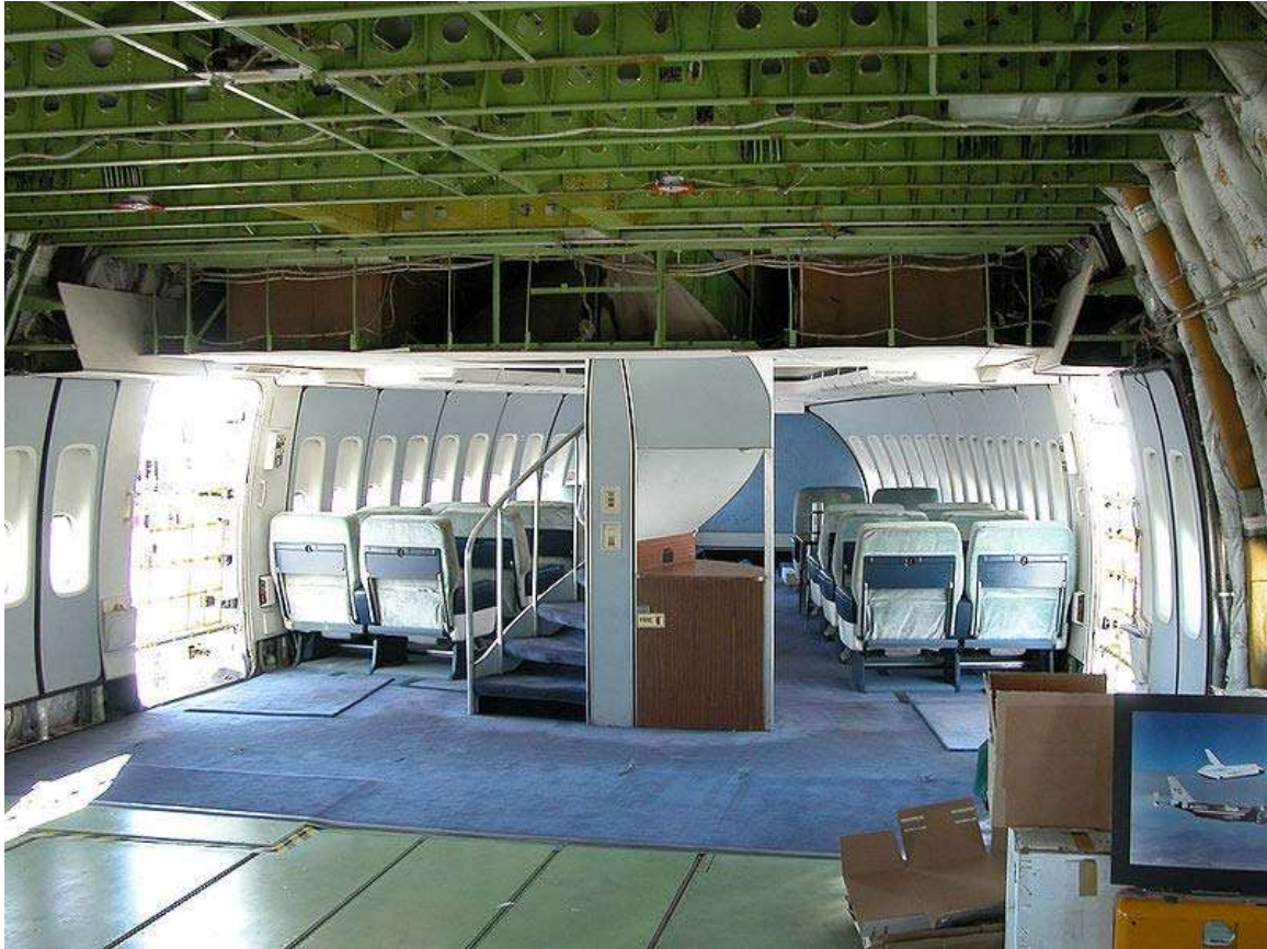
The first class section in the nose of N905NA. This is the only area on the main deck that has not been stripped to the bare metal
