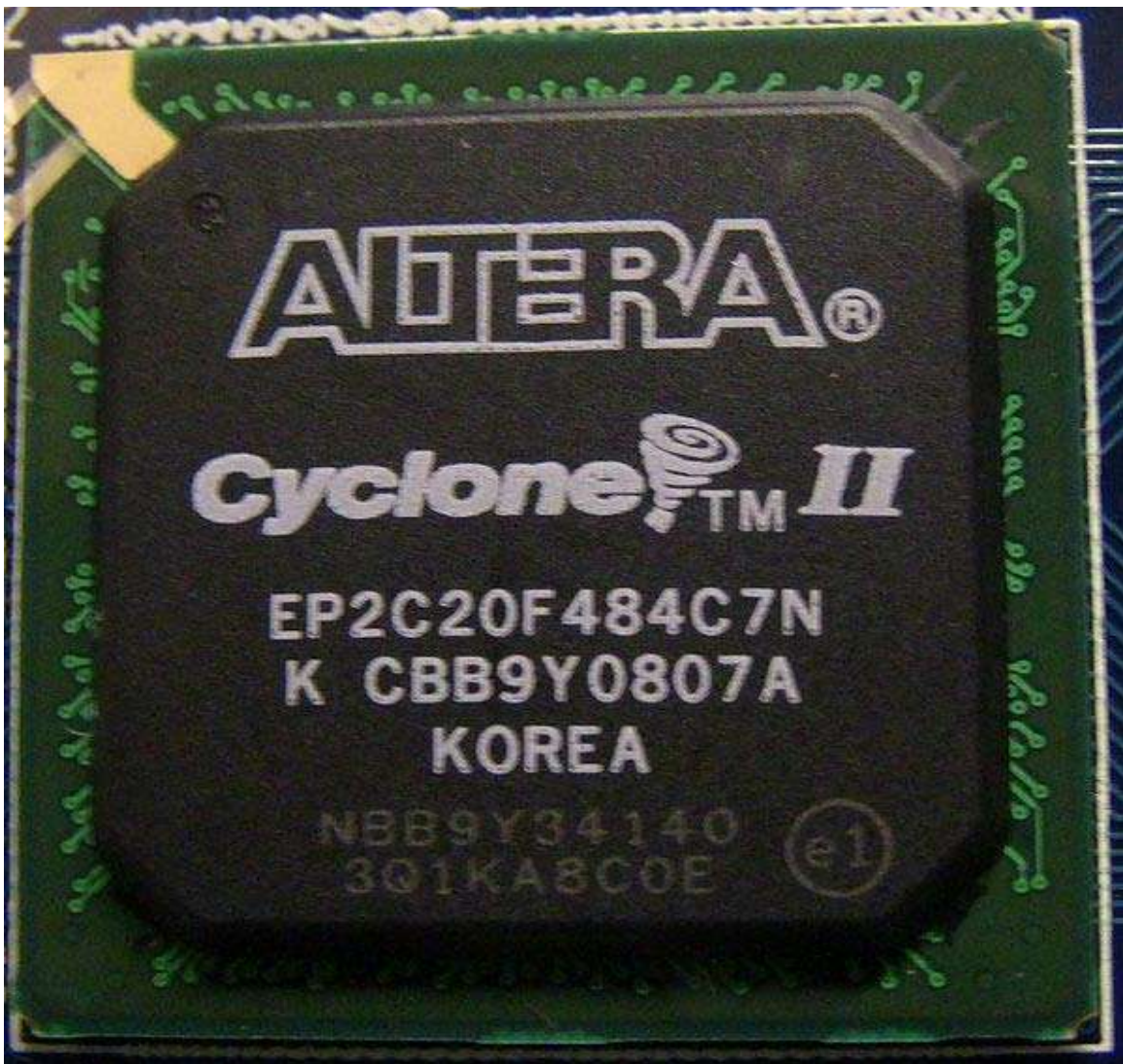
An Altera Cyclone II FPGA, on an Altera teraSIC DE1 Prototyping board
