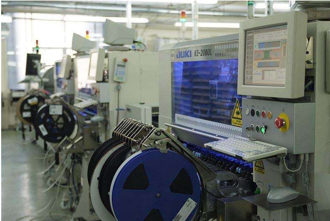
Assembly line of SMT placement machines
