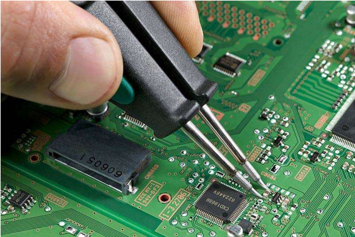
Tweezer soldering iron used on '0805' SMD component
