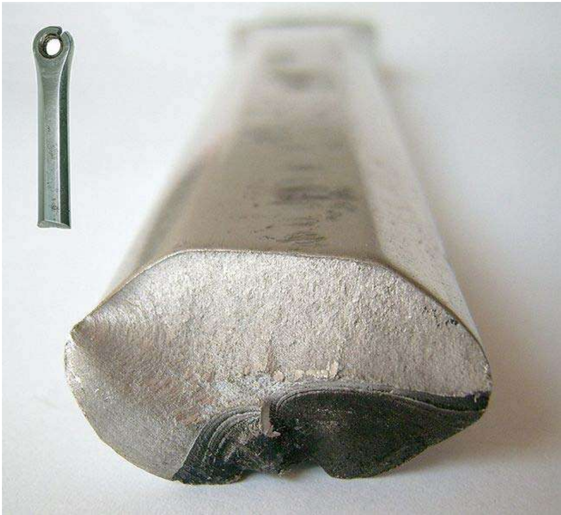
Fracture of an aluminium crank arm. Dark area of striations: slow crack growth. Bright granular area: sudden fracture.
