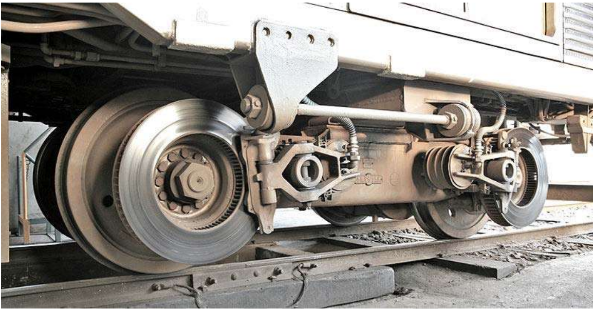
A railroad bogie and disc brakes
