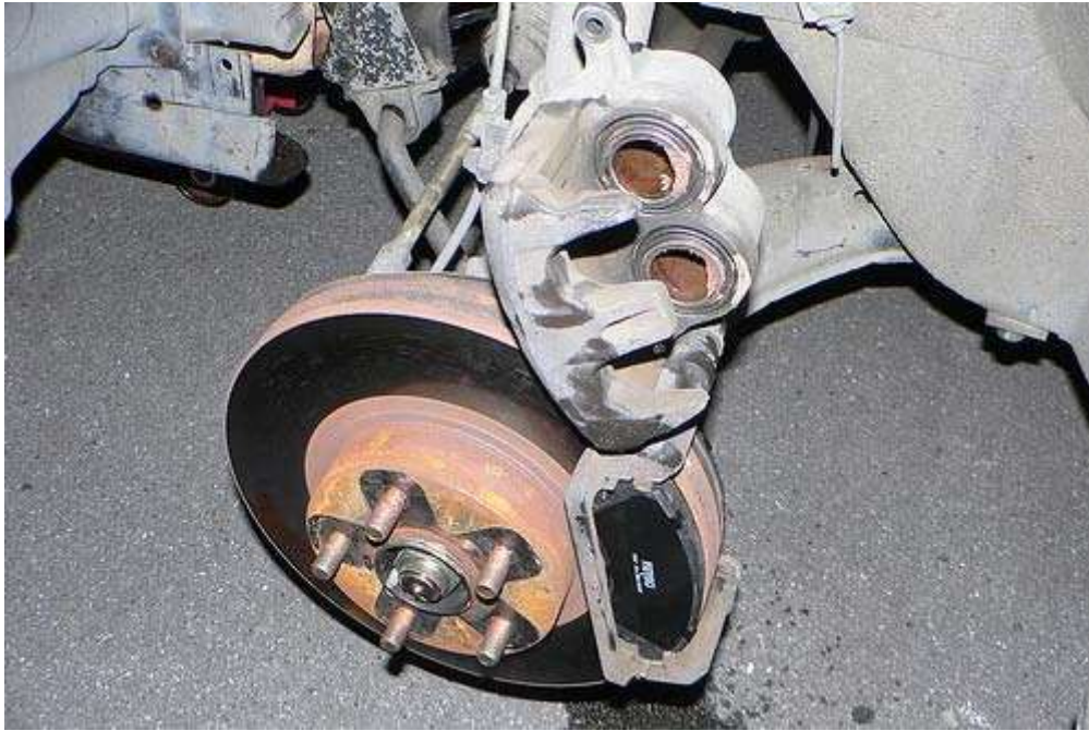
Disc brake caliper (twin-pot, floating) removed from brake pad for changing pads
