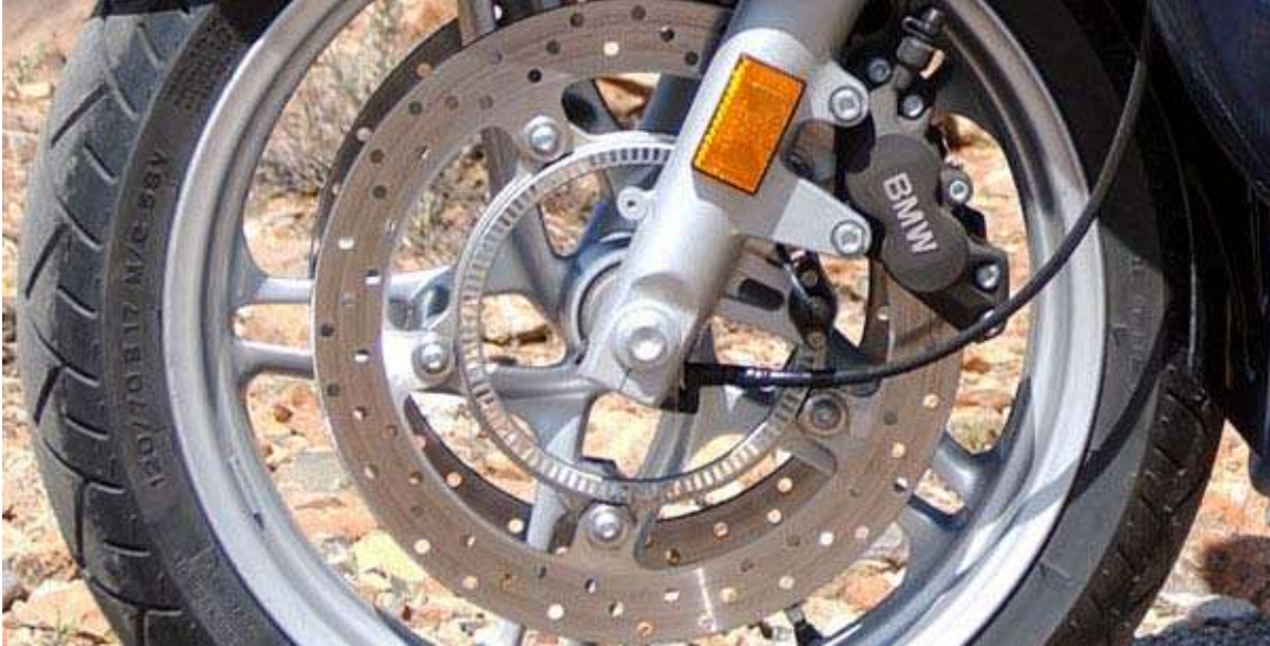
ABS brakes on a BMW motorcycle
