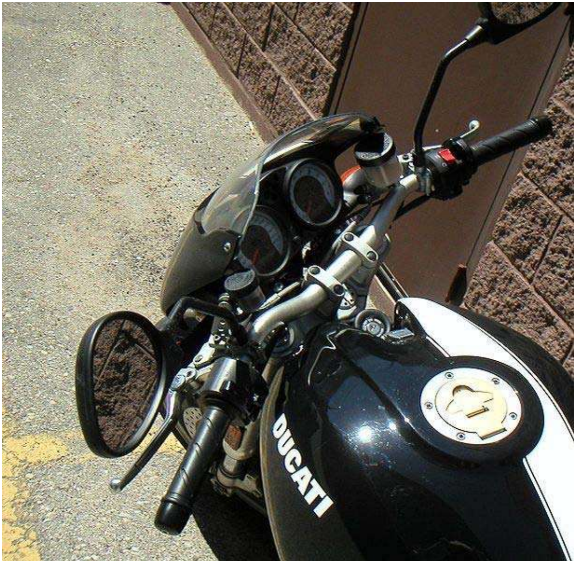
One-piece handlebars on a Ducati bolted to the triple tree with a short riser
