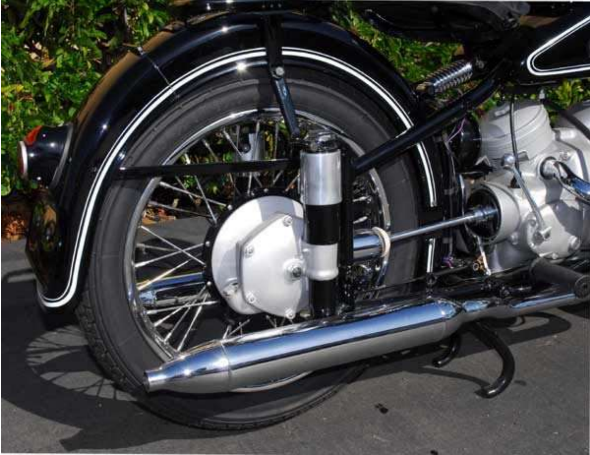
Plunger suspension on a 1953 BMW R51/3
