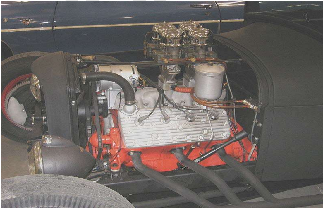
"Rat rodded" Deuce coupe with Edelbrock head and chrome carb hats on late-model flatty.
