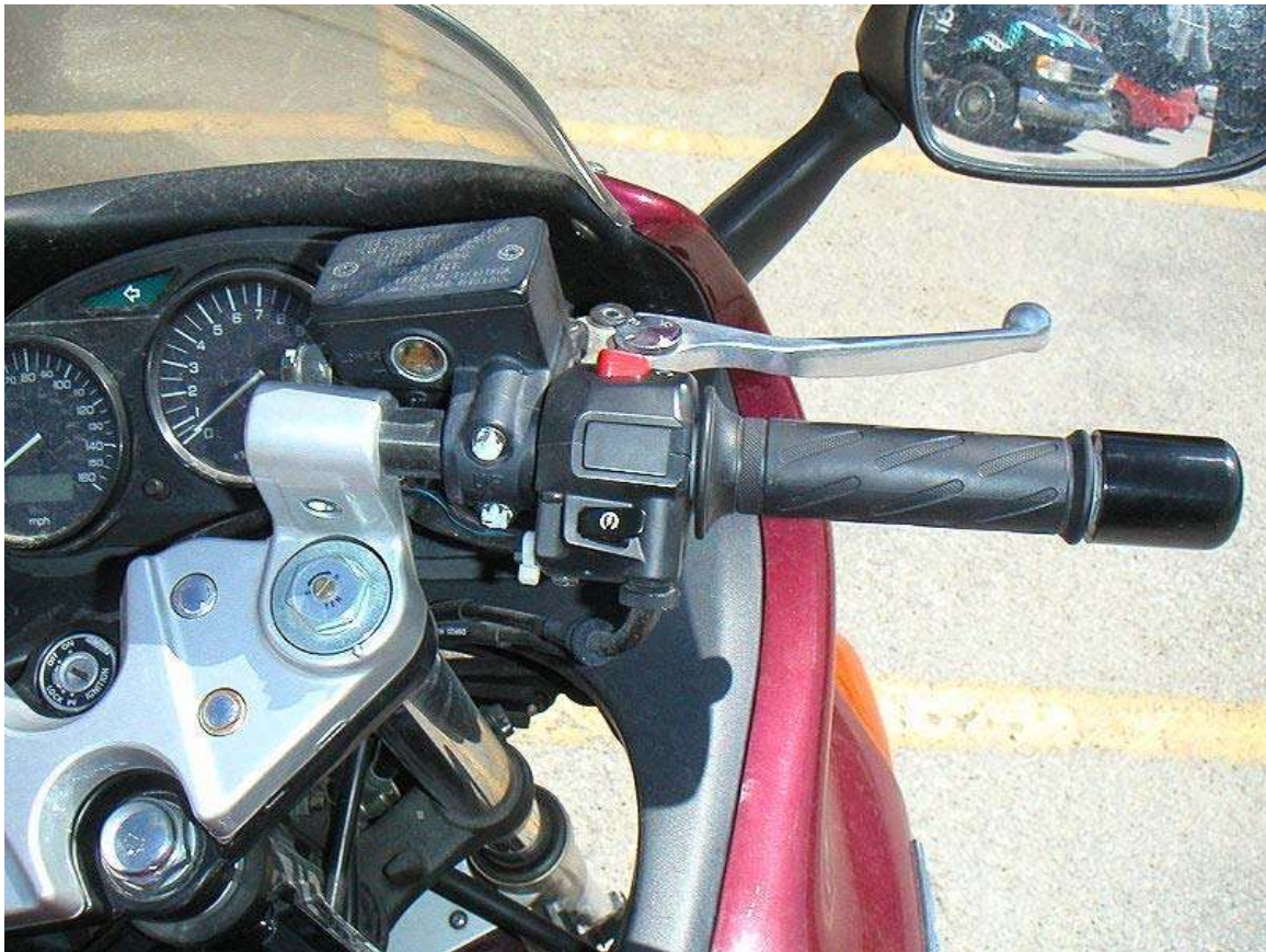
A right clip-on handlebar with twist throttle control, brake lever, and ignition switches
