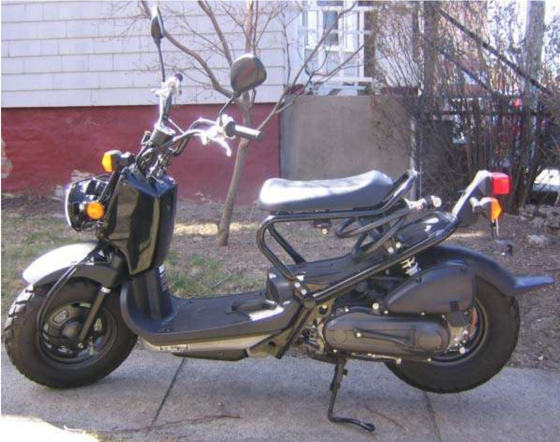
The Honda Ruckus uses a skeleton-style frame without body paneling
