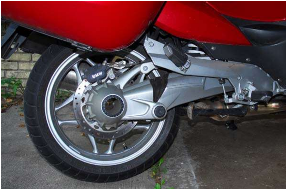
BMW's Paralever rear suspension on an R1200RT
