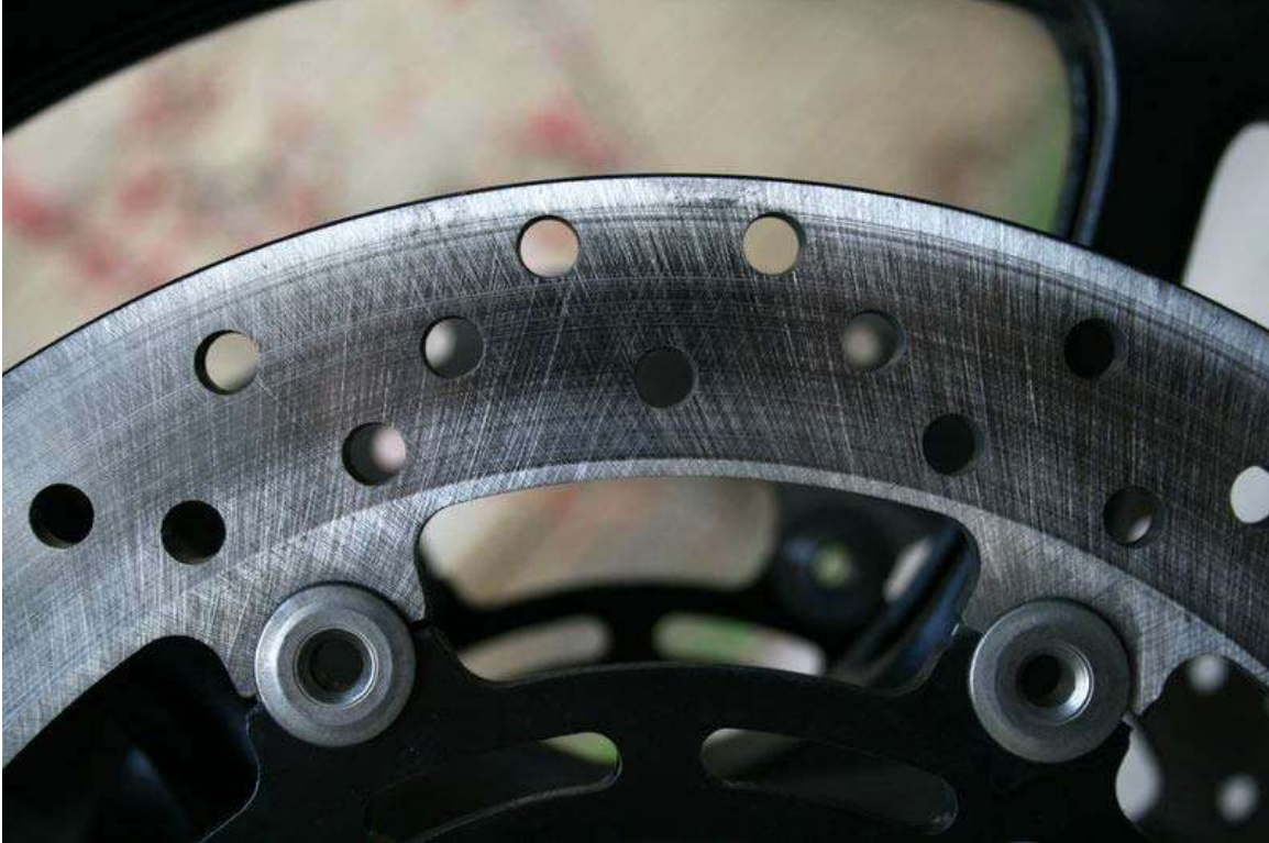
A cross-drilled disc on a modern motorcycle
