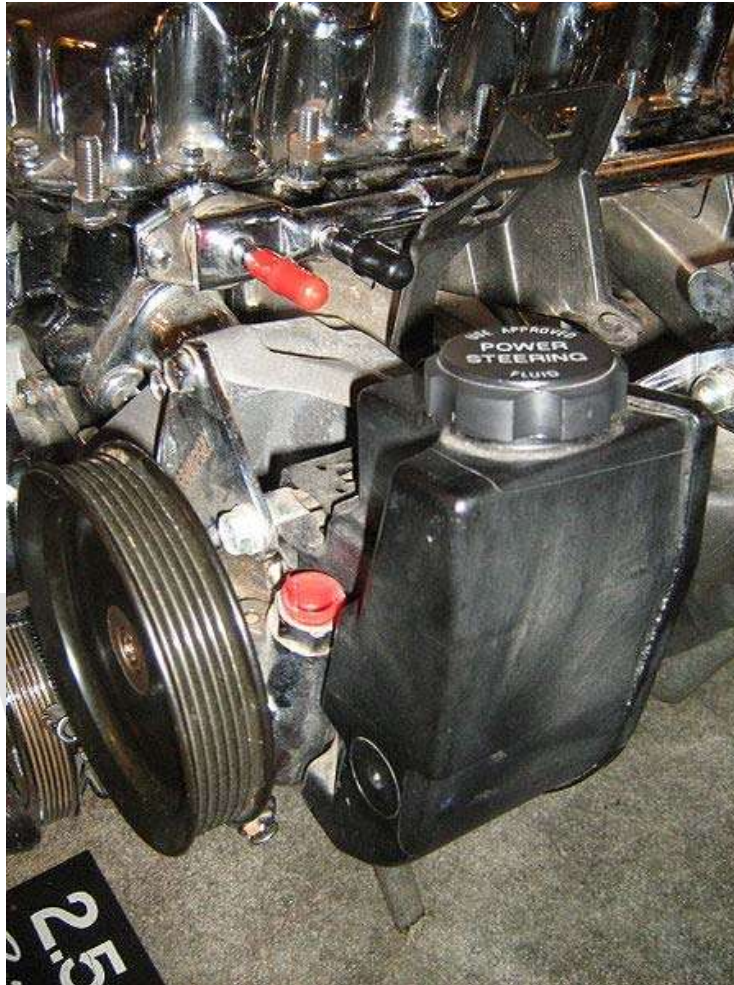
A power steering fluid reservoir and pulley driven pump
