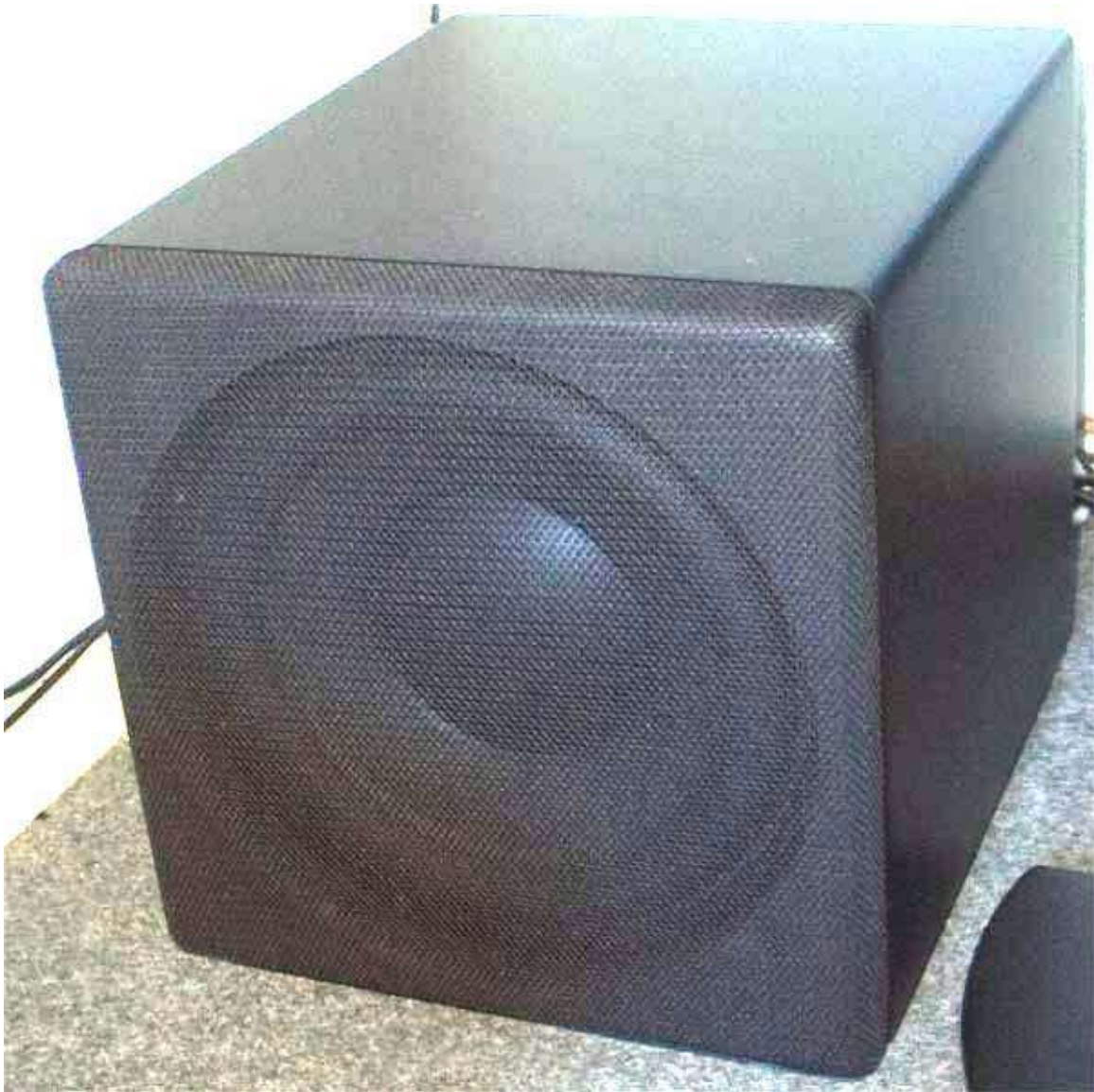
Subwoofer mounted in a sealed enclosure
