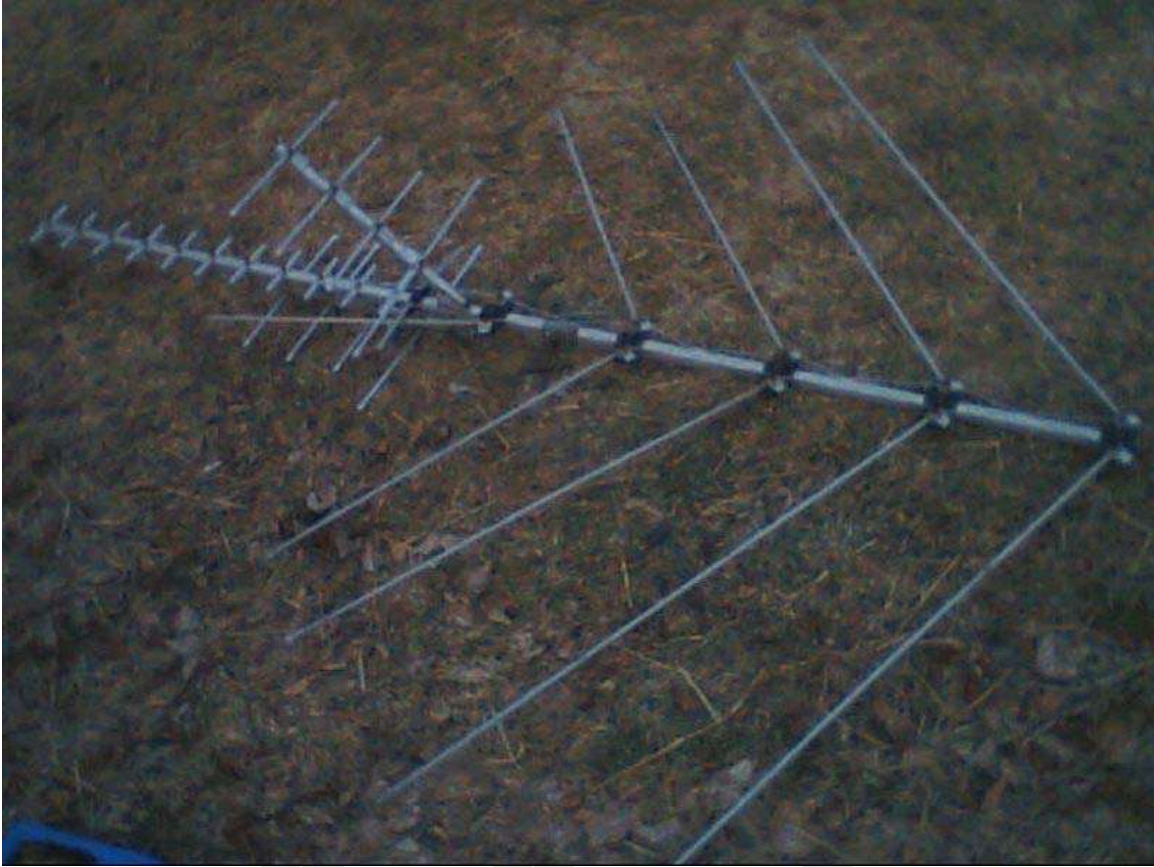
Typical US multiband TV antenna (aerial)
