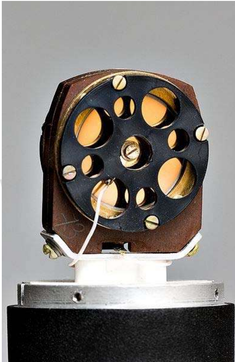
Inside the Oktava 319 condenser microphone
