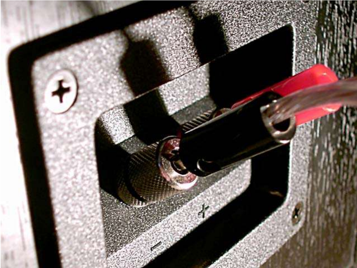
Two-way binding posts on a loudspeaker, connected using banana plugs
