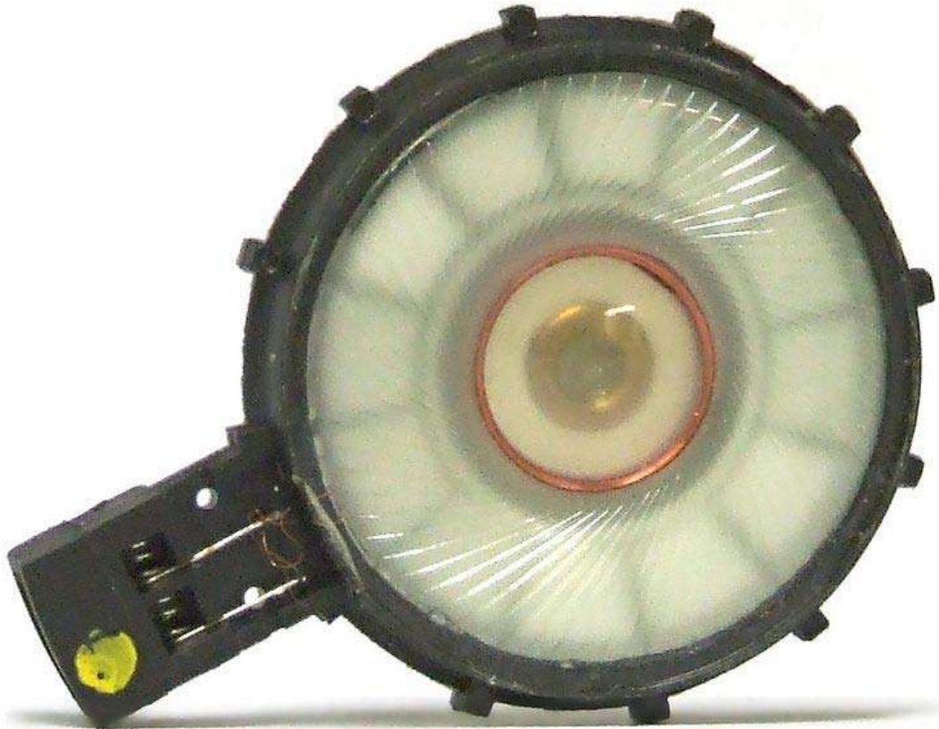
A typical moving-coil headphone transducer
