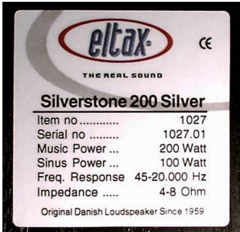
Specifications label on a loudspeaker
