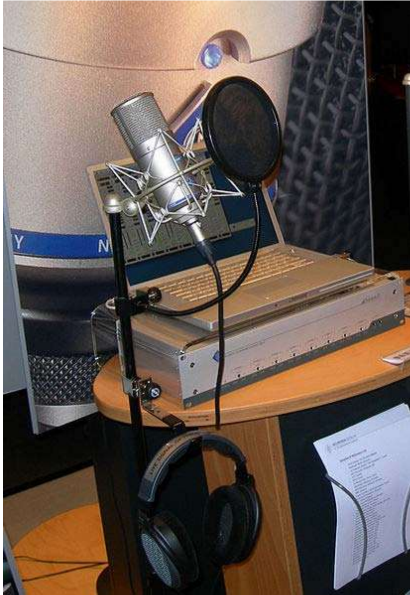
Neumann D-01 digital microphone and Neumann DMI-8 8-channel USB Digital Microphone Interface
