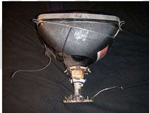
A common CRT used in computer monitors and television sets
