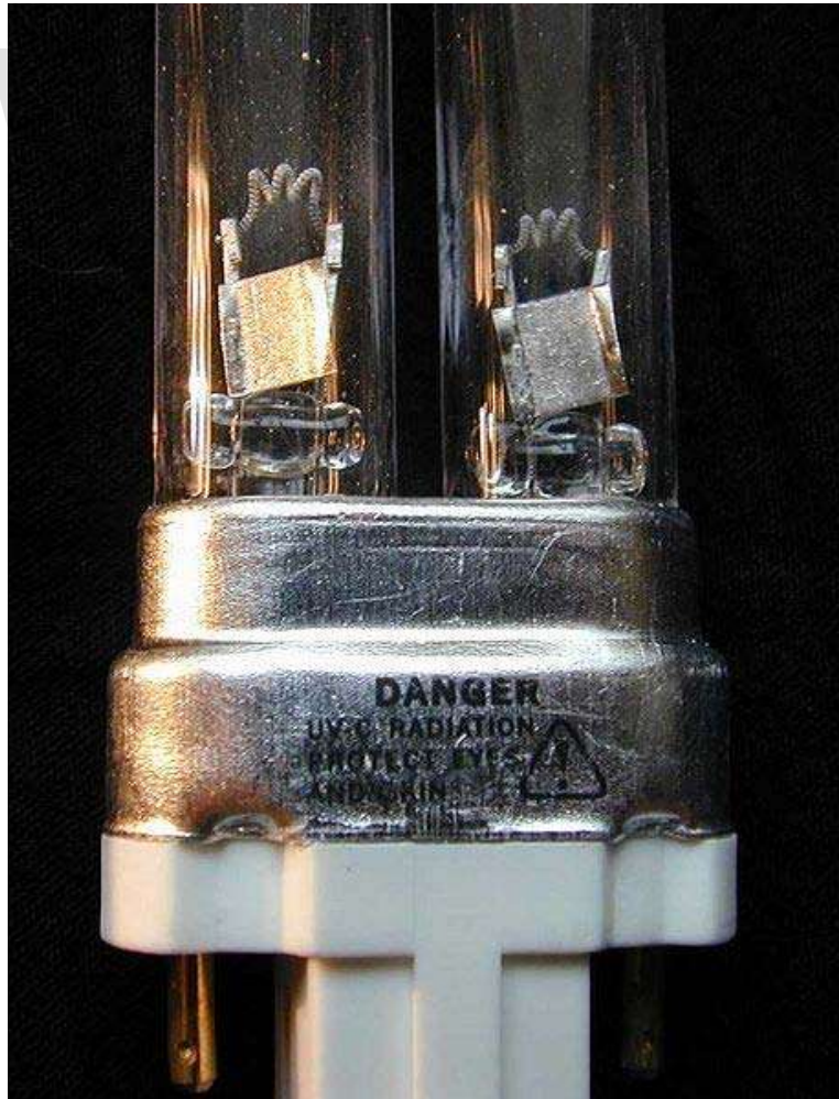
Close-up of the cathodes of a germicidal lamp (an essentially similar design that uses no fluorescent phosphor, allowing the electrodes to be seen.)
