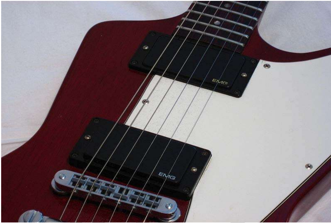
EMG 81 and EMG 85 — pair of popular active pickups
