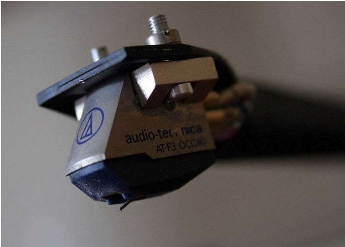
An Audio Technica AT-F3 MC cartridge
