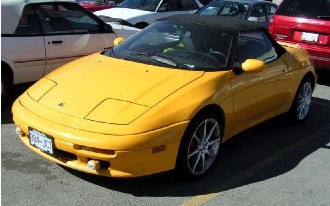
1990s Lotus Elan M100, a front-engine, front wheel (FF) drive sports car
