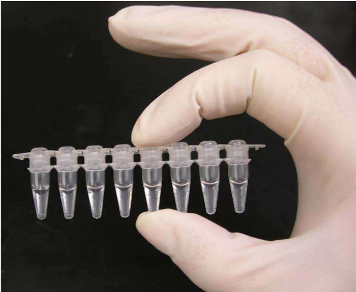
A strip of eight PCR tubes, each containing a 100 µl reaction mixture
