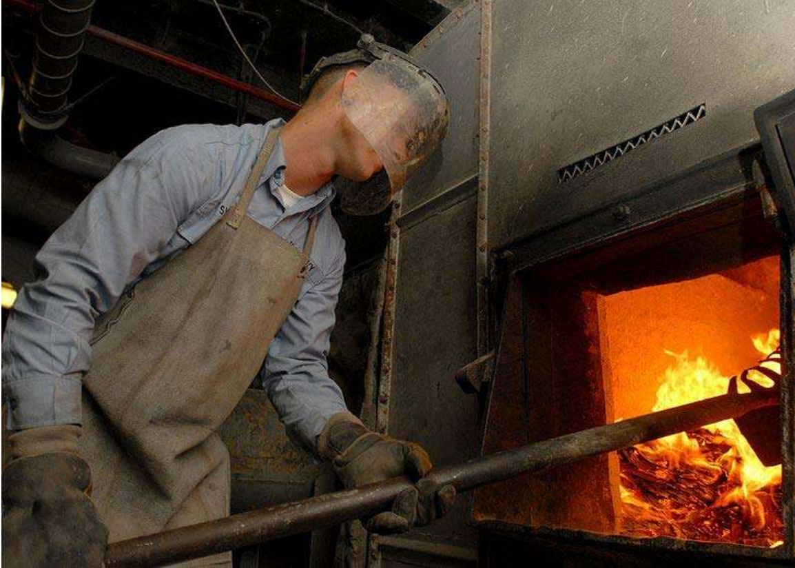
Operation of an incinerator aboard an aircraft carrier
